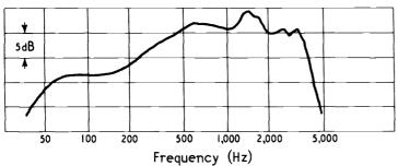
Fig. 9. Axial frequency characteristic of Bextrene cone fitted with p.v.c. surround of the type shown in Fig. 7.
