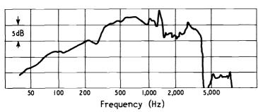
Fig. 6. Axial frequency characteristic of Bextrene cone from second mould, fitted with p.v.c. surround of shape shown in Fig. 4.
