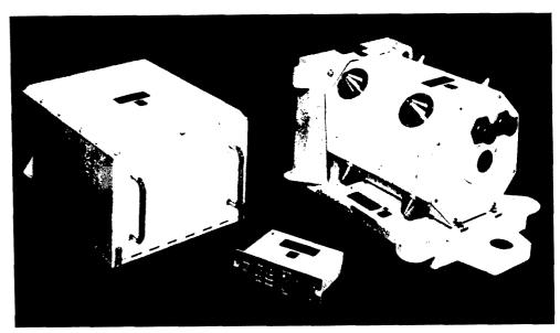
Inertial platform, control panel and associated equipment supplied by Ferranti for the prototype.
