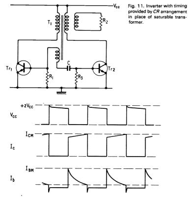
Fig. 12. Voltage and current waveforms in the inverter with CR timing.
