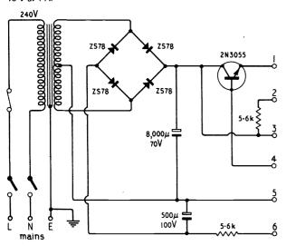
The circuit diagram of the module given in Fig. 2 shows a number of different supply rails which may be related to Fig. 1 as detailed below:
