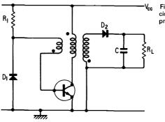
Fig. 7. Simple d.c. converter circuit using ringing choke principle.
