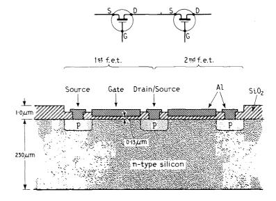
Fig. 1. Basic structure of a field-effect device in an m.o.s. integrated circuit (not to scale), showing how two of the devices can be easily connected in series by making one p-type region common to both.
