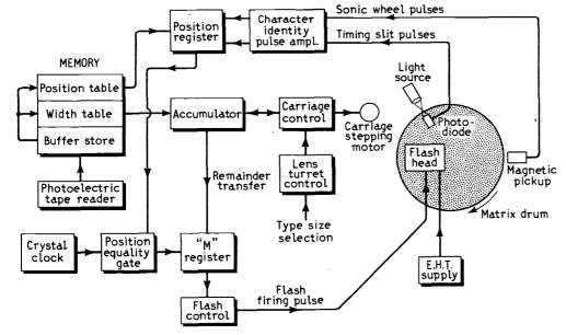
itself the widths of all the characters on its matrix drum. It does this in part of the magnetic core memory in its control unit. Into another part of this memory each line of data is loaded as it is read from the tape. While the line is being read, a justification process similar in principle to that performed in the 540 control unit is carried out.
