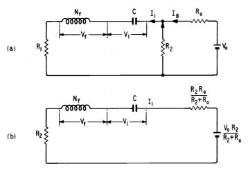
Fig. 82. The transformer can either be of a non-saturable type, or of a saturable type. In the case of the non-saturable transformer circuit, a considerable variation of frequency with load will be experienced and the transformer size required to handle the same power will be three to four times as big as one using a saturable transformer. The circuit with single non-saturable transformer is therefore regarded as not suitable for practical purposes.
