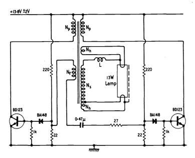
Fig. 14. Circuit of 13-watt fluorescent lamp inverter.
