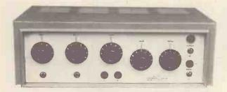
**CP50 AMPLIFIER.** An all silicon transistor 50 watt amplifier for mains and 12 volt battery operation, charging its own battery and automatically going to battery if mains fail. Protected inputs, and overload and short circuit protected outputs for  $8\Omega-15\Omega$  and 100 volt line. Bass and treble controls fitted.
