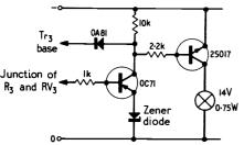
Mr. Hubbard's overload protection circuit
