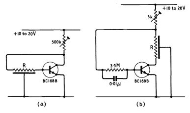
Fig. 6 Phase shift oscillators: (a) low-frequency, for R up to 5 M $\Omega$ : (b) high-frequency, for R down to 1 k $\Omega$ .
