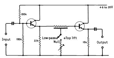
Fig. 5. Practical circuit giving low-pass, notch, and top-lift responses. Any good high-gain low level planar transistors (2N3707, BC109, BC168B, etc.) may be used.
