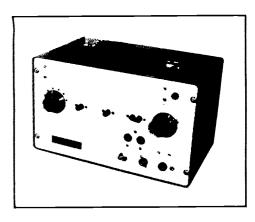
specified by the B.B.C. except that there are no equalizing pulses before and after the field pulse sync. group. The TPG55 measures 12 x 7.75 x 8.5 inches; weight with battery is under 9lb; and the price is £88 10s. The power supply needed for mains operations is extra costing £4 5s. Rank Bush Murphy Ltd, Welwyn Garden City, Herts.
