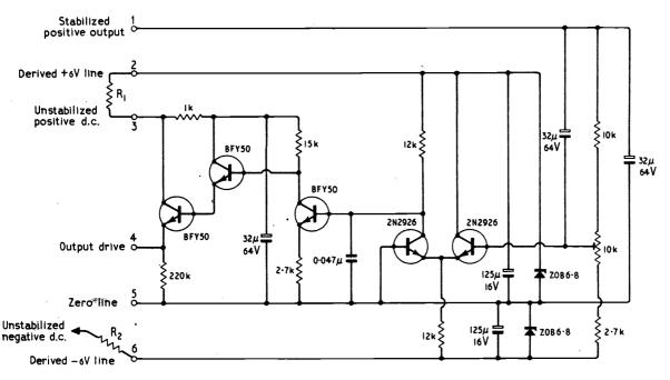
Fig. 2. Details of the stabilization module circuit including the two external resistors. All resistors are Erie EMI 5%; electrolytic capacitors, Mullard C426 series: potentiometer, Painton Miniflatpot; and the 0.047  $\mu$ F capacitor. Mullard C280Ae. The output from the module is taken from terminal No. 1 (positive) and terminal No. 5 (negative).
