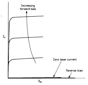
Fig. 2. Collector current vs. collector voltage characteristic of a transistor.
