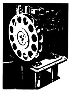
High density precision tape recording head used in the *Concorde* prototype accident recording system being produced by Elliott Automation. The system records 300 parameters and is protected for crash loads and is automatically ejected if submerged.
