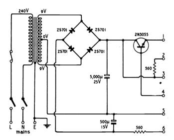
Fig. 1. A typical power supply for use with the stabilization module.
