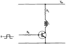
Fig. 4. Basic arrangement of transistor working into inductive load, as found in inverter circuit.
