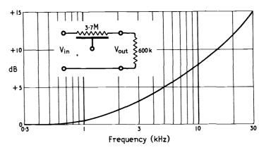
Fig. 4. Top-lift connection. When the "earth" is left off the response rises with frequency. The I.f. insertion loss depends on the resistance values.
