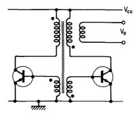
Vcc Fig. 8. Conventional single-transfor mer d.c. inverter circuit.
