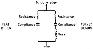
Fig. 8. Mechanical circuit diagram of surround.
