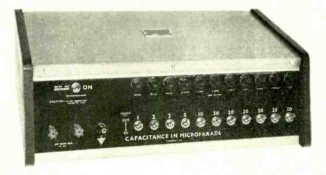
Compact 140  $\mu$ f paper capacitor box designed for stacking in units of up to six. Tolerance  $\pm$  5%. Rated at 300V. AC or DC. Each capacitor individually fused.
