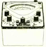
$\begin{array}{c} \textbf{MULTIMETER CT471A Battery-operated, fully-transistorised, sensitivity 100M\Omega/V, measures s.c./d.c. voltage (12mV-1200V scales, <math>\pm 3\%/\pm 2\%$  f.s.d.), s.c./d.c. current (12µA-1.2A scales,  $\pm 3\%/\pm 2\%$  f.s.d.), resistance (12,120M\Omega scales,  $\pm 3\%/\pm 2\%$  f.s.d.), h.f./v.h.f./u.h.f. voltage with multiplier (4V-400V scales up to 500MHz; 40mV-4V up to 1000MHz).
