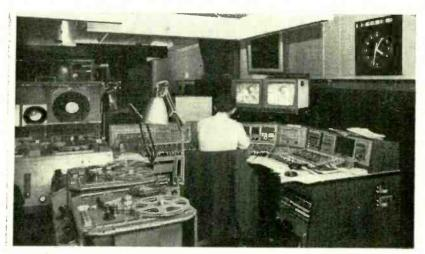
Sound controller's position with tape and disc backing facilities, in the sound control room associated with one of the two colour studios.
