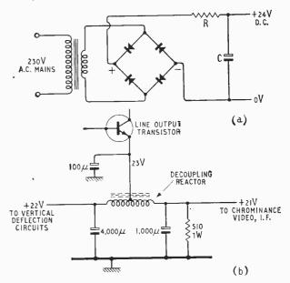
Fig. 6. Obtaining low-voltage, 24-V d.c. supply for transistor circuits in hybrid (transistor-cum-valve) colour receiver: (a) by mains stepdown transformer, and (b) by decoupling reactor in line output transistor emitter (RCA circuit).
