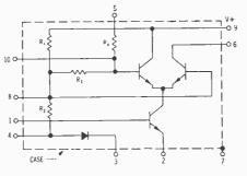
For this kind of operation pins 4, 8 and 10 should be by-passed to earth, the input signal applied to pin 1 (<100<sup>!2</sup> source resistance), a.g.c. input applied to pin 5, the output taken from pin 6 and pins 2, 3, 7 and 9 earthed.
