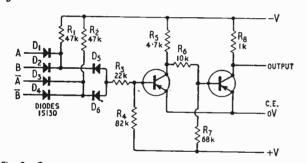
Fig. 9. Comparator circuit. (Cost per comparator: 8 resistors at 2d each, 6 diodes at  $4\frac{1}{2}d$  each, 2 transistors at 9d each = 5s 1d)
