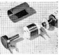
including contact bounce, and release time is of the order of  $500 \,\mu$ s. Mating surfaces are gold coated, and typical contact resistance is  $30 \,\mathrm{m}\Omega$ . Operating life when switched 60 V d.c. at half an amp (resistive) is said to be at least one million operations, rising to five million at 60V 100 mA. The 1 M can be produced in multiple forms. Overall dimensions are less than 1.5 cu. cm. STC Electro-Mechanical Division, West Road, Harlow, Essex.
