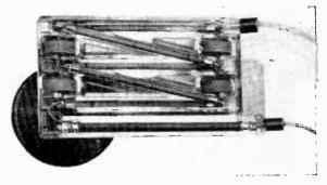
The e.h.t. Cockcroft-Walton voltage tripler is a separate sealed unit which is attached directly to the c.r.t final anode by a clip connector (in the centre of a black circular insulating cover which can be seen underneach)
