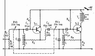
Fig. 3. Complete Q multiplier circuit. All resistors are  $\frac{1}{10}W \pm 10\%$  unless stated otherwise. Transistors are OC7's or similar I.f. types.
