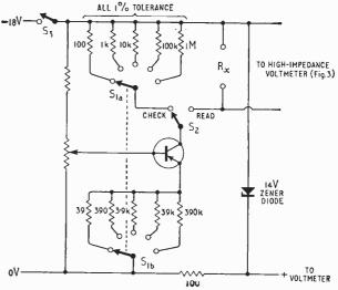
resistors on a low range can be used for this) and the input and output voltages of the amplifier adjusted with the  $5 \text{ k}\Omega$  potentiometer to be the same. If on setting this at one reading the readings at the other end of the scale are incorrect the resistor R should be altered to compensate for this. Once this has been done the readings over the 1-10 V range should be accurate.
