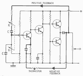
Fig. 2. Basic circuit of oscillator showing feedback loops.
