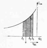
Fig. 3.  $C_{te}$  as a function of  $V_{\rm DE}$ . When base-emitter junction is forward biased infinite capacitance point is never reached since  $l_{\rm E}$  increases rapidly with  $V_{BE}$ .
