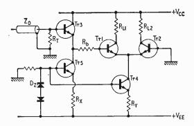
Fig. 6. Current switch for positive input pulses.
