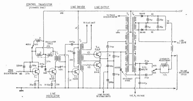
Fig. 1. Part of circuit of line timebase (not including all oscilliator control circuitry and all 625/405 switching)
