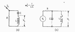
Fig. 1 Basic filter circuits. Variable selectivity can be obtained by cascading several.
