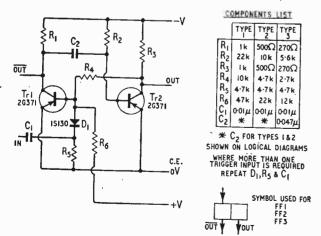
Fig. 10. Flip-flop (monostable) circuit and symbol (Cost per flip-flop: 6 resistors at 2d each, 2 capacitors at 4d each, 2 transistors at 9d each, 1 diode at  $4\frac{1}{2}d = 3s$  6d)
