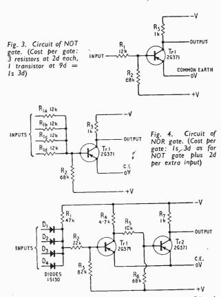
Fig. 5. Circuit of AND gate. (Cost per gate: 7 resistors at 2d each, 4 diodes at  $4\frac{1}{2}$ d each, 2 transistors at 9d each = 4s 2d)
