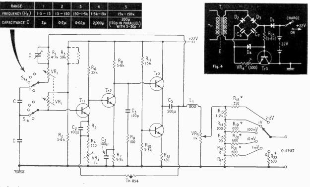
Fig. 3. Complete oscillator circuit with power supply circuit inset (Fig. 4). Note that Ni-Cd battery can be trickle charged by leaving connected to power supply when oscillator is switched off.  $R_5$  should be 4'3k $\Omega$ .
