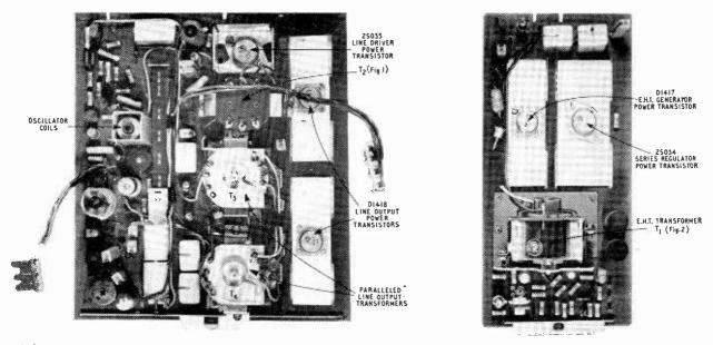
Left: Layout of line timebase unit on replaceable printed-circuit module. Right: The e.h.t. unit on its replaceable printed-circuit module.
