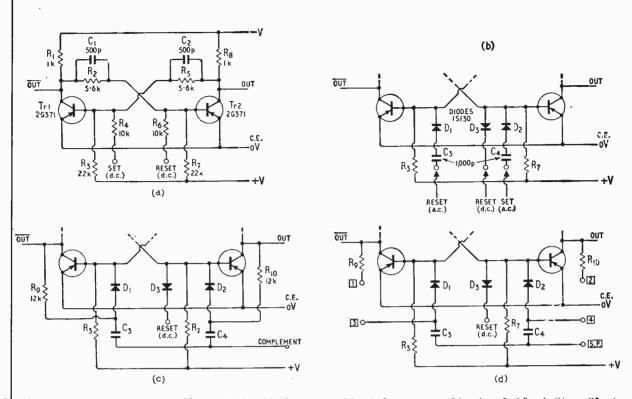
Fig. 11. (a) Set/reset d.c. bistable circuit (Cost per d.c. bistable: 8 resistors at 2d each, 2 transistors at 9d each = 3s 6d). At (b), modifications to (a) to produce set/reset a.c. bistable. (Cost per a.c. bistable = 4s  $11\frac{1}{2}d$ ). At (c), modifications to (a) to produce counter bistable. (Cost per counter bistable: 5s  $3\frac{1}{2}d$ ). At (d), modifications to (a) to produce set/reset bistable. (Cost per counter bistable).
