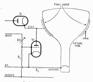
Fig. 2. Basic e.h.t. regulation circuit
