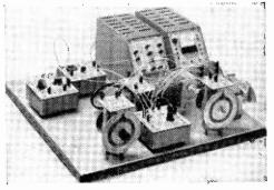
d.c. error channel for synchro elements and a demodulator, giving an a.c. (50 c/s carrier) error channel. With certain auxiliary apparatus, frequency and transient response studies can be carried out. The price is  $\pounds 275$ .
