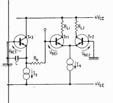
Fig. 5. Current switch biasing in which Tr1, Tr2 and Tr3 are on the same silicon slice.
