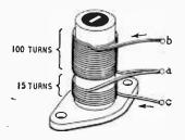
Fig. 3. Details of L<sub>1</sub>. Winding consists of 115 turns 38 s.w.g. enamelled wire scramble wound on a  $\frac{1}{4}$  in dia. former, with core, and tapped at 15 turns.
