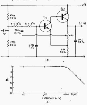
Fig. 14. (a) Active filter to give attenuation of frequencies liable to beat with tape recorder bias frequency (Trl: BC108, 2N929, 2N3707 or 2N2926; Tr2: 2N3703, OC201, NKT2044). (b) Response of filter.
