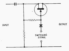
Fig. 8. Series gate using field-effect transistor.
