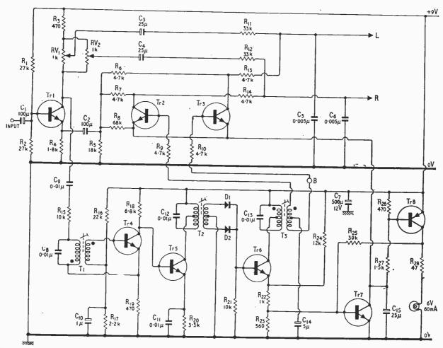
Fig. 9. Stereo decoder circuit (negative earth version). In the positive earth version, polarity of electrolytic capacitors is reversed, resistors  $R_1$ ,  $R_{16}$  and  $R_{18}$  altered in value and p-n-p transistors used (apart from Tr8).
