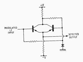
Fig. 7. Possible arrangement for an integrated-circuit detector.
