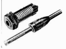
A QUICK and secure method of connecting miniature cables with up to 12 cores is said to be provided by the Rendar multipole jack plug and socket. In addition to its form as a connector, it can also be supplied with a large number of combinations of make and/or break contacts on the socket. Electrical contact is made by a slight clockwise turn of the plug after insertion, the plug remaining locked in this position. Rendar Instruments Ltd.
