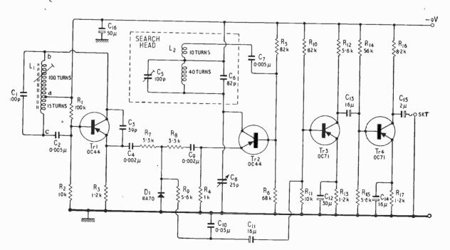
Fig. 2. Metal locator circuit. All resistors are 10% tolerance, ½ W.
