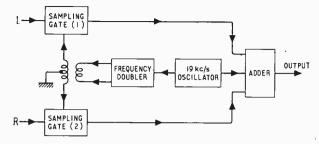
Fig. 3. Sampling method of stereo signal encoding.
