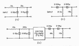
Fig. 4. Filter circuits: (a) 100 c/s, (b) 1 kc/s, and (c) 10 kc/s.
