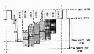
Fig. 6. Diagram showing colour-bar test waveform (for full amplitude 95% saturated primary and complementary colours). Heavy contour shows how signal would be reproduced ideally on a monochrome receiver in bands of progressively darker shades of grey from white to black.
