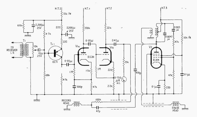
Fig. 3. (Above) Amplifier circuit for sound recording, with (right) the power supply and control unit.
