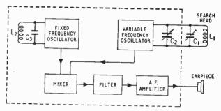
Fig. 1. Block diagram of metal location system.
