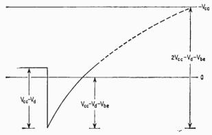
Fig. 2. Base waveform of Tr2 during "off" period.
