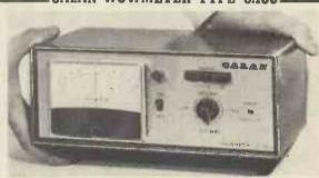
This new instrument will be of immediate interest to all con-cerned with the performance of magnetic tape transport systems. Here for the first time is an instrument suitably priced for use in the domestic tape recorder service workshop and the production line. Accurate measurements can be taken of capstan slip and the performance of the back tension system may be easily assessed. The unit is provided complete with 3Kc/s test tapes recorded at any two of the standard tape speeds.
