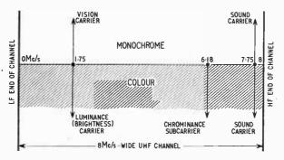
Fig. 1. Location of information carrier frequencies within u.h.f. channel used for both monochrome and colour transmission. This illustrates how black-and-white and sound information carrier frequencies are the same in both transmissions, while colour information in the colour transmission is on a separate subcarrier not present in the black-and-white transmission.
