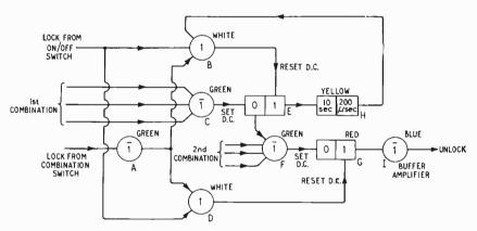
Fig. 7. Logic arrangement for lock with time-limit facility.
