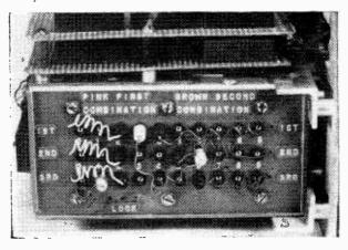
B/2. In the external alarm a key-operated switch is used that could be arranged to disconnect the alarm unit's batteries.
