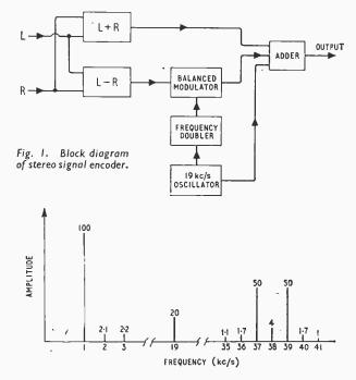
Fig. 2. Frequency spectrum at output of stereo encoder with slightly distorted I kc/s signal in one channel.
