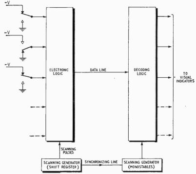
Fig. 9. Principle of time-division multiplexing.
