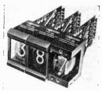
minal type selected. A choice of turret lug terminals or edge connectors is offered. This TNR-50 series may be custom designed to meet special electrical functions such as coded input to octal readout, counters and memories. Litton Precision Products, 503, Uxbridge Road, Hayes, Middlesex.
