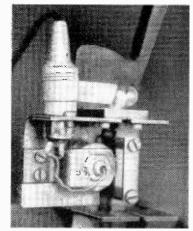
Left: The erase head mounted on the projector.
