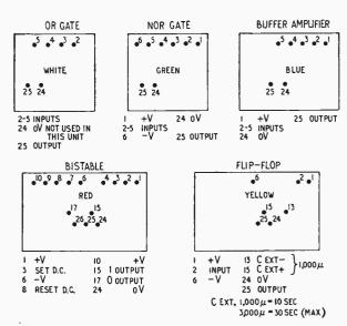
Fig. 11. Connections on the logic modules.
