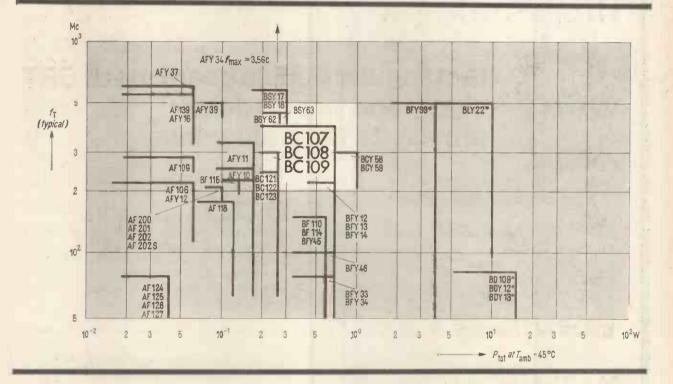
BC 107 For general purpose high gain preamplifier and driver stages, d.c. amplifier and switching applications.
