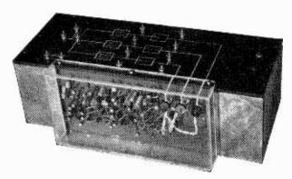
Fig. 8. Completed demodulator.
