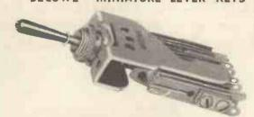
Designed for use in compact modern equipment for all climates, these stainless-steel Keys are only 0.425" wide by 0.78" long and 1.76" deep behind panel.
