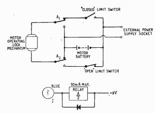
Fig. 4. Battery circuit for bolt actuation.
