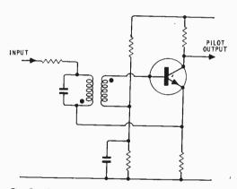
Fig. 5. Q multiplier method of pilot tone extraction.
