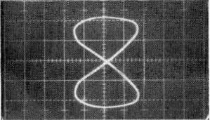
Fig. 11. Fattern obtained when phase relationship between 39 kc/s waveform at B (Fig. 9.) and 19 kc/s input is correct.
