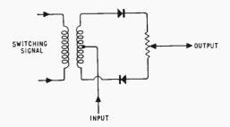
Fig. 6. Balanced diode series gate.
