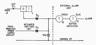
Fig. 9. Arrangement for an external alarm.
