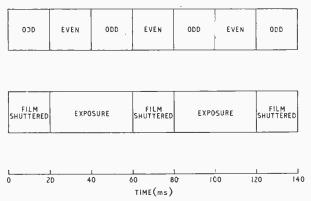
Fig. 1. Cycle of exposure of film to television fields, to give  $16\frac{2}{3}$  film frames (complete television pictures) per second.
