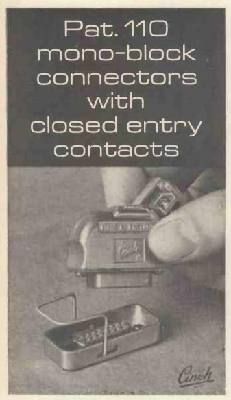
Designed to comply with D.E.F 5325 PAT. 110, these connectors consist of one-piece Diallyl Phthalate moulding with hard gold plated plug pins, socket contacts, and beryllium copper contact clips. Closed entry contact design eliminates the risk of damage to the sockets by test probes. The shells are of passivated cadmium plated steel and the covers and cable clamps are of die-cast aluminium Grade LM6.
