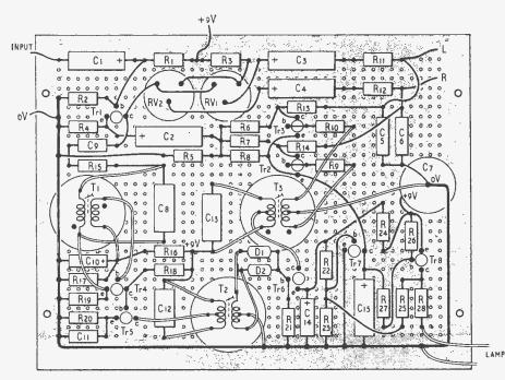
Fig. 10. Diagram to show suggested layout and wiring. The components and wires shown unfilled are on the top side of the board (Lektrokit) and the wires shown solid on the other side, as made clear below  $\Psi$ .
