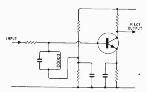
Fig. 4. Simple method of pilot tone extraction.
