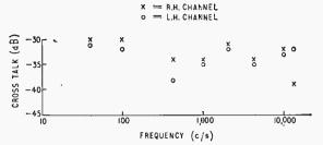
Fig. 13. Channel separation (experimental results).
