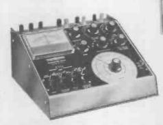
Heathkit Model IM-30U transistor tester from Daystrom Ltd.
