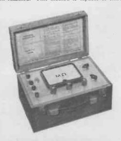
Fig. 35. Typical commercial high-resistance megohmmeter (W. G. Pye 11801 Wide Range Megohmmeter, 3M $\Omega$  to 200 million M $\Omega$ ).
