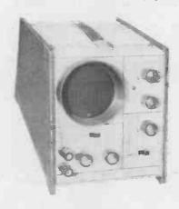
Telequipment oscilloscope designed for teaching "O"-level physics.
