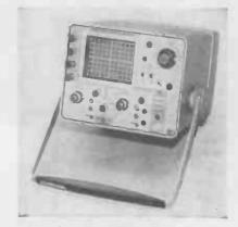
Tektronix Type 422 portable oscilloscope
