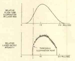
Fig. 8. Spiky output is due to momentary rapid depopulation and repopulation of metastable level.
