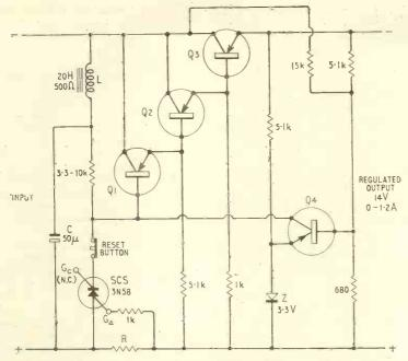
Fig. 5. Overload trip using silicon controlled switch.
