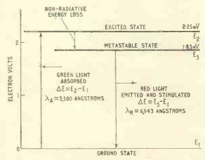
Fig. 6. Energy level diagram for the ruby laser.
