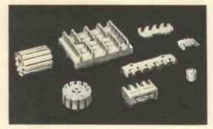
Refractories for high-temperature insulation.
