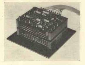
Sealectro programming board with circuit deck.
