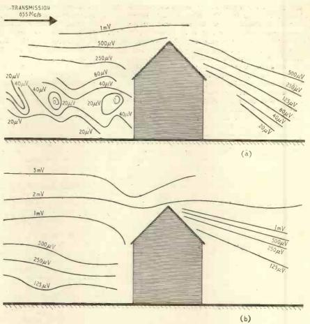
Fig. 2. Terminal voltages from aerial plots adjacent to a suburban two-storey house; (a) using a  $\lambda/2$  dipole and (b) using a Yagi with a 12 dB forward gain relative to a dipole.
