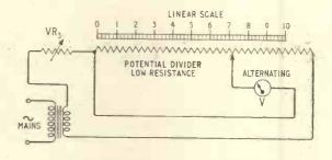
Fig. 2. Calibration of scale divisions.
