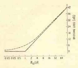
Fig. 3. Bridging loss produced by resistance R across a line, with generator and load impedances Ro.
