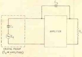
Fig. 5. Equalization for crystal pickup.
