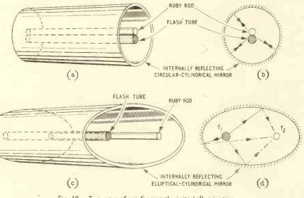
Fig. 10. Two ways of reinforcing the initial illumination.
