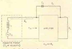
Fig. 3. Equalization for magnetic pickup.
