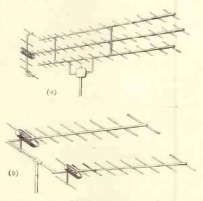
Fig. 5. Techniques for increasing u.h.f. aerial gain and directivity; (a) using director side rows and (b) broadside coupling.
