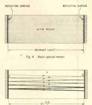
Fig. 5. Fabry-Perot resonator. Rays are successively reflected from end to end of the cavity A, reinforcing each other and producing a strong parallel beam. (Rays are shown slightly non-parallel for clarity.)
