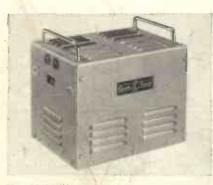
Claude Lyons Series TS are the most advanced electro-mechanicai a.c. automatic voltage stabilisers available anywhere today – providing high-speed, accurate stabilisation of voltage without distortion of waveform. Speed of correction is up to 60 volts/sec with an accuracy of  $\pm$  0.25% from zero to full load. Ouput voltage is unaffected by variations in supply frequency, load current or load power factor. Indoor tropical rating is standard on all models.
