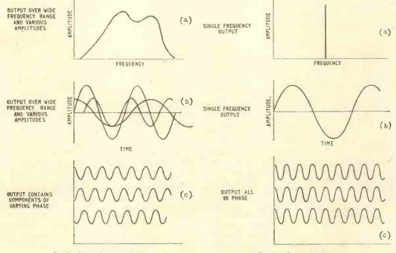
Fig. I. Non-coherent radiation.
