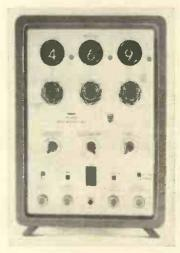
Philips trigger delay unit, Type GM4585.
