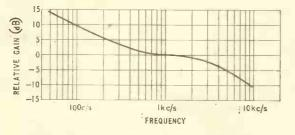
Fig. 2. Equalization required for magnetic pickups.
