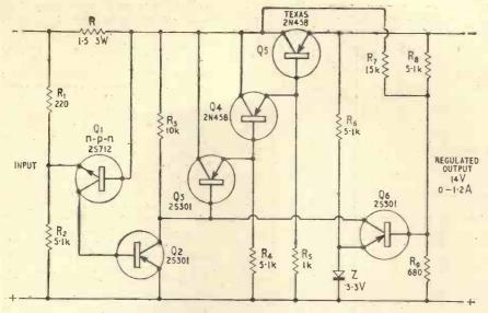
Fig. 3. Transistor regulator with current-limited output.
