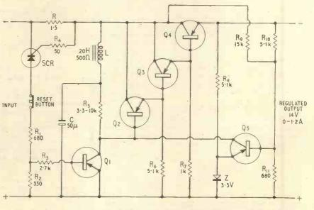
Fig. 4. Overload trip action is provided by this circuit, using a silicon controlled rectifier.
