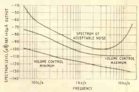
Fig. 9. Noise spectrum of pre-amplifier (magnetic pickup position).
