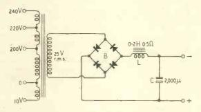
Fig. 2. Power supply unit with choke-input filter.
