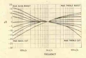
Fig. 7. Pre-amplifier tone control characteristics.
