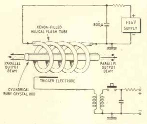
Fig. 9. Ruby crystal laser with helical flash-tube pump.
