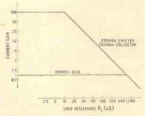
Fig. 6. Asymptotic behaviour of current gain of a transistor as a unction of load resistance.
