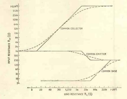
Fig. 4. Input resistance of a transistor as a function of load resistance in the three modes of operation.
