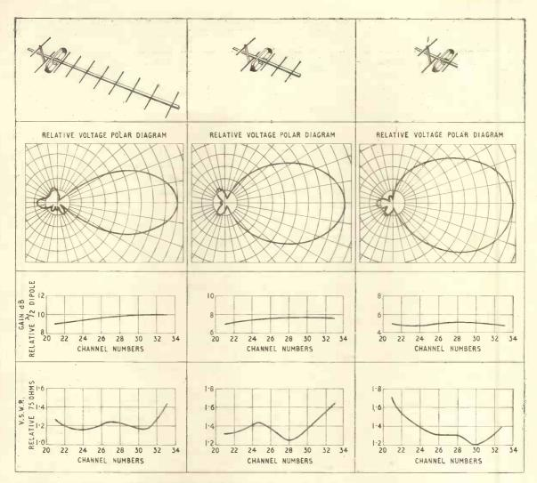
Fig. 4. Typical performance figures for wide-band u.h.f. aerials,
