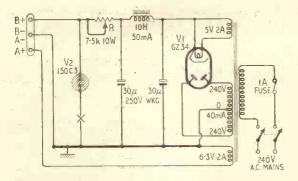
Fig. 1. Voltage-regulated power supply suitable for use with BC-221 frequency meter. R is adjusted to give 15 mA in a milliammeter inserted at X.
