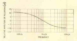
Fig. 4. Standard recording characteristic (amplitude versus frequency).
