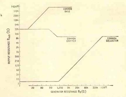
Fig. 5. Asymptotic behaviour of output resistance of a transistor as a function of source resistance.
