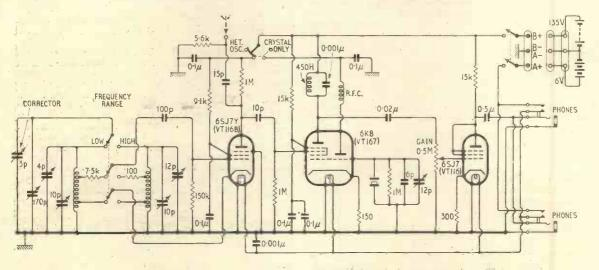
Fig. 4. Circuit diagram and components list of BC-221-O. This is typical of most models.
