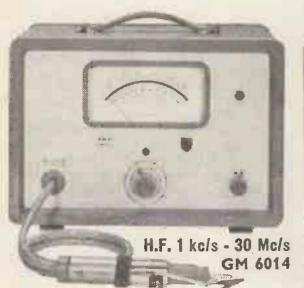
Range (fsd) 1 mV - 300 V -80 dB to + 32 dB Input impedance without attenuator 1 M $\Omega$  - 50 k $\Omega$ //7 pF with attenuator 50 M $\Omega$  - 2 M $\Omega$ //2 pF Accuracy 3% Calibration voltages 30 mV and 3 V
