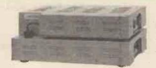
LOW DISTORTION POWER AMPLIFIER Specification: Power Output: 10W, 20W, 50W, or above with a choice of 3, 5 or 15 ohm load. Input for Specification Output: 250 mV Total Harmonic Distortion: 0.1% at full output Frequency Response: 20 c/s-20 kc/s ± 1 dB Signal/Noise-Ratio: Better than 80 dB Damping Factor: More than 50 Supply: A.C. Mains 240/120 V, 50-60 c/s or battery with built-in D.C. converter—12/24 V Size: 11 × 4 × 7± inches
