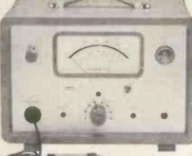
U.H.F. 0.1 Mc/s - 800 Mc/s GM 6025 Range (fsd) 10 mV - 10 V -60 dB to + 22 dB Input impedance at 200 Mc/s  $35 k\Omega //1 pF$ Accuracy 5% Calibration voltages for each range Probe-diode quickly exchangeable T-piece for measurements on 50  $\Omega$ coaxial lines available
