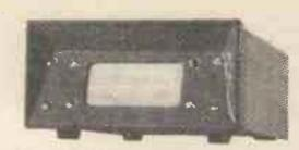
AUTOMATIC GAIN-CONTROLLED MICROPHONE Specification: Input: Built-in microphone Output Signal: 15 mV Output Impedance: Less than 100 ohms Frequency Response: 250 c/s-3,500 c/s A.G.C. Range: More than 60 dB Supply: A long service battery is supplied with a life of approx. 50 hours Size: 4½ x 2¼ x 6% inches
