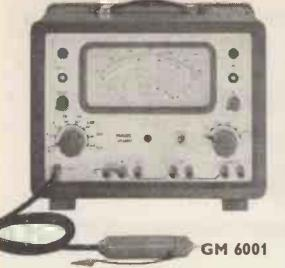
DC Range (fsd) 300 mV - 1000 V with EHT probe up to 30 kV Input impedance  $10\Omega - 100 M\Omega$ Accuracy 2.5% AC 20 c/s - 1000 Mc/s Range (fsd) 1 V - 300 V Input capacitance 3.5 pF Accuracy 3% Resistances Range  $1.\Omega$  -1000 M $\Omega$  (centre scale values  $10\Omega - 100 M\Omega$ )
