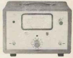
L.F. 2 c/s - 1 Mc/s GM 6012 Range (fsd) 1 mV - 300 V -80 dB to + 52 dBInput impedance (1 mV - 3 V) 4 MΩ //20 pF (10V-300V) 10 MΩ //10 pF Accuracy (5 c/s - 100 kc/s) 2.5% (2 c/s - 1 Mc/s) 5 % Calibration voltage 30 mV and 10 V Amplifier output 50 x
