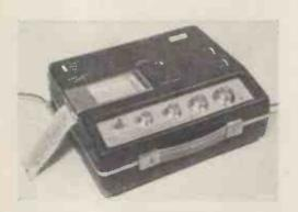
Devices R.I. recorder, with hot stylus unit in use, quickly be interchanged with an ink pen system.
