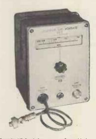
Grundig VS-2 u.h.f. converter for wobbulators.
