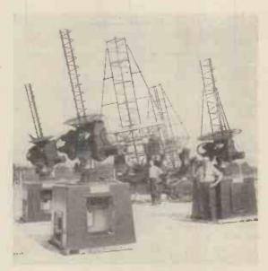
FRAME-GRID AERIALS?—These five helical aerials have been designed by Cossor Radar & Electronics and are for use by the War Office at the Guided Weapons Trials Establishment on the coast of Anglesey. They will operate in the frequency range 100—400Mc/s employing circular polarization and will be for telemetering missiles.
