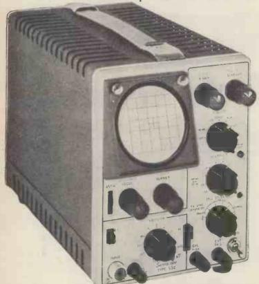
The introduction of the first Serviscope S31 set a new standard in small portable oscilloscopes. Now with the model S32 replacing the S31, the Serviscope again reaches far out beyond all competition. This successor to the S31 retains all the features of the earlier model including the same compact dimensions, calibrated attenuator and time base and unique triggering facilities, but has five immense improvements:
