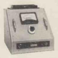
Shaw "Varsity" moisture meter. Material sample is placed in 2,000cm³ container on top of the instrument.
