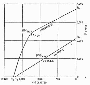
Fig. 1. Demagnetization curves for barium ferrite.
