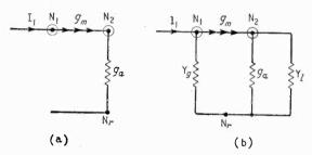
Fig. 5. Equivalent nodal circuits of a valve amplifier (a) in the ideal form of Fig. 3 and (b) with the addition of a grid admittance  $Y_g$  and load admittance  $Y_L$
