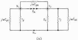
Fig. 6. Valve with interelectrode capacities (a) and its nodal equivalent circuit (b).
