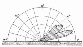
Fig. 11. Vertical radiation pattern of a scale model 2-element "Quad" aerial.
