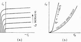
Fig. 11. Common-base characteristics of the transistor (a) at its output and (b) at its input.
