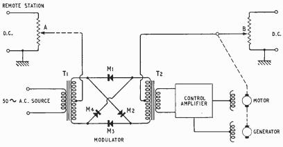
Fig. 1. Servo system schematic used for the remote control of a television camera.
