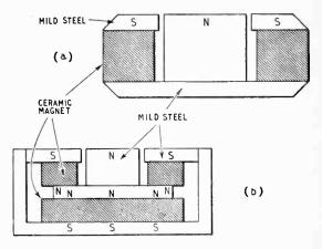
Fig. 4. (a) Ring type loudspeaker assembly (b) Pot type assembly.
