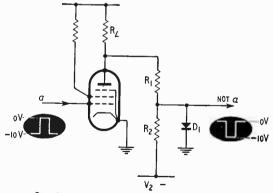
Fig. 6 Voltage inverter circuit of a NOT gate.
