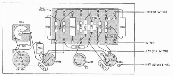
Fig. 2. Layout of components and wiring on the underside of the "top" plate of the chassis box.
