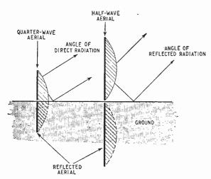
Fig. 1. Direct and reflected radiation from aerials adjacent to earth.
