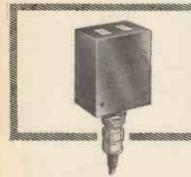
The Proximity Switch will provide a signal to operate a Basic Logic Unit. whenever a mass of ferrous material comes within 5mm of the operating face. Having no moving parts, it is an encapsulated wound commonent suitable for use in conditions of vibration, shock, dust, damp-in fact, in any environment where the epoxy potting compound and the cable gland will not be damaged.
