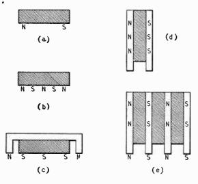
Fig. 5. Holding assemblies using ceramic magnets.
