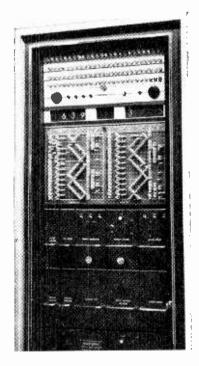
Beckman Instruments "123" datalogging system. "Peg board" is used for setting up.
