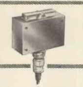
The Contactless Changeover Switch, a form of differential transformer, will provide signals to operate Basic Logic Units, changing over when the armature is rocked by about 1.5 degrees i.e. 1mm movement at one end. Apart from the solid steel armature which pivots on a stainless steel pin in a bronze bush, there are no moving parts; the body of the device being similar to that of the proximity switch.
