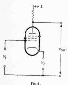
impedance levels between network and source. Reasonable accuracy can be obtained by using multi-grid valves as shown in the subtraction circuit of Fig. 4.
