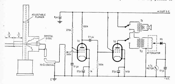
Fig. 6. Receiver and field-strength meter used for aerial measurements at 3,000Mc/s. VI = EF91, V2 = EL91; T1 = loud-speaker transformer; T2 = 1 to 1 ratio a.f. transformer; M1 meter rectifier or diode.
