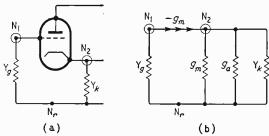
Fig. 8. Typical cathode-follower (a) and its nodal equivalent circuit (b).
