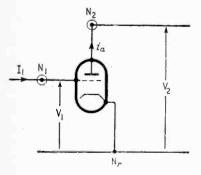
Fig. 3. Basic ideal valve amplifier.
