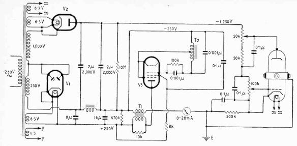
Fig. 5. Klystron oscillator, power supply and modulator used by the author. VI = 250V rectifier; V2 = 1,250V rectifier; V3 = EF91; Klystron (see text); T1 = modulation transformer, ratio 1 to 1; T2 = tapped a.f. transformer.
