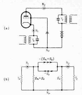
Fig. 10. Simple grounded-grid amplifier (a) and its nodal equivalent circuit (b).
