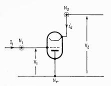
Fig. 7. Basic ideal grounded-anode valve (cathode follower).
