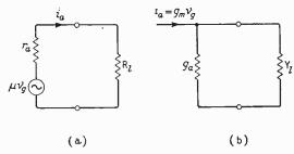
Fig. 2. Voltage (a) and current (b) generator equivalent circuits of the valve amplifier.
