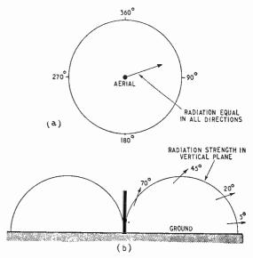
Fig. 2. Radiation field from vertical aerial; (a) in horizontal plane, (b) in vertical plane.
