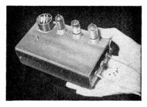
The completed crystal marker showing the top plate screwed to the chassis box.
