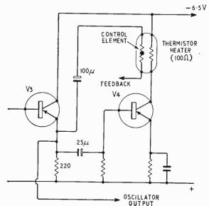
Fig. 1. Use of separate power amplifier for thermistor
