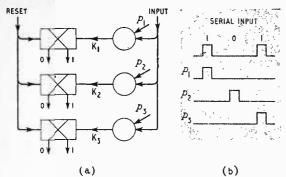
Fig. 10 (a) Staticisor (store) for serial input train of three binary pulses. (b) Serial input train and clock pulses for storing 101 in the staticisor of Fig. 10 (a).
