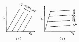
Fig. 1. Idealized triode (a) and pentode (b) characteristics.
