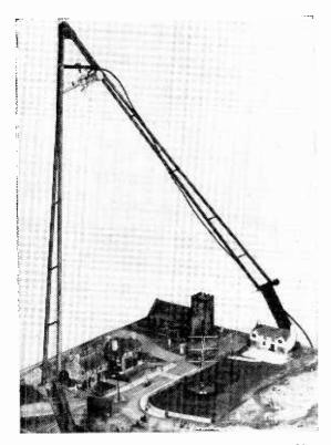
The 3,000-Mc/s model aerial testing table (scale 4mm/ft) used by the author. The aerial shown in lower centre is a scaled-down 6-element, stacked array for a normal frequency of 30Mc/s.
