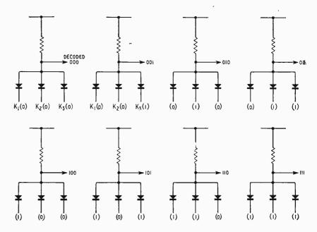
Fig. 11 Set of eight AND gate decoders for the eight possible states of three bi-stable elements.
