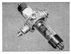
Fig. 4. Typical 3,000-Mc/s Klystron oscillator, the Type CV67.
