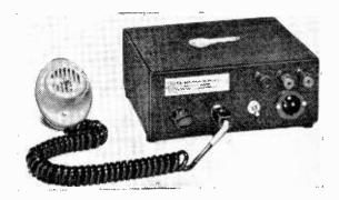
R.E.E. 20W transistor PA amplifier. The key gives a good indication of its size
