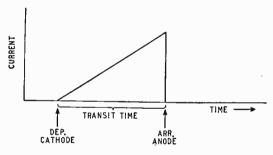
Fig. 2. Assuming a uniform field in Fig. 1, the charge is accelerated uniformly, and since the current in the circuit is proportional to the charge's velocity it increases steadily throughout the flight.
