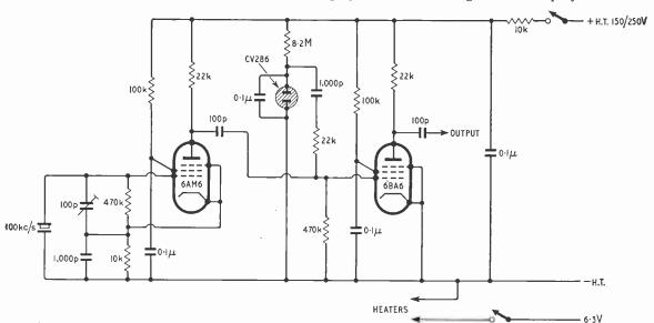
Fig. 1. Circuit diagram for the 100-kc/s crystal marker.
