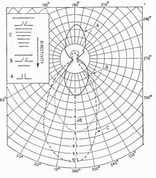
Fig. 9. Gains of 3- and 8-element Yagi aerials compared with a half-wave dipole measured at 3,000Mc/s.
