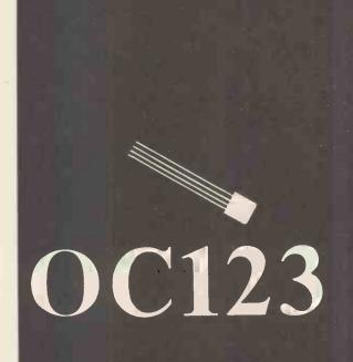
The OC123 is a ferrite core driver transistor similar to the OC23, but scaled down into a small metal can for those applications where space saving is of cardinal importance—such as in closely packed printed circuit boards—and where the dissipation rating need not be so high as with the OC23.
