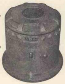
acceleration of 31 "G" peak can be obtained for an input current of 10 amps., which is equal to a thrust of 550 lbs. peak for an input power of 1 kW. The vibrator can also be supplied with a blower (V1000C.B.) and will deliver a thrust of 750 lbs. peak for an input power of 2 kW. Can be trunnion mounted if required.
