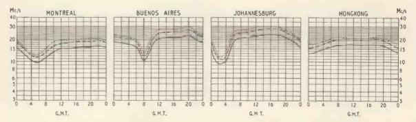
THE full-line curves indicate the highest frequencies likely to be usable at any time of the day or night for reliable communications over four long-distance paths from this country during July.
