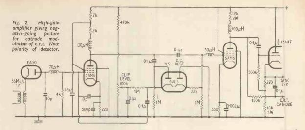
changes in polarity. The d.c. restorer becomes superfluous as the second v.f. stage grid will do the same job, by reducing the cathode bias. The purpose of the "safety circuit" round the cathode follower in Fig. 2 is to ensure that, in the event of a valve failure, the c.r.t. beam is cut off. For grid modulation of the tube this is achieved when the feed is taken directly from the cathode follower, so this safety circuit is not necessary. The modified circuit is shown in Fig. 3.
