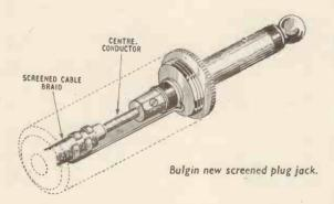
the screened sheath is gripped in a claw-like clamp, which serves also to take any strain on the cable.
