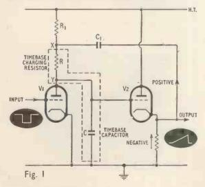
The potential levels during the quiescent period are maintained by  $C_1$  and  $R_1$ . Capacitor  $C_1$  does not discharge appreciably during the period of the sweep provided that:
