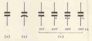
Fig. 2. How the familiar two-line capacitor symbol can be adapted to provide additional information: (a) standard; (b) indication of outer foil connection; (c) a representative voltage rating code as used on the Continent.
