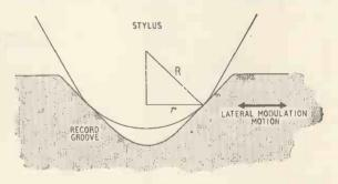
Fig. 1. "Effective stylus tip radius" (r) for lateral modulation.
