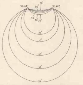
Fig. 3. Fixing-accuracy contours in feet for summer daylight operation. Contours are drawn for a 0.01 lane deviation.
