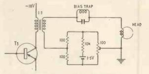
(see accompanying diagram) and to adjust this for minimum noise when playing a virgin tape. This is also the condition for minimum distortion.
