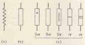
Fig. 1. The "common or garden" fixed resistor, (a) as cultivated in Britain, (b) the less elegant but equally distinctive Continental variety, (c) a Continental bunch, complete with wattage coding.
