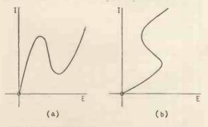
Fig. 6. Two types of current/voltage curve showing negative resistance.
