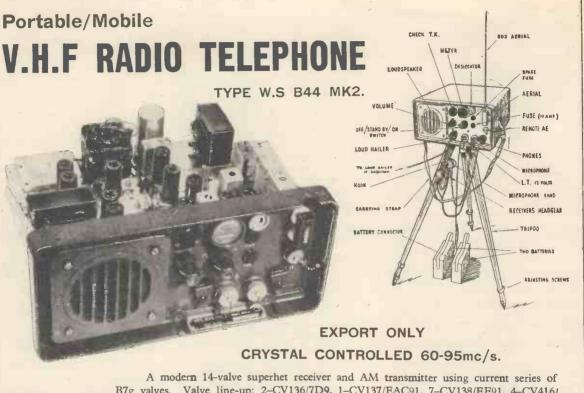
B7g valves. Valve line-up: 2-CV136/7D9, 1-CV137/EAC91, 7-CV138/EF91, 4-CV416/ 6F17. Robust cast aluminium case includes 5in. loudspeaker. Internal vibrator pack (synchronous type) provides operation from 12-volt accumulators or vehicle or boat 12-volt supply, in fixed or mobile use. Available, less crystals and accessories, but with connecting plugs, ex-stock. Accessories and crystals for specified frequencies in the range 60-95 Mc/s can be supplied to order at extra cost.
