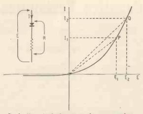
Fig. 2. Many circuit elements now in common use have resistances that do not follow the pattern of Fig. I. Though non-linear to d.c., they may be at least approximately linear to a.c. within limits, as for example P to Q here.
