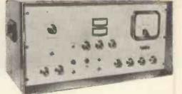
Microcell transistor test set.
