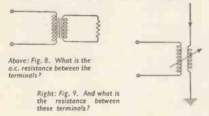
heat in the circuit element referred to. That is rother an important point, as we see if we consider Fig. 8. What is the "circuit element" to which the terminals are connected? The primary winding? The whole transformer? Or the transformer and its load regarded as one element?
