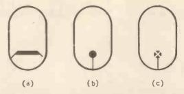
Fig. 6. Sketch (a) may seem a distinctive cathode, but (b) is quicker to draw, and in the form (c) provides additional information.
