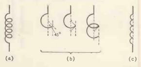
Fig. 3. Coils may look like (a), but to draw this symbol accurately is not simple—one way is shown in (b) which is not so quickly accomplished as the straightforward half-circles (c) now widely used on the Continent and in the United States
