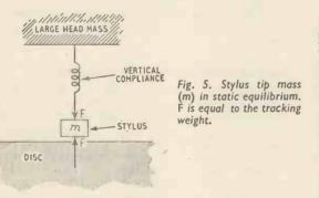
resonates with the effective tip mass. But this does not alter the main argument, nor that a greater compliance gives a greater tracking possibility at all frequencies below this resonance and that a lower tip mass gives better tracking above this resonance.
