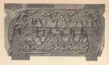
A complete range of transistorized counter panels of common size, fixing method and electrical connexion, designed to provide a flexible unit system whereby any special requirements in the counting or data processing fields can be quickly built up.
