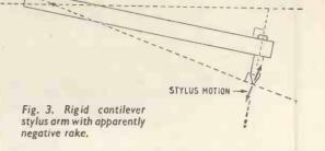
the rondel has been mounted with an apparently "negative rake" (as in Fig. 3). But surely the original purpose of "positive rake" as it was applied to the older type of needle (as in Fig. 4(a)) was to ensure that any forward drag at the stylus tip did not cause the stylus to dig further into the groove (as in Fig. 4(b)) with a cumulative effect upon this drag and its resultant digging.
