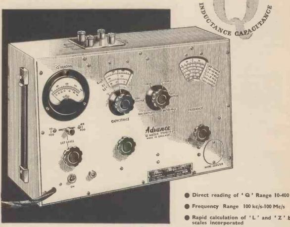
The 'Q' meters Models T1 and T2 provide a convenient method of making R.F. measurements of circuit magnification, inductance, capacitance and power factor at frequencies between 100 kc/s and 100 Mc/s. The two models are identical except that the Model T2 provides additional facilities for comparing 'Q,' inductance and cap-acitance, and is most suitable for the production testing of coils.
