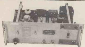
POWER UNITS TYPE 234: Primary 200/250 v. 50 cycles. Outputs of 250 v. 100 mA., and 6.3 v. 4 amps. Fitted double smoothing. For normal rack mounting (or bench use) having grey front panel size 19in. x 7in. BRAND NEW. ONLY 59/6 (carriage etc., 7/6):
