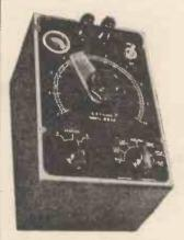
CR50 BRIDGE measures from 10pFd to 100mFd and from I ohm to 10 Megohms In fourteen ranges, having a total scale length of over 120 inches. Leakage test for condensers, Indication of balance is given by a magic eye fed from a high gain pentode. Internal standards of "Constants " 1% resistors. Robustly constructed for bench use, complete and ready for use from A.C. £8/2/6 plus 4/6 mains. carr./packing.
