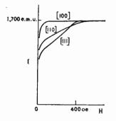
Fig. 8 Magnetization curves for the [100], [110] and [111] directions of a crystal of iron.
