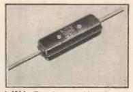
L.1314. For 2-core cables, 2 amp. 250 v. A.C./D.C. This new small flex lead filter is designed for the suppression of interference at band I television frequencies only, and is for insertion in the flex lead within 6in. of the motor of an appliance. This is the most conveni-ent form of filter which can be readily installed and is complete with terminals, cord grips, etc.
