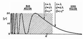
Fig. 2. With vertical polarization spacings d within the shaded area for the test aerials should be avoided.
