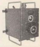
L.T. Transformer, input 230 v. Output 50 v., 50 ampere, but adjustable by voltage regulator switch on primary. In steel case fitted with mains switch, will take 100% overload. Grs. Wt. 150 lbs. Wound at 800 amps. per sq. in. As illus, above. New in manufacturer's cases. £15 each. Carriage in England £1.
