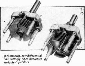
able in capacitance up to 65pF each section with 0.015in air gaps and up to 15pF each section with 0.045in gaps. The other, the C701/709, is a differential type with capacitance up to 150pF each half with 0.015in air gaps and up to 30pF each half with 0.045in air gaps.
