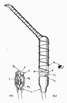
Fig. 3. (a) Construction of screened model. (b) Lead with isolating capacitor.
