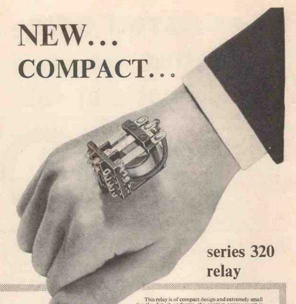
for the duty it performs, the contact arrangement is three pole double throw and connections to contact and coil are conveniently brought out at one end of the relay. Contacts and terminations are housed in a high grade Bakelite moulding and the design of the moulding gives increased creepage path and excellent insulation. Guards are fitted to avoid flashover between contacts.
