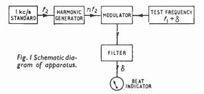
cies is through harmonic generation, for which several well-known methods exist, all involving deliberate distortion of the fundamental and then selective amplification of the required harmonic frequency.
