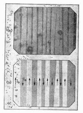
Fig. 4. (a) Photograph taken through a microscope of a powder pattern on a crystal of cobalt. The portion of the crystal recorded is about 0.025 inch across. (b) Sketch illustrating the domain structure revealed by the pattern.
