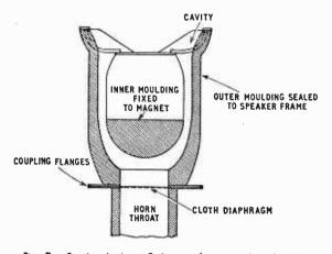
Fig. 7. Sectional view of the speaker mounting showing the method of extending the horn throat area up to the cavity at the rear of the cone.
