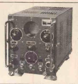
SIGNAL GENERA-TORS TF-517-F/I. Special offer of these Laboratory Signal Generators. Cover 10-18 Mc/s, 33-58 Mc/s. and 150-300 Mc/s. In good, used condition, with charts. Checked before despatch. Complete with power pack for normal A.C. mains. ONLY £12/10/- (carriage, etc.,
