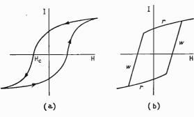
Fig. 9 (a) Typical hysteresis loop. As the applied field alternates the magnetization I follows the loop in the direction indicated. (b) Explanation of hysteresis in terms of rotation (r) and impeded wall motion (w).
