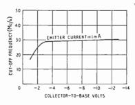
impurities in the graded base tends to give a low value of base resistance—both useful features for high-frequency operation. The alpha cut-off frequencies obtained are usually of the order of tens of megacycles. As an example, the new RCA drift transistors 2N370, 2N371 and 2N372
