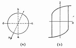
Fig. 13. Illustrating irreversible rotation in single-domain particles.
