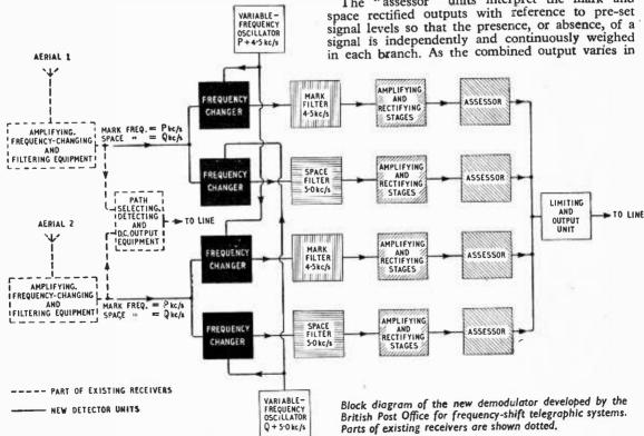
magnitude, as well as in polarity, it is further amplified and limited before passing to the land line. The circuits concerned with this operation deliver a final output of  $\pm 30$  volts d.c.
