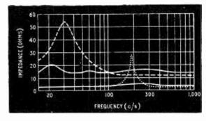
Fig. 9. Electrical impedance curves of two speakers, in the horn (full lines) and unmounted (dotted lines).
