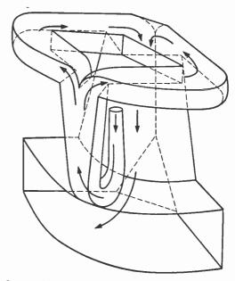
Fig. 4. Shape of the practical folded horn, showing the sound path from the small circular throat to the large quadrant shaped mouth.
