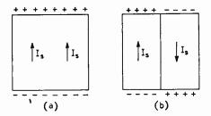
Fig. 12. Magnetostatic energies for single- and multidomain specimens.
