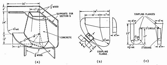
Fig. 5. (a) View of the main frame of the horn to which the final vertical section and the mouth are permanently fixed. (b) An unde side view of the mid-le part, showing the square opening which feeds into the ve tical section, and the small rectangular opening which couples to the "]"-si.aped section. (c) Two views of the "]", or throat, section.
