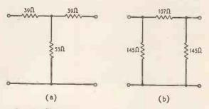
Fig. 4. These two attenuators are completely interchangeable.
