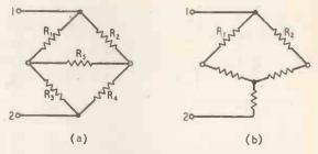
Fig. 7 . . . they fail when applied to a bridge circuit (a). However, the star-delta transformation succeeds (b).
