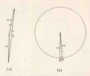
Fig. 1. The resultant of two signals of nearly equal strength and frequency varies in "instantaneous frequency" as well as amplitude, but the average frequency is exactly equal to that of the stronger signal.
