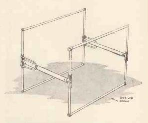
Labgear "Bi-Square" aerial, note the tuning stubs in the reflector element.
