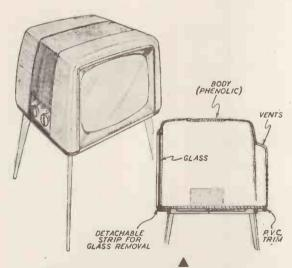
One-piece phenolic cover. Everything is there in one moulding: loudspeaker apertures, vented back, rabbet for glass with simple removal. Chassis, tube and controls mounted on plywood base. A separate centre pad in the tool could give variety in the speaker openings which could also be covered or painted to give colour changes. An extruded flexible p.v.c. trim provides a non-scratch, non-skid buffer for a polished table top and allows yet another possible colour change.
