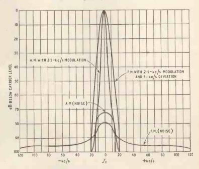
Fig. 1. Comparison of modulation and noise spectra of a.m. and r.m. transmitters designed for narrow-channel operation.
