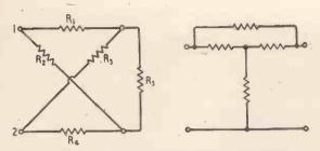
Left:—Fig. 8. This lattice circuit is just a different way af drawing the bridge—Fig. 7(a). Right:—Fig. 9. The bridged T is another network that can be simplified by the star-delta transformation.
