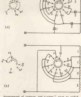
Arrangement of contacts and "wiper" rings on switch plates for (a) capacitors and (b) resistors, viewed from the The knob is assumed turned fully anti-clockwise. Dotted sketches on left show the contacts on the front surface of the wafer as viewed from the back.
