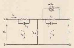
Fig. 2. High frequency equivalent circuit.
