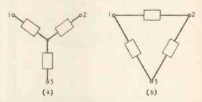
Fig. 1. Diagrams like this (or drawn with inductances in place of the oblongs) are common in books on 3-phase electric supply systems. They are called the star (a) and delta (b).
