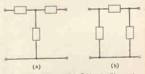
Fig. 2. These diagrams of the T (a) and n (b) networks are common in books on communication circuits, and of course are electrically the same as those in Fig. 1.
