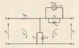
Fig. 3. The circuit of Fig. 2 rotated to represent the common emitter arrangement.
