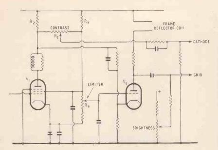
Fig. 2. H.M.V. receivers have a pentode video stage V1 with a triode black-spotter V2.
