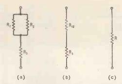
Fig. 6. The ordinary series and parallel additions can be used to find the single resistance equivalent to networks like (a), but . .
