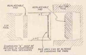
Method of changing the "face" of a cabinet. Not new, but could be more widely known. Although the body remains basically unaltered the part that really matters may be subjected to innumerable alterations.
