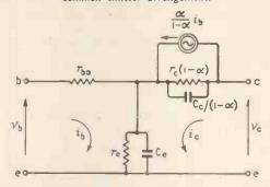
Fig. 4. The circuit of Fig. 3 modified so that amplification is expressed in terms of i<sub>b</sub>
