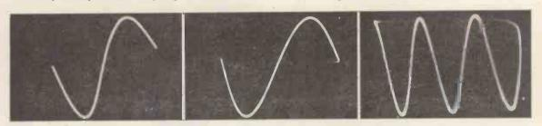
Oscillograms showing oscillator output at 3 c/s, 2 kc/s and 200 kc/s.
