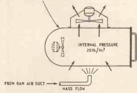
Fig. 3. Pressurized construction with external forced convection cooling by ram air or fan.
