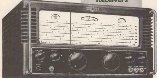
Superbly engineered and of advanced design, the two models offered possess excellent electrical characteristics and are robustly constructed for service in any climate. The "770 R" has continuous AM/FM coverage from 19 Mc/s to 165 Mc/s; the "770 U" from 150 Mc/s to 500 Mc/s. Both incorporate six-position turret tuning assemblies of unique design and giving high reliability. Fully illustrated literature with performance curves on request.
