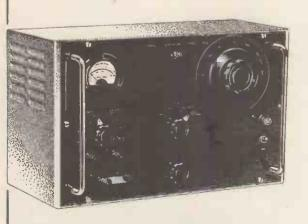
Signal Generator utilises resistance-capacitance type of oscillator to provide stable, accurate and easily controlled voltages in the frequency range 30 c/s to 30 kc/s. A screened and balanced output transformer and attenuator enable unbalanced, balanced and floating outputs to be obtained from a source of a constant 600 ohm impedance.
