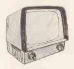
Complex curved sides, top and back in phenolic; chassis sits in virtually a plain wooden box with a fancy front. The moulding is used as a dust cover and holds tne glass and mask, the glass being detachable via the wooden trim across the front. Plain colours, stoved enamel or the patented "Oxvar" finish could be used on the phenolic cover.
