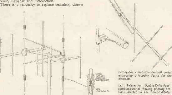
collinear half-wave dipoles operated in phase. The principle of operation is similar to that of some of the American wide-band television aerials, but in those the makers use either folded or open stubs resonating in their "high" band. The principle was explained in "Wide-Band Television Aerials" in Wireless World of June, 1956.
