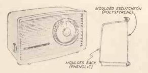
An alternative treatment of the two-piece cabinet in which the front escutcheon is constant. Either a moulded or a wrapped-ply back cover with internal fittings could be used.
