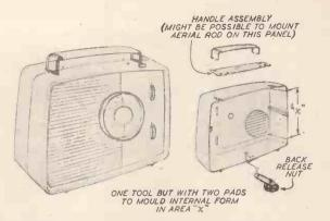
Method of achieving maximum internal flexibility in a portable with the minimum of tool cost using "identical" back and front forms, but with a slight amendment to the top tool. For example, if we require holes in the front of the cabinet we mould, say, 5,000 off. The pad is then changed to seal off those holes and 5,000 backs are moulded.
