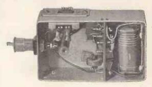
Fig. 2. Miniature crystal controlled transistor oscillator for testing v.h.f. mobile equipment (Labgear).
