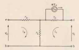
Fig. 1. Low frequency equivalent circuit.
