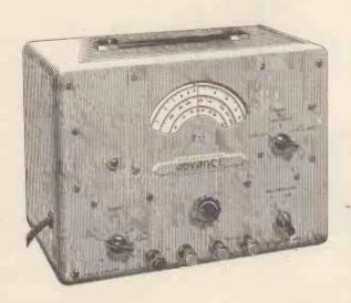
Covers from 15-50,000 c/s in three ranges. Accuracy  $\pm$  (2% + 1 c/s). Output (continuously variable) into 600 ohms. 0.1mW·1W (0.25-25v)  $\pm$  2db, output impedance approximating to 600 ohms over the whole range. Maximum output into 5 ohms is greater than  $\frac{1}{2}$ W.
