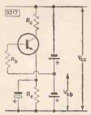
Circuit values can also be calculated, without using graphs. The procedure is as follows. (1) Choose  $V_{cc}$ ,  $V_{bb}$ ,  $I_{cnom.}$ , and  $R_{b}$ . (2) Then
