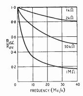
Fig. 7. Variation of  $R_{rf}/R_{dc}$  with frequency for different values of carbon composition resis.ors.
