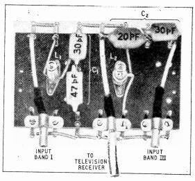
Fig. 3. Practical version of the aerial cross-over network. The thin laminated base measures  $2\frac{1}{2}\times4\frac{1}{2}$ in and should be mounted in a screening box about 2in deep
