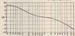
Fig. 2. Replay characteristic for coarse groove records.
