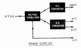
Block diagram of Mullard experimental oscilloscope.
