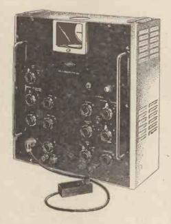
THE OSCILLOSCOPE TYPE 830 has been designed for general wideband frequency work and is particularly suitable for observing pulse waveforms with very fast rise-times. The frequency response of the Y amplifier is flat from 30 c/s to 20 Mc/s and the time-base provides writing speeds up to 20 cms. per microsecond.
