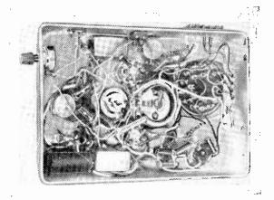
Under-chassis view of the complete 1.t.c.p. amplifier.
