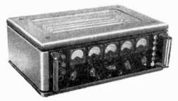
Mullard transistor counter-chronometer.
