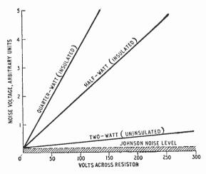
Fig. 2. Noise voltage from carbon composition resistors of the same value but different wattage ratings.
