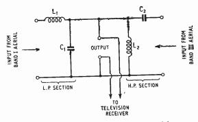
Fig. 2. Theoretical circuit diagram of the aerial crossover network.
