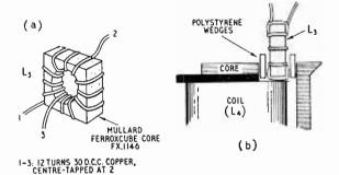
Fig. 6. Details of the experimental oscillator tuning coil and polarizing magnet for the automatic frequency correction system described.
