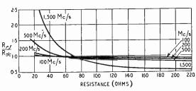
Fig. 8. Behaviour of low value carbon composition resistors at high radio frequencies.
