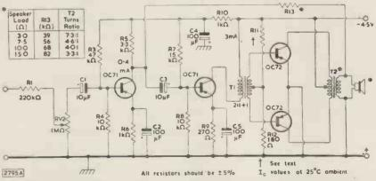
The value of R11 must be chosen from the range 6.8, 6.2, 5.6, 5.1, 4.7, and  $4.3k\Omega$  so as to adjust the total quiescent current in the output stage to 1.3mA±10% at 20°C or 1.6mA±10% at 25°C. The operating ranges with speech and music are 15°C to 45°C ambient temperature and 4.5V to 2.7V (or even 2.0V, depending on the distortion tolerated by the listener) with a Leclanché type battery.
