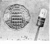
Above:- Mulla:d phototransistor compared in size with a threepenny bit.
