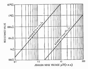
Fig. 1. Relation between Johnson noise and resistance value.
