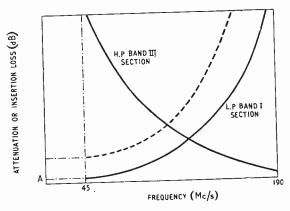
Fig. 1. Attenuation, or insertion loss, of the high-and-low pass filter sections comprising the aerial cross-over network described in the text.
