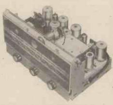
HFT111 Tuner.—An advanced 8-valve FM/AM tuner with built-in power pack designed to give high fidelity reproduction when used with amplifying equipment of comparable quality. Features: a stabilised permeability tuning system, noise limiter and phase discriminator. Attenuators provided for both FM and AM outputs.
