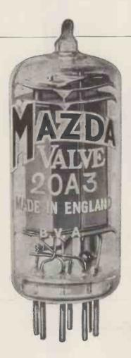
The 20A3 is a miniature indirectly heated tetrode thyratron which can be used as a high speed relay. It has a high control ratio, low grid/anode capacitance and passes a very low grid current. Used in conjuction with a high resistance circuit, the 20A3 can be operated directly from a high-vacuum photo-cell.
