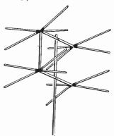
Fig. 4. Two forward tilted conical dipole aerials (with reflectors) stacked vertically for fringe areas.
