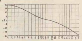
Fig. 1. Replay characteristic for microgroove records.
