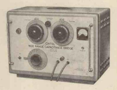
Designed for the accurate measurement of capacitance and resistance in the range 0.002pF to 100 $\mu$ F and 1 $\Omega$  to 10,000M $\Omega$  respectively.
