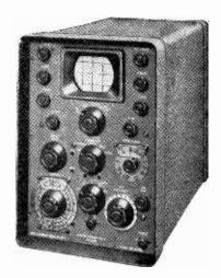
Marconi Instruments alignment oscilloscope, Type TF1104.
