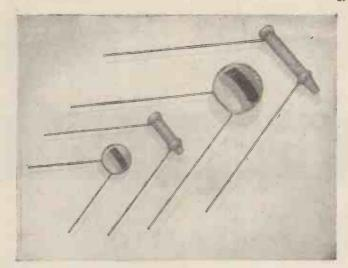
Hunts announce their new ranges of Tubular and Disc Ceramics. Precise in their characteristics and robust in design, these capacitors are available in High-K, High-Q and Special Purpose Tubulars and in High-K Discs.
