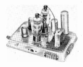
Amplifier with "replacement" output transformer.
