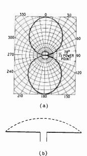
Fig. 1. Polar diagram (a) and current distribution (b) of a half-wave dipole cut for Band 1.
