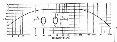
Amplification/frequency characteristic of the i.f. amplifier, measured between A and B.
