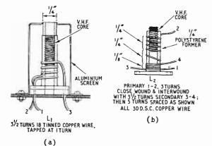
Above: Fig. 3. Constructional details of the v.h.f. tuning coils,  $L_1$  and  $L_2$ .
