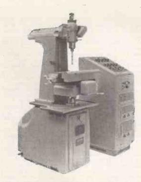
Electronically controlled drilling machine. The required position of the work-table is set up initially on the control desk (right).
