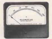
Rectangular panel instruments are available with scale lengths of 2.5", 3.2", and 4.2". These offer the advantage of an increase in scale length of approximately 50% over their equivalent round models, for which they can be used as direct replacements using the same panel fixing boles.
