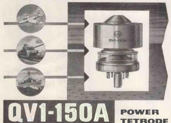
The new Mullard QV1-150A is an external anode tetrode of exceptionally small dimensions, completely interchangeable with the popular American 4X-150A. It is forced-air cooled and will operate with excellent efficiency and power gain at frequencies as high as 500 Mc/s.
