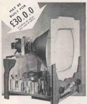
THE COMPLETE TELEVISOR IS SAFE TO HANDLE, BEING COMPLETELY ISOLATED FROM THE MAINS BY A DOUBLE WOUND MAINS TRANSFORMER. ALL PRESET CONTROLS CAN BE ADJUSTED FROM THE FRONT, MAKING SETTING UP VERY SIMPLE.
