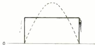
Fig. 3. The mean or average of the half-wave (dotted) is the same as that of the flat-topped half-wave having the same area under it.
