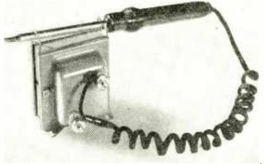
The iron on a rest fixed to the transformer
