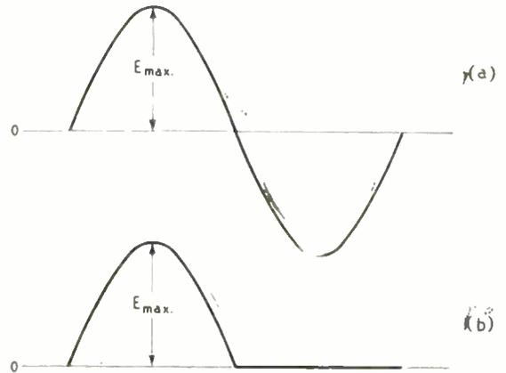
Fig. 2. The voltage waveform (a) delivered by the generator, and (b) appearing across the load resistance,  $R_L$ . (b) is just the first half-cycle of (a), followed by no voltage for the next half-cycle.
