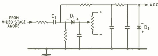
Fig. 4. A.g.c. circuit of H.M.V. fringe-area receiver.
