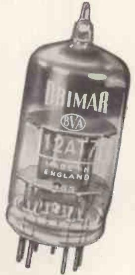
The 12AT7 is a very reliable frequency changer and is widely used in modern TV receivers, VHF and UHF communications equipment. It is also frequently employed in industrial equipment, computers, navigational aids and test equipment.
