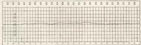
Although manufactured under the same conditions as Type '88' and having all the special features, Type '77' undergoes an individual "Pen Test" examination for accuracy of sensitivity. Each reel is "Pen Tested" throughout its entire length to ensure a level of sensitivity not exceeding  $\pm \frac{1}{2}$  dB, and an overall variation from reel to reel not greater than  $\pm 1$  dB. A typical example of a "Pen Tested" chart is given above.
