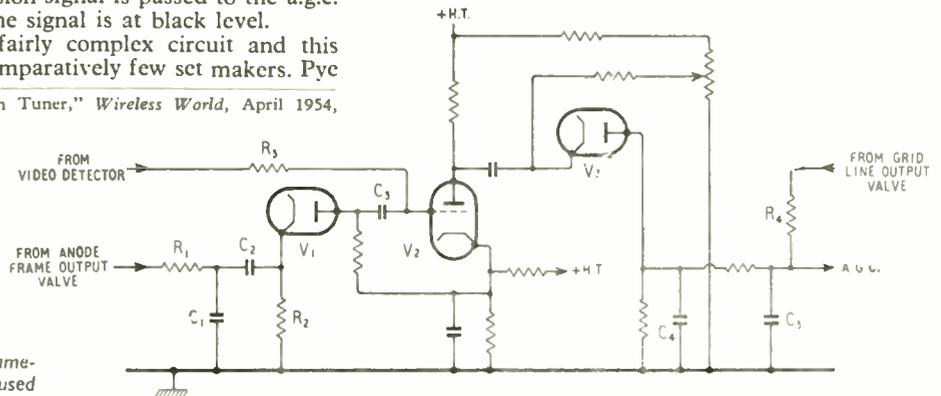
Fig. 2. Arrangement of frame-pulse gated-a.g.c. system used by Ultra.
