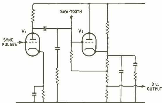
Fig. 5. Kolster-Brandes phase detector for flywheel sync.
