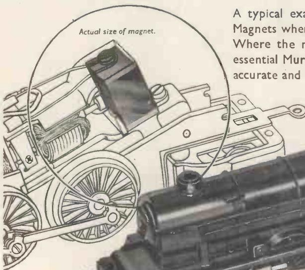
A typical example of the use of Murex Sintered Permanent Magnets where a stable source of energy is required. Where the need for high magnetic stability and efficiency is essential Murex Sintered Permanent Magnets continue to give accurate and reliable service.
