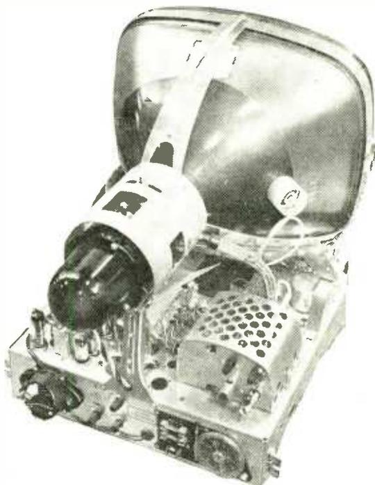
Murphy chassis. Note the thorough screening of the line timebase, the deflector-coils and the inter-connecting leads.
