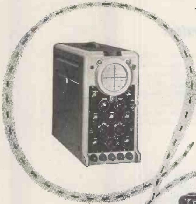
Two similar amplifier channels with an approximate gain of 2000 and an upper frequency response of 5 megacycles ( $-6\text{DB}$ ) are features of this new Cossor Double Beam general purpose oscillograph. The repetitive or triggered time base has a sweep duration from 200 milliseconds to 5 microseconds.
