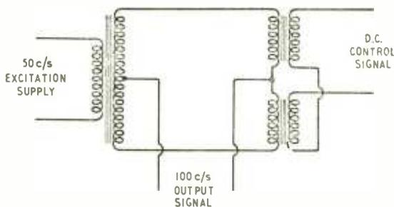
Fig. 3. Basic circuit of second-harmonic magnetic modulator.
