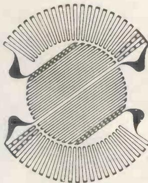
Technograph patents throughout the world now cover various alternative processes including the basic technique of making electrically conductive patterns by either the etching of metal foil previously laminated to any of the various types of insulating base, or the etching of foil patterns from metal insulated on one side by means other than laminating and bonding. These patents, together with numerous applications still pending, cover many fundamental aspects of the new technology.
