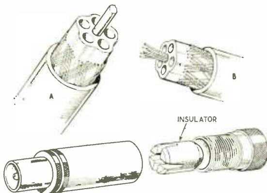
Aerialite semi-air-spaced coaxial cables (enlarged 4-5 times.) A is the "Super" and B the "Standard." Easy-fix plug also shown.
