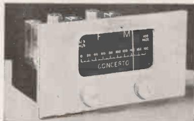
6 Stage high sensitivity F.M. feeder unit with built-in A.C. power supply. Complete band II coverage. Grounded grid triode low noise R.F. stage. High stability frequency changer. 2 stages of high gain I.F. amplification. Latest type ratio discriminator using balanced diodes. Pre-set control for minimum A.M. noise. Special de-emphasis circuit. One stage of high fidelity L.F. amplification. Specially designed for F.M. reception and ease of operation.
