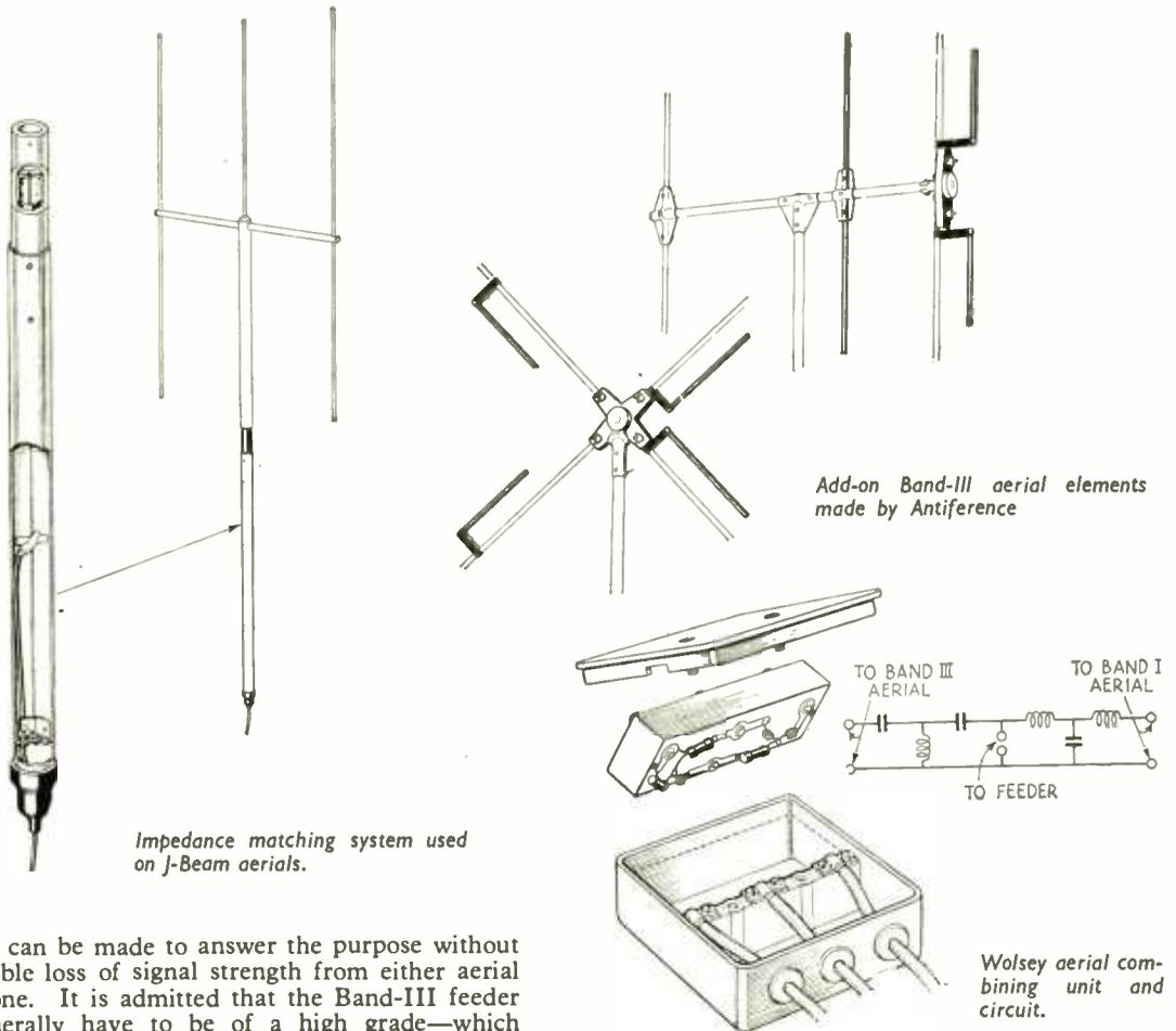
Impedance matching system used on J-Beam aerials.
