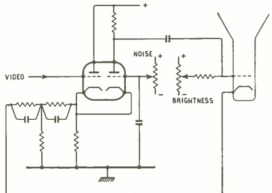
peak white. When it conducts amplified interference voltages appear at the anode in the same phase and are applied to the grid of the tube. Because of the amplification the noise signal on the grid can exceed that on the cathode and so black out the spot.
