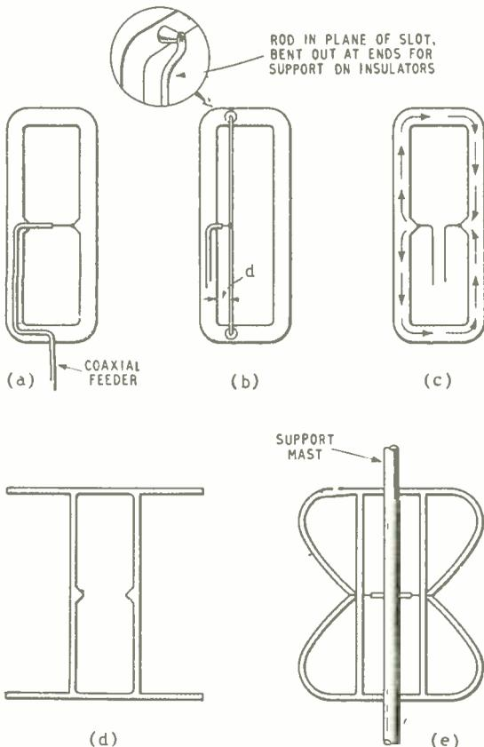
of a slot aerial is not a new idea and is, incidentally, the subject of a B.B.C. patent application (No. 19736/51). I should imagine that the single reflector illustrated by Mr. Dent achieves gain in the horizontal plane at the expense of the vertical polar diagram and that it would be better to use two rods, stacked half a wavelength apart and approximately level with the ends of the slot.
