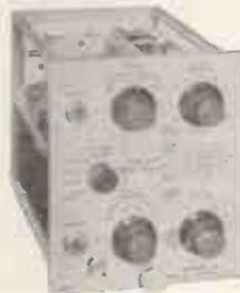
**Type 53C Dual-Trace Plug-In Preamplifier**—two identical amplifier channels, each with dc to 8.5-mc passband, 0.04- $\mu\text{sec}$  risetime, sensitivity 0.05  $\text{v/cm}$  to 50  $\text{v/cm}$  continuously variable with 9 calibrated steps from 0.05  $\text{v/cm}$  to 20  $\text{v/cm}$ . Electronic switching triggered by oscilloscope sweep, or free running at about 100 kc. Polarity reversal switches. Price \$275.
