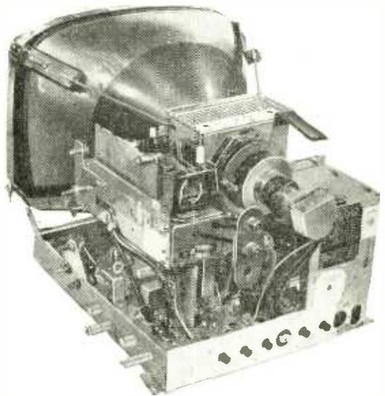
Ultra chassis. The tuner is mounted on the near side so that the controls project through the side of the cabinet.
