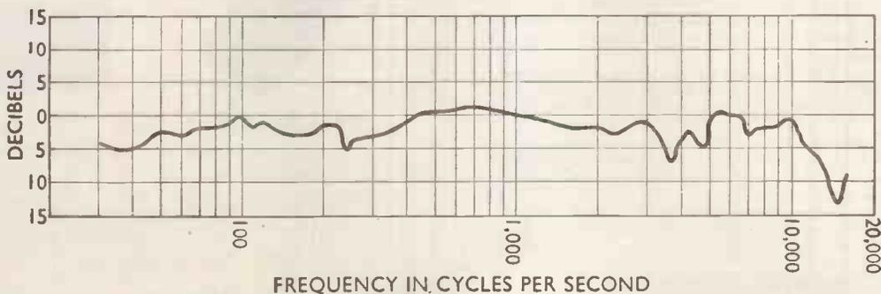
Overall frequency response of the complete equipment, comprising L.P. record, specified pick-up, Osram 912 amplifier and G.E.C. Metal Cone Loudspeakers in octagonal loaded port-cabinet.
