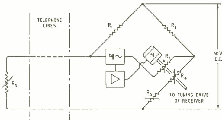
Fig. 1. Basic bridge circuit with remote resistance control.
