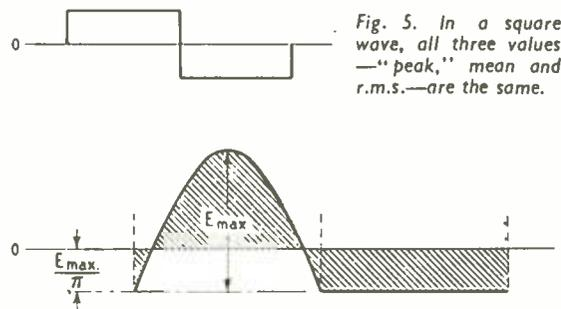
Fig. 5. In a square wave, all three values—"peak," mean and r.m.s.—are the same.
