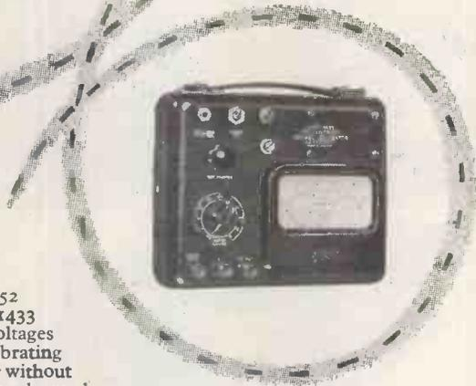
Primarily designed to be used with the Model 1052 oscillograph the Cossor Voltage Calibrator Model 1433 provides an accurate means of calibration of input voltages to the plates or amplifiers of any oscillograph. Calibrating voltages are read directly from a wide scale meter without any computation being necessary. Measurements can be made to an accuracy of  $\pm 5\%$  and the instrument can be used in any application where a source of accurately-known voltage is required.
