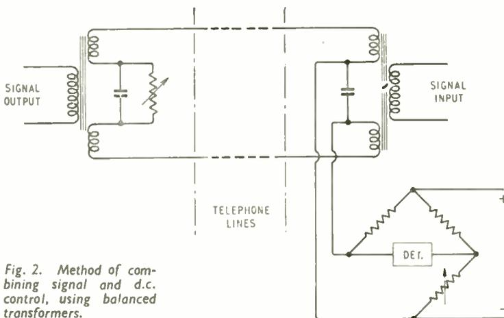
Fig. 2. Method of combining signal and d.c. control, using balanced transformers.
