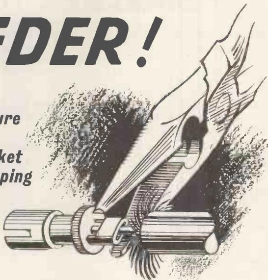
A VERY common fault in domestic television installation is the careless manner in which feeders are attached to co-axial plugs and sockets. Often the feeder is merely pushed through the co-axial pin without soldering, leaving a loose, dry joint.
