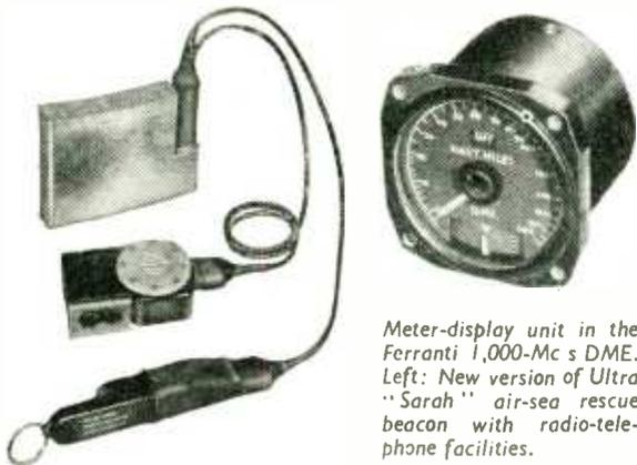
Meter-display unit in the Ferranti 1,000-Mc/s DME. Left: New version of Ultra "Sarah" air-sea rescue beacon with radio-telephone facilities.
