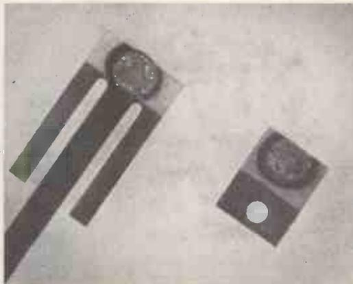
*After 200,000 operations at 230 volts, 15 amps. A.C., the contacts of a short break snap-action switch were still free from pronounced pips and craters.*
