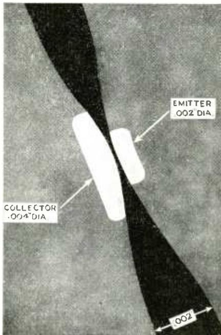
Left: Fig. 2. Photomicrograph of section of etched wafer. The white areas show the relative sizes of the indium electrodes.
