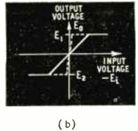
Fig. 5. Arrangement of biased diodes to simulate a mechanical system with limits on displacement, rate or torque.
