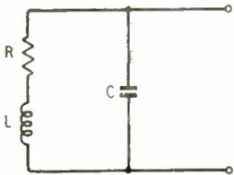
Fig. 3. Equivalent circuit of a carbon resistor.
