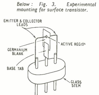
Below: Fig. 3. Experimental mounting for surface transistor.
