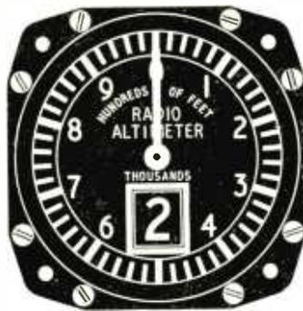
Fig. 5. Face of the height indicator. The full scale represents 1,000 ft, so the pointer makes five revolutions for 5,000 ft. Integral thousands are clocked-up in the window at the bottom.
