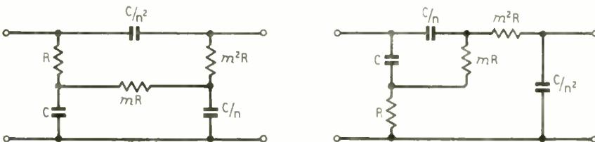
Fig. 10. The series- $\pi$  network on the left can be twisted round to give the step-up network on the right. This form is especially convenient for use with valve circuits.
