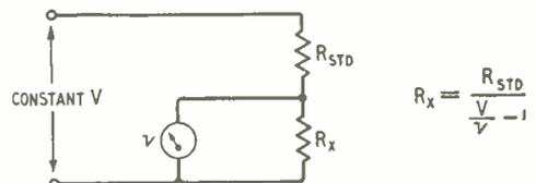
Fig. 3. Circuit of Fig. 2 altered to give readings near full-scale deflection when  $R_x > R_{STD}$
