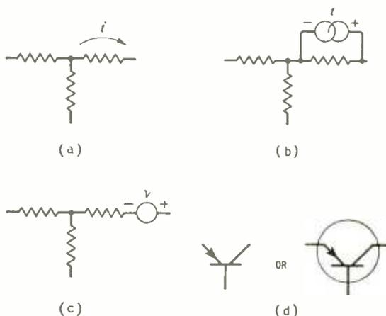
advantage that the current source appears *connected* to the rest of the circuit which is not the case with the arrow symbol of (a).
