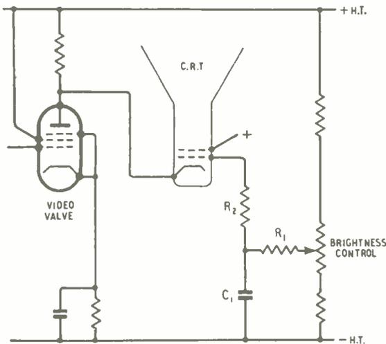
the accompanying diagram, the time constant  $C1R1$  serving to hold the grid voltage up to ensure that the e.h.t. capacitor is discharged through the tube. The grid limiting resistor is  $R2$ .
