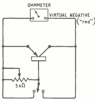
Left: Fig. 6. Circuit for demonstrating the function of a transistor as a bistable switch.
