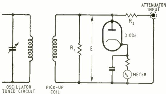
Fig. 7. Typical coupling circuit between oscillator and attenuator.
