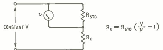
Fig. 2. Basic circuit of electrostatic megohmmeter ( $R_x < R_{STD}$ )
