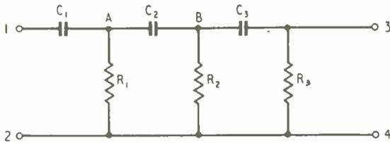
Fig. 4. Resistance-capacitance circuit used in the phase-shift oscillator.
