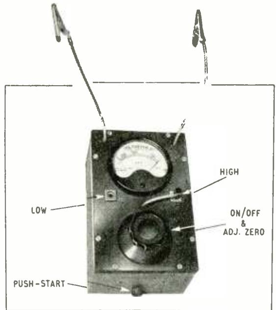
Polythene-insulated leads and wander-plug switching are employed. The meter is of the electrostatic type.
