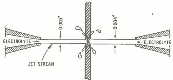
Above: Fig. 1. Etching of germanium wafer by jets of electrolyte.
