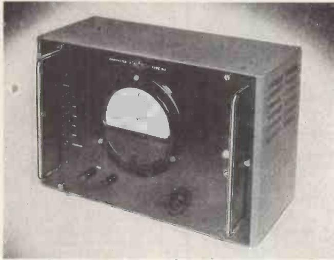
**T**HE AIRMEC OHMMETER is intended for production and laboratory continuity testing, and enables the value of any resistance between 1 ohm and 10 Megohms to be rapidly determined. A large meter, having a scale length of approximately 7 inches, is employed, thus enabling excellent reading accuracy to be obtained.
