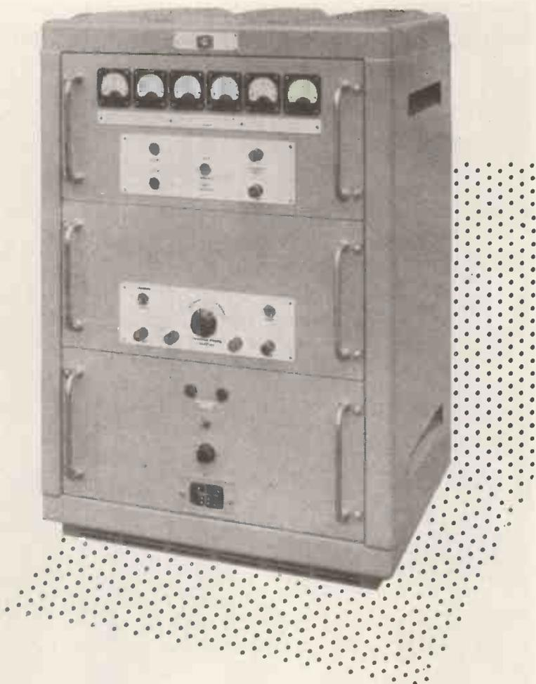
Designed for the measurement of any frequency in the range 10 c/s to 1 Mc/s with a basic accuracy of  $\pm 0.005\% \pm 0.1, 1.0, \text{ or } 10 \text{ c/s}$ .
