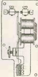
Extra light weight, extra sensitive for high speed or radio control work, weight only 1 1/2 oz., closes on 2 mA., solid platinum changeover contacts, adjustable pressure. Price. 13/6.
