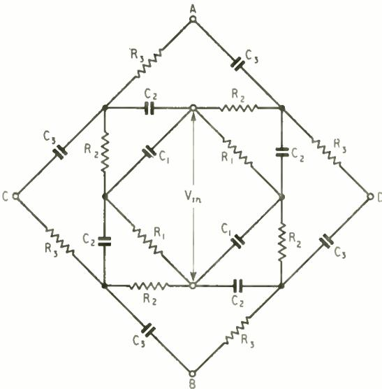
Fig. 9. Four-phase step-up network giving a measured gain of 1.67 at 640 c s.  $R_1 = 100\Omega$ ,  $R_2 = 1k\Omega$ ,  $R_3 = 50k\Omega$ ,  $C_1 = 2.5\mu F$ ,  $C_2 = 0.25\mu F$ ,  $C_3 = 0.005\mu F$ .
