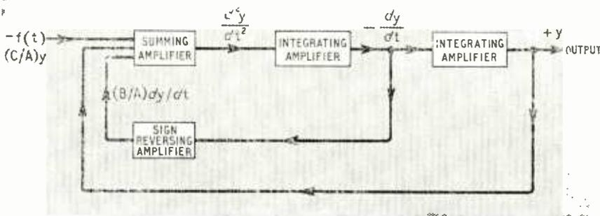
Left: Fig. 3. Four d.c. amplifiers arranged as a differential analyser.
