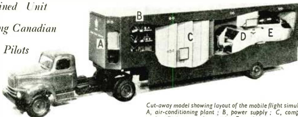
Cut-away model showing layout of the mobile flight simulator. A, air-conditioning plant; B, power supply; C, computer racks; D, instructor's console; E, cockpit.
