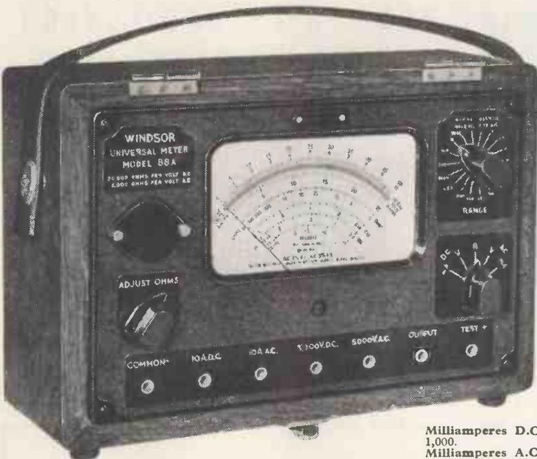
Five inch moving coil meter with knife-edge pointer and anti-parallax mirror. Instantaneous overload protection. Buzzer for continuity testing.
