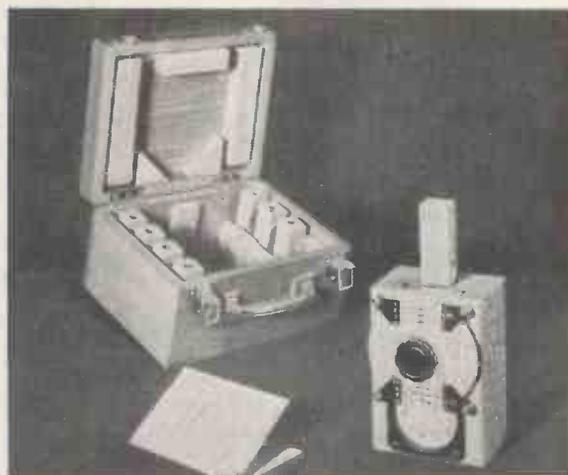
circuit in which resonance is indicated by a sensitive moving-coil micro-ammeter with crystal rectifier. It has an accuracy of  $\pm 3\%$ . For carrying purposes, a polished hardwood case accommodates the instrument and its eight plug-in coils.
