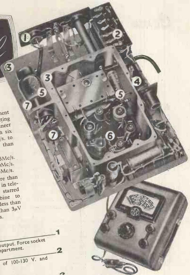
An inexpensive yet precision instrument designed especially to meet the exacting needs of the modern service engineer and laboratory technician. With six frequency ranges covering 50 Kc/s. to 80 Mc/s., its accuracy is better than  $\pm 1\%$  of the scale reading.
