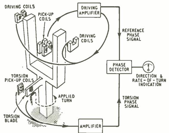
Fig. 1. Essentials of the experimental vibratory gyroscope.
