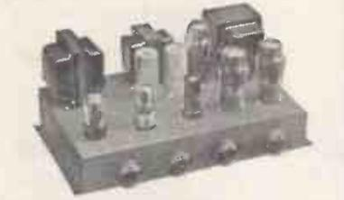
Nusound 8 1/2 watt Quality Amplifier = PP 6V6— independent Bass and Treble boost and cut—neg. Feedback—provision for Radio Feeder Unit—Freq. response 25 to 20,000 c.p.s. + 1dB—hum 80 DB down at 6.5 watts—Feedback 14 DB. Available with Remote Control Unit. Price £17/10/-, or as illustrated.
