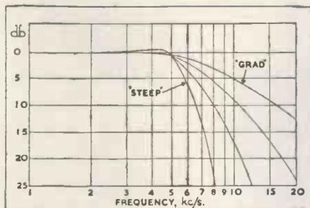
Representing a unique feedback circuit development, the "Vari-Slope" pre-amplifier gives audibly better reproduction. This advance consists of variable slope "electronic" low-pass filters operating on negative voltage feedback principles. No Inductors ("Chokes") are used, and their disadvantages are completely eliminated. The turnover frequencies are 5kc/s, 7kc/s, and 9kc/s, and the slopes of attenuation are continuously variable over the range 5db to 50db per octave.
