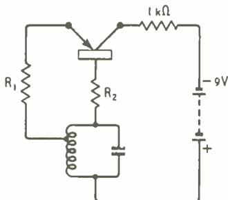
Fig. 8. Sine-wave oscillator using the astable switching circuit.
