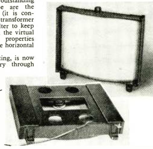
E. D. Parchment, 69, Clapham Road, London, S.W.9. It consists of a curved perforated back-plate with a stretched diaphragm of plastic film, coated on the outside with a metallic film. The whole is housed in a moulded plastic frame measuring approximately  $4\frac{1}{4}$  in  $\times$   $3\frac{1}{4}$  in  $\times$   $\frac{1}{2}$  in.
