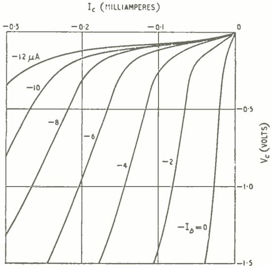
Fig. 4. Earthed-emitter characteristic of the surface-barrier transistor.
