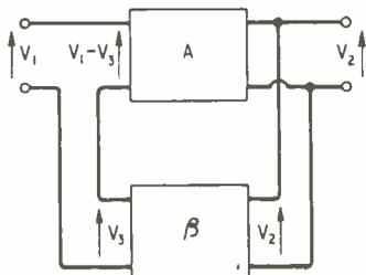
Fig. 1. The basic feedback amplifier or oscillator consists of the amplifier  $A$  and the feedback  $\beta$ .
