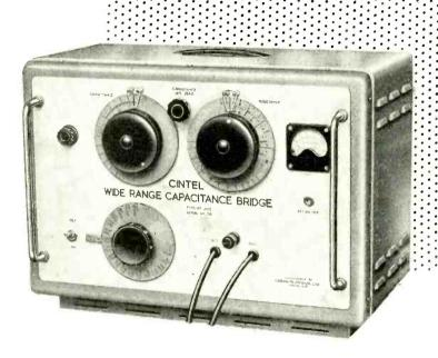
For the accurate measurement of in situ capacitance or resistance, all measurements being made in the form of a three terminal network.
