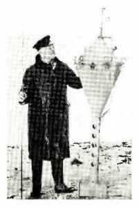
WHALING BUOY. Lightweight version of Venner's standard radio-transmitting dahn buoy (see Nov. 1952 issue, p. 468) for marking whales after the kill to facilitate recovery by the parent ship. It has a range of 30 miles and radiates for 22 hours. being arranged for overseas visitors to the exhibition.
