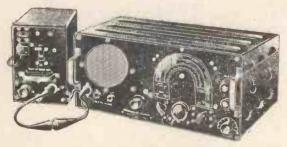
16-50, 200-550 and 800-2,500 metres. R/F, F/C, 2 1.F's D.D.T. Pentode Output. Spin-wheel tuning. In black metal case with built-in speaker. Complete with power pack A.C. 300-250 v. Can also be supplied with 12 v. D.C. power pack if required. BRAND NEW— EX-GOVT. #17.10.0
