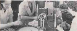
Soldering capacitors at A. H. Hunt Limited. The capacitors are heated together with short pre-cut lengths of Ersin Multicore.
