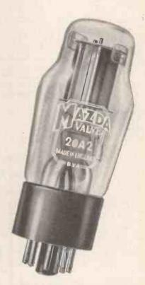
IMPORTANT: Cathode and Heater should normally be tied externally. If left free the *Heater to Cathode Voltage* must never exceed 25 volts peak. The heater must be switched on for 15 seconds before anode voltage is applied.
