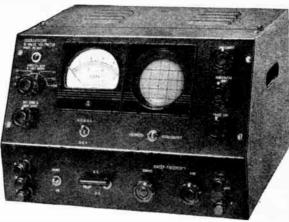
THE VOLTASCOPE—A combined valve-voltmeter and oscilloscope. VALVE-VOLTMETER—Infinite Input oscilloscope. OSCILLOSCOPE—3 inch screen tube provided with balanced amplifiers for Y and X plates giving a 5 times. trace expansion. Maximum sensitivity 150mV/cm. Response from D.C. to 100 kcs.
