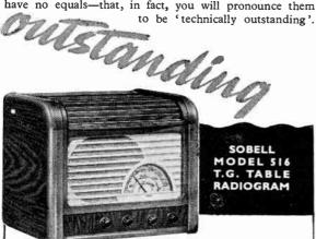
Roll top gives easy access to gramophone turntable. The receiver is a 5-valve super-het. operating from 200/250 volts, 40/100 cycles per second A.C. supply. Wave range: 16-50 metres; 193-577 metres; 800-2, 140 metres.
