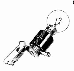
All parts plated and keyed to body. Available in bracket or clip-fixing types.
