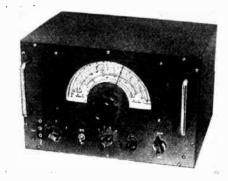
Labgear optional pre-selector or convertor unit for A.C. operation.
