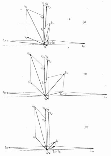
Fig. 3. Vector diagrams of action of "Stabilistor": (a) supply voltage low, load maximum; (b) supply voltage high, load maximum; (c) supply voltage high, no load. The effect of choke L at 50 c/s is assumed to be neglible.
