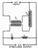
Fig. 2. Basic circuit of the "Stabilistor."
