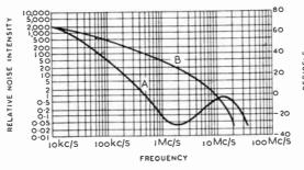
Variation of radio noise with frequency at noon (A) and at midnight (B) in the Northern temperate zone. From curves given by R. K. Potter, Proc. I.R.E., Sept. 1932.
