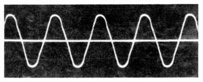
Fig. 4. Oscillogram of the output voltage waveform of a "Stabilistor," showing the low harmonic content, compared with Fig. 1.
