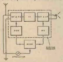
Fig. 1.—Block diagram showing the additions necessary to obtain a test signal from an existing receiver.
