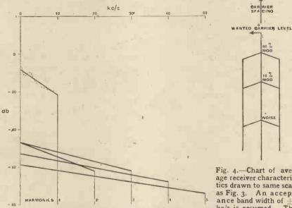
Fig. 3.-Average distribution of fundamental and harmonic sidebands in one half of the spectrum radiated from a transmitter modulated roo per cent, by a 75-instrument orchestra playing at "maximum" level. Sideband levels are referred to the carrier.
