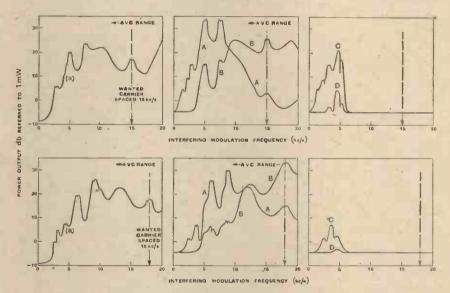
Fig. 2.—Curves (a) : Magnitude of sideband interference resulting from 10,000  $\mu$ V undesired signal spaced 15 kc/s and 18 kc/s from 100  $\mu$ V wanted carrier. Curves : A, no filters in unwanted "transmitter"; B, RF filter only; C, AF filter only; D, RF and AF filters both in circuit.
