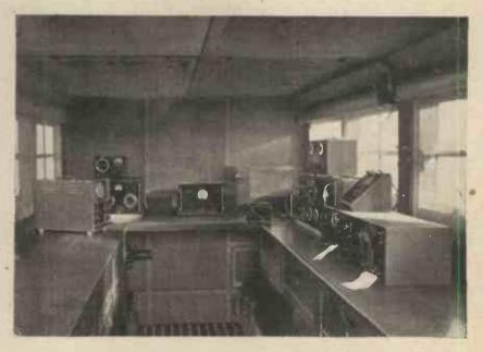
A mobile test room mounted on a six-wheel lorry chassis. Some of the test apparatus with which it is equipped can be seen on the benches. Lockers and drawers under the benches contain other apparatus, tools and spare parts.
