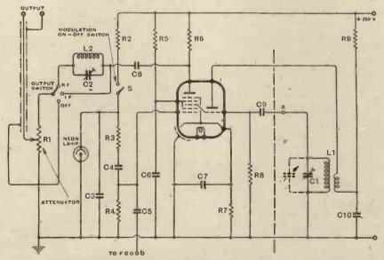
Fig. 3:—The mixer circuit shown in this diagram is suitable for a portable unit. Component values are: R1,  $100\Omega$  var.; R2, 2 M $\Omega$ ; R3, 2 M $\Omega$ ; R4, 25,000 $\Omega$ ; R5, R6,  $10,000\Omega$ ; R7,  $300\Omega$ ; R8,  $30,000\Omega$ ; R9, 25,000 $\Omega$ ; C3, C4,  $0.001\mu$ F; C5,  $50\mu\mu$ F; C6, C7,  $0.1\mu$ F; C8;  $0.01\mu$ F; C9,  $0.0001\mu$ F; C10,  $0.1\mu$ F. Valve: Mazda TH41.
