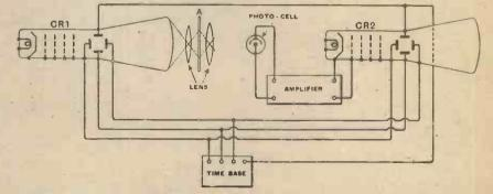
The diagram shows the connections adopted for CRI and CR2 to create a positive image of a photographic negative.
