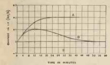
Fig. 2.—Frequency drift of the circuit shown in Fig. 1. Curve A uncompensated, curve B compensated by negative temperature coefficient condenser. The positive change in IF is due to the oscillator being on the low frequency side of the signal.
