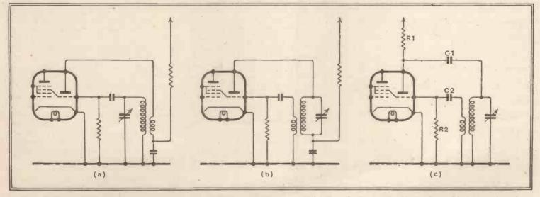
Fig. 8.—Three arrangements of the reaction-coil oscillator are shown here. At (a) there is the tuned-grid circuit, at (b) the tuned-anode, while (c) shows the shunt-fed tuned-anode oscillator.
