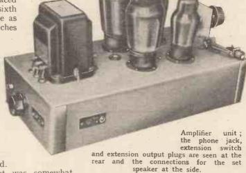
operation, when required, a jack was mounted near this switch; there was some difficulty in connecting the phones, since with a push-pull amplifier there is no suitable point in any early stage. It was found, however, that the voltage available across a 15-ohm speaker, or resistance, was just about of the right order to give a satisfactory signal, with high-resistance phones, at normal settings of the volume control
