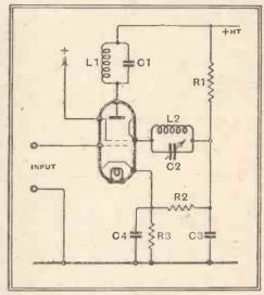
Fig. 2. As a frequency-changer the valve needs only a tuned circuit L2C2 connected in the auxiliary cathode lead.
