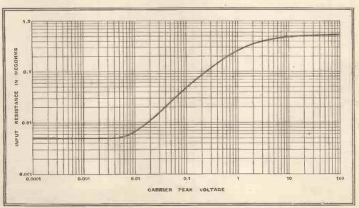
Fig. 8.—This curve illustrates the variation of input resistance with signal input voltage for I volt positive bias on the diode and RI equal to IM... The diode AC resistance is 5,000 ohms.
