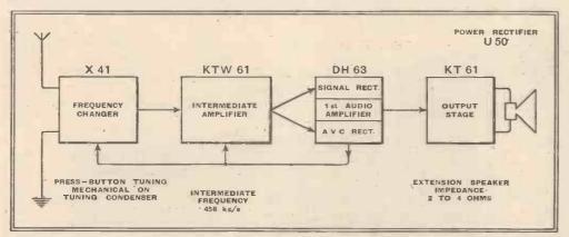
Schematic circuit diagram of the G.E.C. Model 4050.
