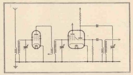
Fig. 9.—The skeleton circuit of the receiver as so far discussed is shown in this diagram.
