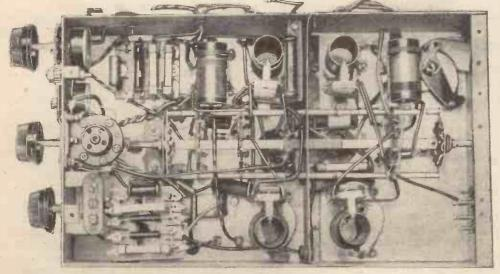
Underside of the pre-tuned unit; note the two panels carrying, respectively, the diode and the phase-changer components; also the small panel mounting for the 200-0hm resistor in the cathode of the RF pentode, and that for the voltage dropping resistance fitted near the dividing screen. The 8-mfd. condenser for detector decoupling is under the AF output terminal strip at the front of the chassis.
