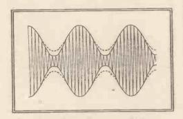
Fig. 9.—The variation in the input resistance of the diode affects the damping of the tuned circuit and distorts the input voltage waveform as shown here.
