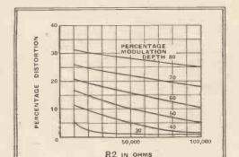
Fig. 3.—These curves show the effect on distortion of varying R2 for various modulation depths. The signal input is 40 volts
