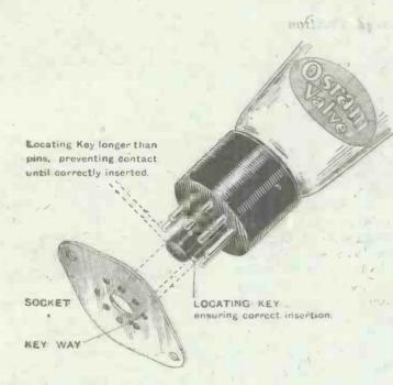
The utility of the valves with the self locating octal base is becoming firmly established, and designers and others will appreciate the introduction of new types having characteristic advantages hitherto not obtainable in this range.
