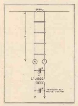
Fig. 26.—Tuned feeder system for a centre-fed half-wave aerial where a is an odd number of quarter-waves long
