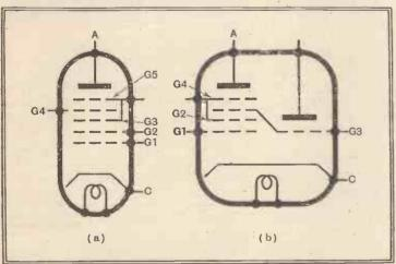
In the heptode GI is the oscillator grid, G2 the oscillator anode, G3 and G5 are screen grids, which are maintained at a fixed potential, while G4 is the signal grid. In the triode-hexode GI is the signal grid, G2 and G4 are screen grids, while G3 is the oscillator grid. Both valves, of course, may have an extra electrode outside the outer screen to reduce the effects of secondary emission; they then become octodes and triode-heptodes respectively.
