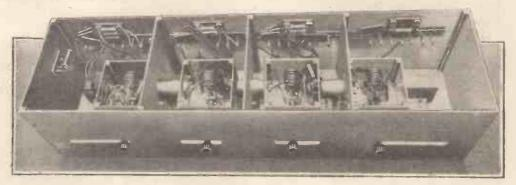
A receiver embodying the new valves and designed for operation at 40 Mc/s is shown here.
