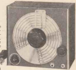
The meter is direct-reading, with separate scales for each of the bands covered.
