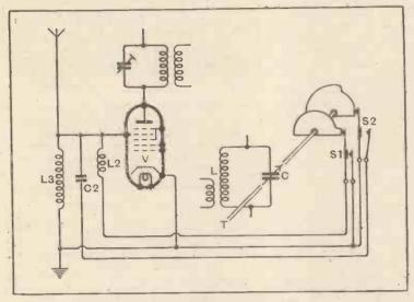
Cam-operated switches providing automatic extensions of wave-
