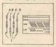
Tuning scale with automatically registering cursor.
