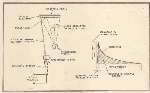
Fig. 1.—In this diagram is sketched the arrangement of a simple storage system with secondaryemission modulation.
