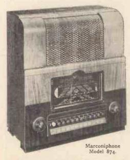
The Model 874 for AC mains is basically a four-valve superheterodyne with an additional double diode for automatic frequency control. This is a refinement in a pushbutton receiver with individually tuned
