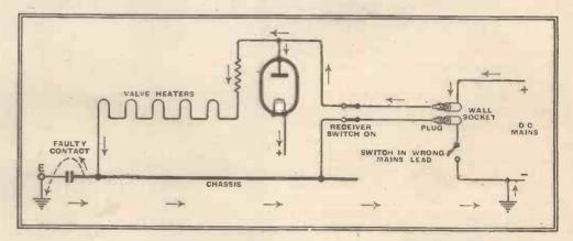
The arrows show the path of the current through the receiver, notwithstanding the wall switch being "off."
