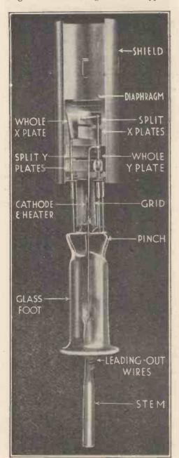
Fig. 13. Bedford tube incorporating von Ardenne's split-plate arrangement for avoiding origin distortion.
