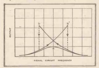
Fig. 3.—Variation of output with tuning due to the effect of AVC bias.
