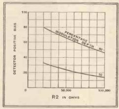
Fig. 6.—These curves show the relation between R2 and the positive bias for minimum distortion; again, for a signal input of 40 volts.
