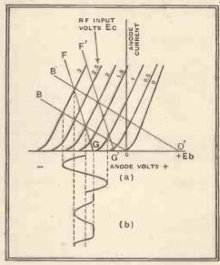
Fig. 7.—The DC load line is indicated by OB and the AC load line by FG. If the former only were operative the output would be undistorted (a), but when FG is the working line there is distortion as shown at (b). The use of positive bias shifts the load lines to O'B' and F'G' and obviates the distortion.
