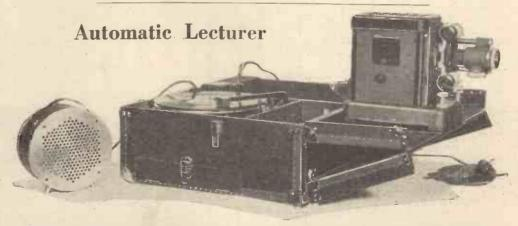
Portable equipment is being demonstrated by the Telefunken Company which enables talks previously recorded on slow-motion 15-minute discs to be amplified and, where necessary, illustrated by means of short films or lantern slides from a projector incorporated in the unit. The necessary breaks in the recording to permit the showing of particular slides can be timed during the recording. It is claimed that a satisfactory "lecture tour" can be carried out by anyone able to operate the gear.
