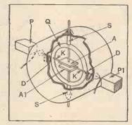
Ultra-short-wave valve with compensation against the effects of heat.
