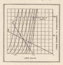
Fig. 12.—The grid-volts anode-current curves of the negative feed-back detector reveal its close relationship to the diode with positive bias.
