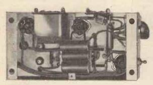
Underside of the chassis on which all the components of the unit are assembled.
