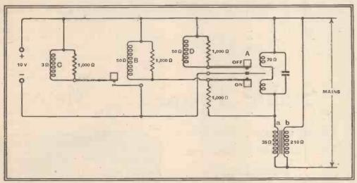
Fig. 5.—Circuit diagram of the relay unit simplified by excluding details such as switching for "local" receiver operation, to make the relay actions clearer.
