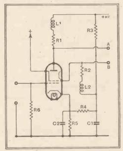
Fig. 3. Used for a VF stage the output to the sync separator can be taken from the auxiliary cathode in opposite phase to the output at the anode, which is fed to the CR tube.
