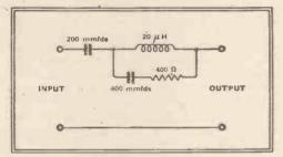
Fig. 4.-Standard all-wave dummy aerial.
