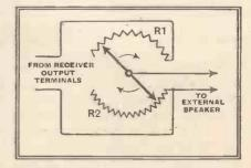
Constant impedance volume control near the "minimum" position. As volume is increased RI is reduced and R2 increased. The value of RI should be approximately equal to the loud speaker impedance and R2 about five times the resistance of RI.
