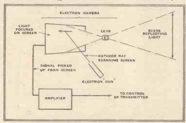
.—Very diagrammatic view of what goes on at the transmitting The light on the screen releases electrons according to its brightness, and when touched by the scanning ray a signal is obtained; but to be any good it must at least be much stronger than the amplifier "noise."
