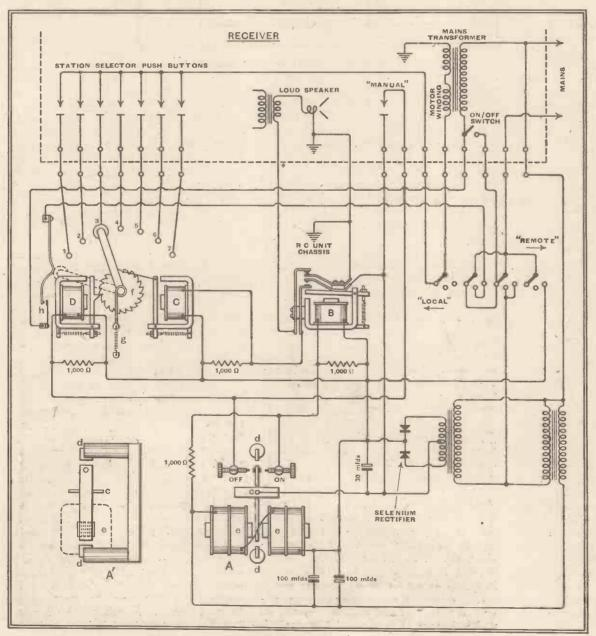
Fig. 4.-Full circuit diagram of the relay unit.
