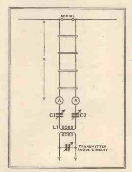
Fig. 27.—If the tuned feeders are an even number of quarter-waves long, a half-wave aerial should be arranged in this way.
