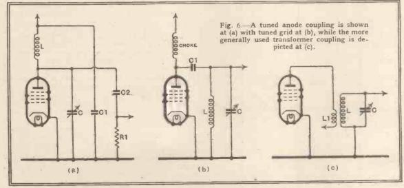
give very similar results, but primary and secondary are completely isolated at audio-frequency. There is also much more scope for varying the characteristics of the stage. The performance does not now depend only on the valve and the tuned circuit but also on the primary inductance LI and its coupling to the secondary.
