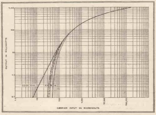
Fig. 10.—A muting action can be obtained by the use of positive bias on the diode and this is well brought out by these input-output curves of a receiver.
