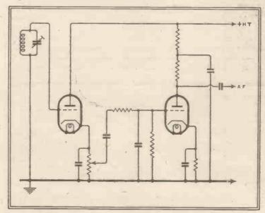
always passes through  $\mathrm{E} a = \mathrm{O}$ ; we should then be able to accept a roo per cent. modulated carrier with practically no output distortion.
