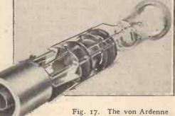
Fig. 17. The von Ardenne polar co-ordinate oscillograph. Circuit for use with the polar co-ordinate oscillograph (a). Variation of circle diameter due to application of potential to be examined is seen to the right of the circuit (b).
