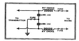
Fig. 21.—An RF filter in the mains leads to the transmitter may be needed to prevent interference with broadcast sets.
