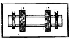
Fig. 1.—Arrangement of coupling transformer providing variable selectivity by means of staggered tuning.
