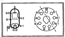
Arrangement of electrodes and base connections. The dotted line across the valve holder indicates the correct positioning of the interstage screen located below the chassis.
