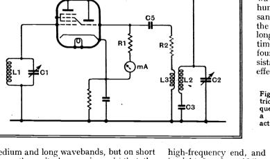
Fig. 1.—A typical triode - hexode frequency-changer with a tuned-anode reaction coil oscillator is shown here.
