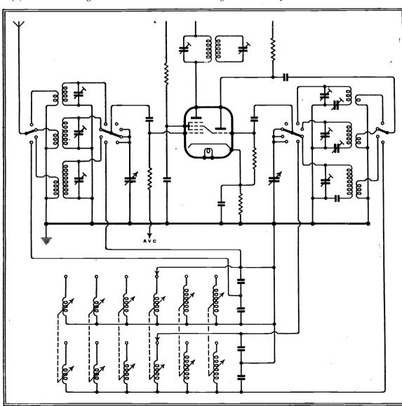
Fig. 2.—Arrangement of manual and press button circuits of a three-band superheterodyne receiver.
