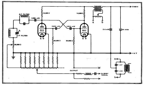
Fig. 2.—Complete circuit of a multi-vibrator with component values. The instrument is designed for a fundamental frequency of 500 c/s.
