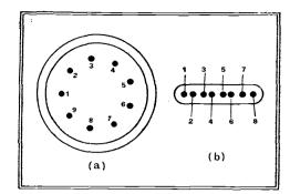
Fig. 4.—This diagram shows at (a) the base arrangement of the new valves and at (b) the pinch of a conventional type.
