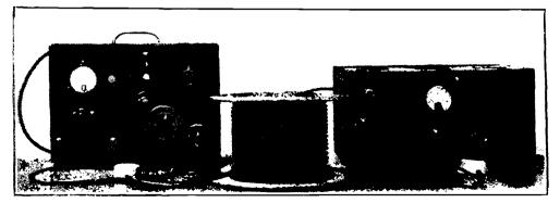
Apparatus for the measurement of cable losses.
