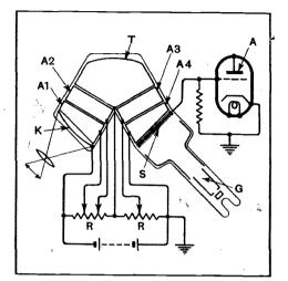
anodes, A<sub>3</sub>, A<sub>4</sub>, which focus it on to a screen S of the mosaic-cell type. The image charges set up on this screen are then scanned
