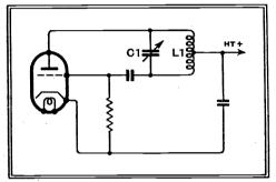
Fig. 5.—A typical Hartley oscillator.
