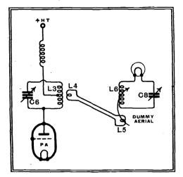
Fig. 12.-Method of coupling the PA anode circuit to a dummy aerial, using a low-impedance link (twisted flex).
