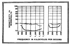
Fig. 4.—Sensitivity of manually tuned circuits, shown in full lines, compared with that of press button circuits (dotted lines).
