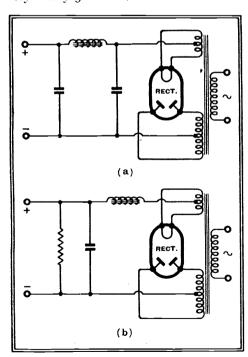
Fig. 13. The conventional reservoir condenser circuit (a) compared with a choke input filter (b).
