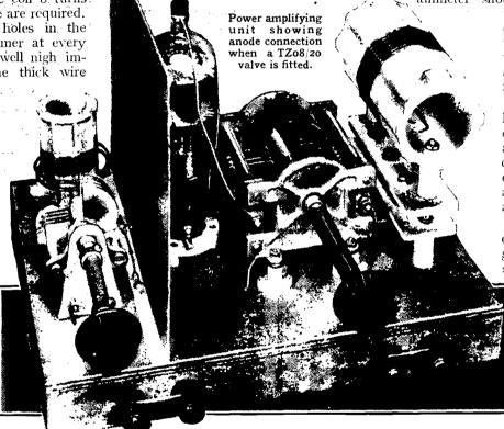
TZo5/20, and this is a very good example of an inexpensive power triode for amateur wavelengths. Its filament requires 6 volts at I.I amps and the valve capacities are not unduly high. This firm have just introduced a new transmitting valve of the same power rating but with appreciably smaller valve capacities and having the anode lead brought out to a plug connection on the top of the bulb. It is suitable for use down to five metres and it is known as the TZo8/20.
