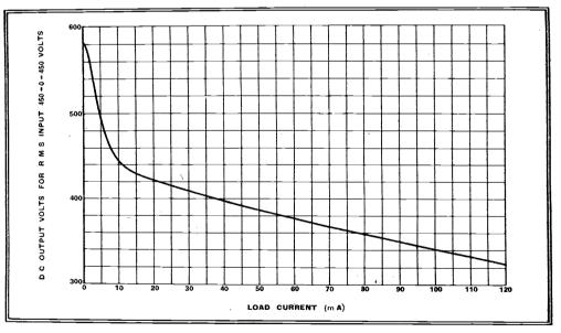
Fig. 17. Output voltage curve for the unit described.
