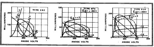
Fig. 1.—Typical load diagrams for triode, pentode and tetrode output valves, showing the possibility of distortion through the ellipse cutting the base line.
