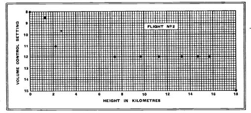
Some description is necessary of the scale of field strength. The volume control of the receiver was calibrated with a scale from o to 15, o being the minimum
