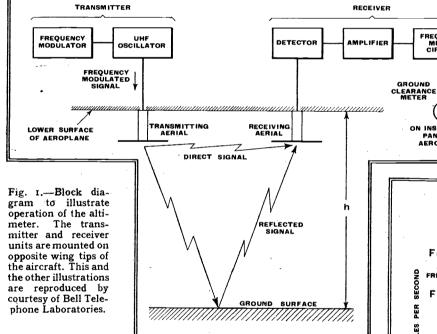
signal employed in making the measurements. Since the ultra-high-frequency transmitter is installed in the plane, and aircraft conditions are severe, this is no minor problem. Both difficulties have been avoided very neatly in the new Western Electric Model I altimeter recently described before the American Institute of the Aeronautical Sciences by Lloyd Espenschied and R. C. Newhouse, of the Bell Telephone Laboratories (New York City).
