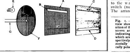
Fig. 1. — Exploded view showing disposition of the rotatable screen and the two indicating scales, which are opaque respectively to horizontally and vertically polarised light.
