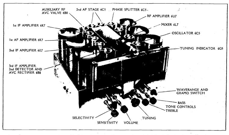
Large diameter screening cans make for high efficiency in the IF circuits. The tuning scale is indirectly illuminated and calibrated in wavelengths on medium and long waves, and megacycles on the two short-wave ranges.
