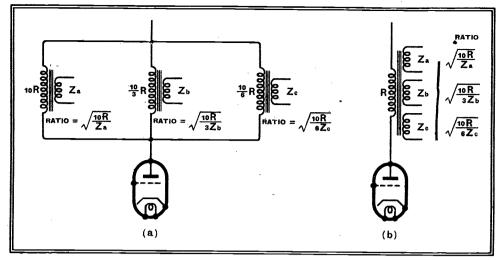
Fig. 3.—Equalising diverse loading by means of multiple transformers.
