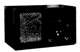
COSSOR MODEL 70. A two wave-band AC superheterodyne with five valves including rectifier. The output valve is a triode and an 8-inch loud speaker is incorporated in the horizontal - type cabinet. Station in the horizontal - type cabinet. Station names are printed on a black background and the price is 8½ guineas.
