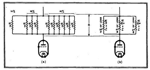
Fig. 2.—Extending the idea illustrated in Fig. 1 by imposing several unequal loads.
