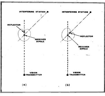
from one particular direction. The familiar dipole with reflector is of this type. As usually erected, the reflector is placed behind the dipole so that reflector, dipole, and transmitter all lie on the same straight line. This gives the maximum signal strength and it also gives the minimum pick-up from an interfering signal if this is located on the same straight line projected backwards.
