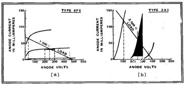
6.—The damping effect on the loud speaker represented by the shaded area (a) for a pentode compared (b) with a triode.
