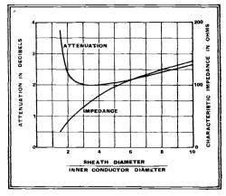
Fig. 3.—Cable attenuation and characteristic impedance for single concentric cable with sheath and inner conductor of copper. For convenience a dielectric constant of unity is assumed in estimating impedance.
