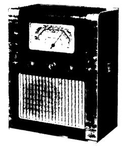
Cossor Model 31 all-wave 4-valve battery receiver.
