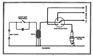
nected to the engine crankshaft in such a manner that the contact-breaker provides the necessary primary current and subsequent high-voltage secondary pulse at the appropriate firing time, while the distributor arm selects the appropriate sparking plug.
