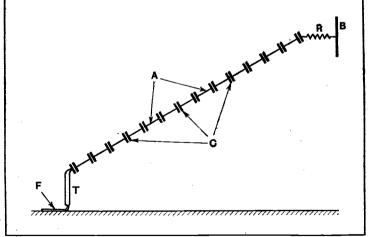
Television aerial with condensers inserted at short intervals in the lead-in wire.
