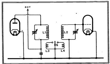
Fig. 2.—How the windings of the transformer of Fig. 1 are connected.
