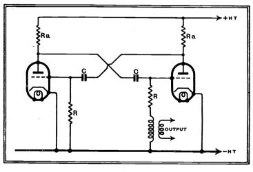
sists of two resistance-coupled valves in which the anode of each is coupled to the grid of the other. This arrangement is oscillatory and produces a signal extremely rich in harmonics. The frequency of the fundamental oscillation is dependent upon the time constant of the grid circuit. The frequency may be fixed, or locked by the
