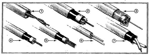
Fig. 1.—Construction of various single and twin cables as used for high-frequency work.
