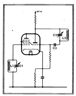
Fig. 2.—The modified Colpitt's oscillator can be used with a triode-hexode if the tuning condenser is not earthed.
