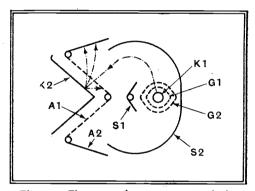
Fig. 2.—The general arrangement of the electrodes is shown here together with the electron paths.
