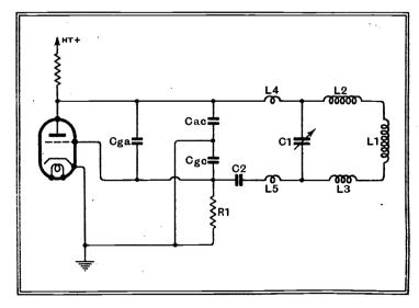
Fig. 4.—When the tuning condenser is connected directly to the valve the equivalent circuit takes this form.
