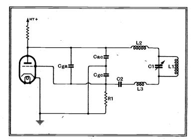
condenser should be adjustable with a minimum capacity of about 1-2  $\mu\mu$ F. and a maximum of some 6-10  $\mu\mu$ F. Additional capacity in either of these latter points enables the effective tapping point on the tuned circuit to be changed. Normally, the tapping point is provided by the valve capacities—the grid-cathode and anodecathode capacities being in series across the circuit.
