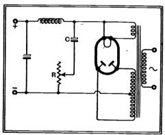
Fig. 1.—With this circuit, which differs from the standard arrangement only in the introduction of a variable resistance R, the output voltage can be controlled without affecting the regulation.
