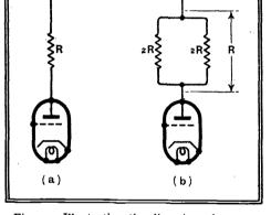
Fig. 1.—Illustrating the diversion of power in an output anode circuit into two separate loads.
