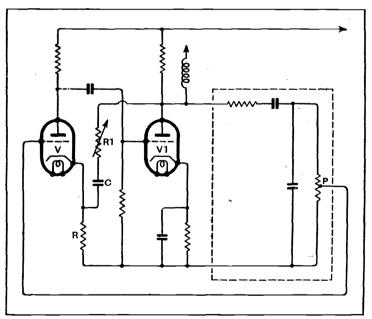
Feed-back circuit for generation or selective amplification of oscil-
