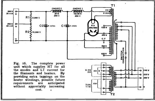
does not exceed 5 per cent. of the HT voltage it is usually satisfactory for the power amplifier of a CW telegraph transmitter. For the oscillator, frequency doublers and pre-amplifiers I per cent. of ripple is tolerable, while for telephony transmitters the ripple must be reduced to no more than 0.25 per cent.
