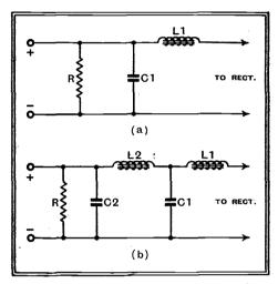
Fig. 15. Designs for smoothing filters for telegraphy and telephony transmissions.
