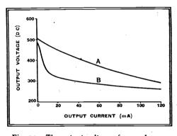
Fig. 14. The output voltage of a condenser input filter (A) is lower but better regulated than that of a choke input filter (B).
