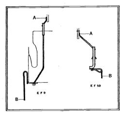
Fig. 3.—The lengths of the internal cathode leads for the EF9 and the new EF50 are well brought out in these sketches.
