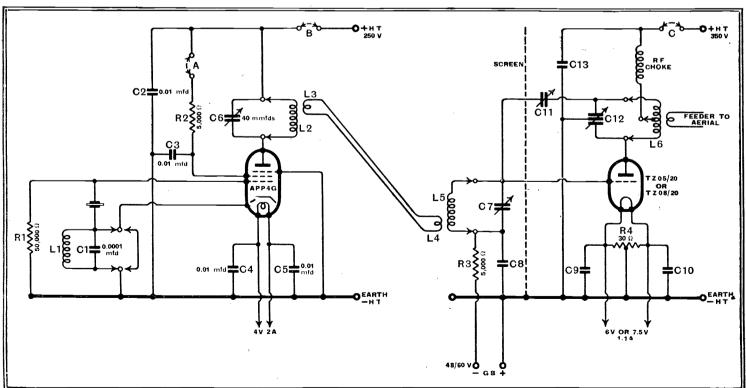
Fig. 18.-In this circuit are three points, A. B and C, where a key for telegraph transmission can be inserted; the merits of the various keying
