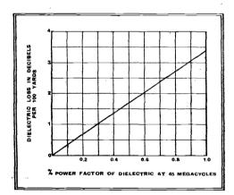
Fig. 2.—Showing the effect of different dielectrics on cable losses. Cable constants: L, 0.46 microhenrys per yard; C, 46.4 m-mfds, per yd.; Z, 100 ohms.
