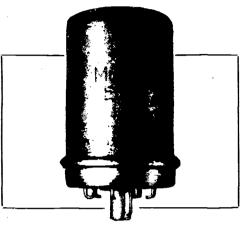
Mullard EE50 "all glass" valve which supersedes the original secondary emission valve TSE4.
