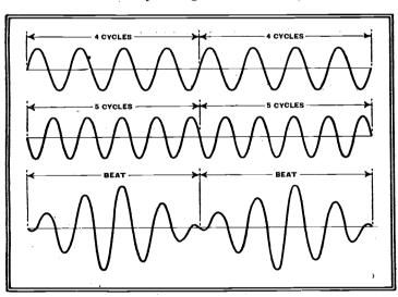
Fig. 1.—Production of a beat note between two oscillations of different frequency.
