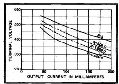
Fig. 2.—Regulation curves of the circuit of Fig. 1, using a type 5Z3 rectifier and for different values of R.
