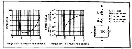
Fig. 2.—Electrical characteristics and equivalent circuit of a 10-inch moving coil loud speaker.
