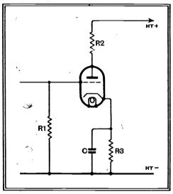
Fig. 2.—Feed-back along R3 can be avoided by using a large-capacity by-pass condenser C.
