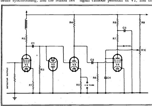
Fig. 5.—This circuit can be recommended as being highly satisfactory, simple to put into operation, and free from the disadvantages of most alternatives. V1 is the VF stage and V2 the DC restoring diode. V3 is a phase-splitter and the CR tube is fed from its cathode while the sync separator V4 is fed from its anode.
