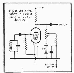
obtained, enough to provide almost pertect AVC, a great advantage for receivers required to work with very small aerials.
