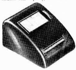
STATION-FINDING MADE EASY.—This "rotary station log" contains a 12-ft. length of tape, on which is printed information relating to over 1,600 broadcasting stations throughout the world. Stations Stations are listed in order of frequency, and, as the device is of American origin, in order of call-signs as well. One knurled disc rotates the drum carrying the tape, while the other controls an indicator showing standard zone time.
