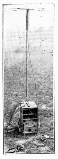
ONE - MAN BROADCASTING STATION. Complete short-wave transmitting and receiving equipment that can be carried on the back. Designed by the Telefunken Co., the apparatus, which weighs approximately 42 lb., has an effective broadcast range of just over three miles.
