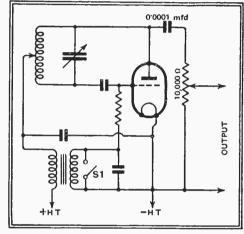
Fig. 2. The addition of a few simple components will convert the circuit of Fig. 1 into a useful testing oscillator.
