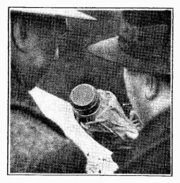
BRAVING THE ELEMENTS. German commentators, even in bad weather, can fearlessly go about their tasks at (openair events when using this waterproof-covered microphone.
