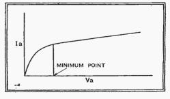
Fig. 3. In operation, the volume expander functions over a linear part of the valve characteristic.
