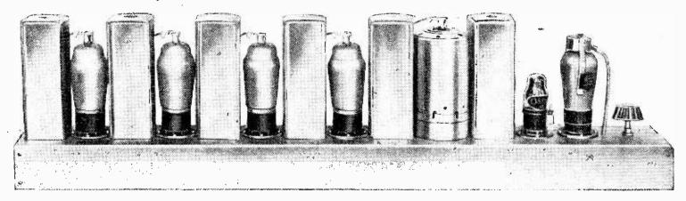
The single-diode detector can be seen in this experimental receiver adjacent to the last screening can.
