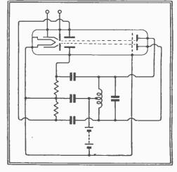
Fig. 4.—The deflection valve as a generator of oscillations.
