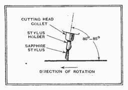
Correct method of mounting sapphire stylus for cutting "Simplat" type records.
