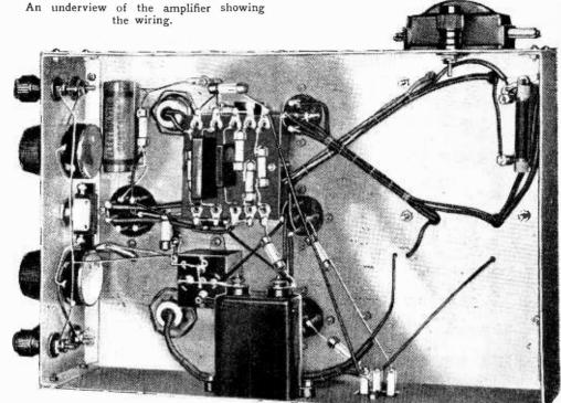
course, be earthed, and the amplifier itself should be earthed. The external connections for a microphone are given in Fig. 3; a battery is advised for energising the microphone since it is simpler than taking
