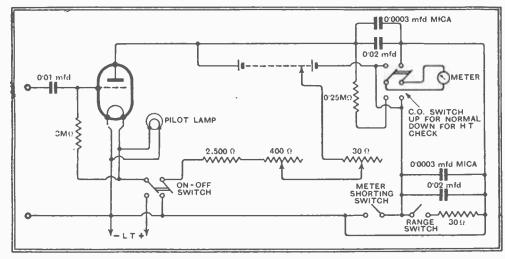
Fig. 3.—Complete circuit diagram of the two-range valve voltmeter.
