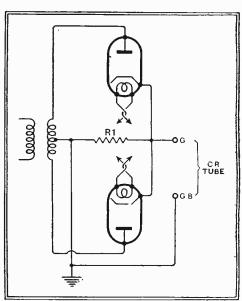
Fig. 13.—Two diodes are needed for a pushpull detector and the input transformer must be very carefully designed.
