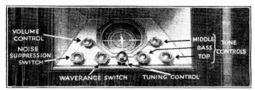
An excellent example of a multi-knob control panel which caters for the critical listener.
