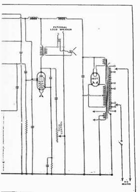
response by the AF tone control. Starting from the normal position and turning the control in a clockwise direction, on the other hand, leaves the AF response at maximum, but increases the band width of the IF amplifier to give the highest degree of fidelity of which the set is capable.
