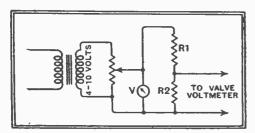
Fig. 4.—Calibrating the meter from the mains with the help of an AC voltmeter.
