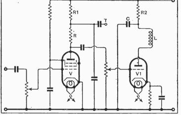
Method of separating frame and line sync signals in television apparatus.
