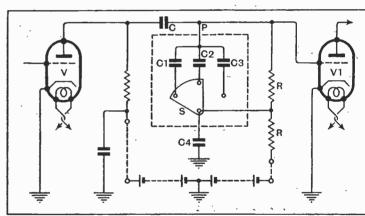
Tone control circuit evolved for silent operation during adjustment.
