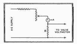
Fig. 6.—Another method of calibration: in this case the current flowing through R is measured, and the voltage developed across it is calculated.
