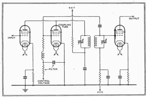
Fig. 3.—In this circuit an RF pentode varies the coupling between the two circuits of an IF
