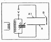
Electrode assembly in a coldcathode electron - multiplier
