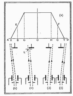
Fig. 2.—Illustrating the operation of the deflection valve.
