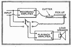
Fig. 5.—Arrangement for aural comparison test.
