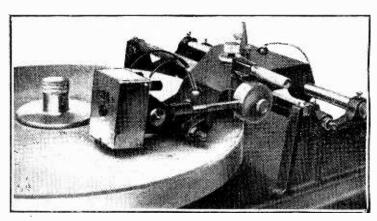
Cutting head and traversing mechanism of the Parmeko recorder.
