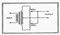
Fig. 1 (above) The fundamental volume expansion circuit,
