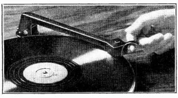
"PERMANENT" PICK-UP. Weighing only 25 grams, this pick-up, recently introduced by Siemens in Germany, is fitted with a sapphire needle capable of playing 5,000 single sides of 12-inch records without deterioration of frequency response. The output level of 40 millivolts is maintained up to at least 10,000 cycles.
