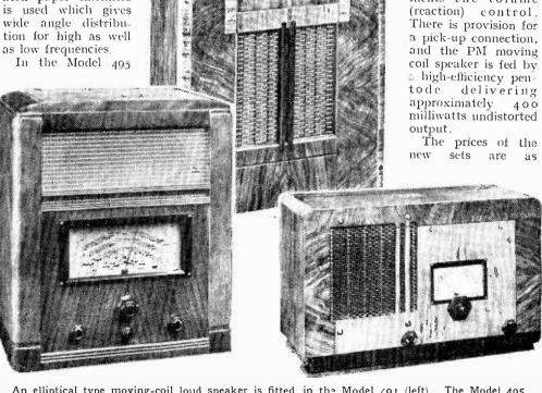
An elliptical type moving-coil loud speaker is fitted in the Model 491 (left). The Model 495 adiogram (top) has outside controls and occupies very little floor space. A station call brated dial, and improved selectivity are features of the Model 167 battery receiver (right).
