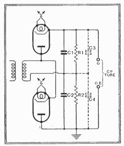
Fig. 15.—The voltage-doubler detector can be regarded as two diode detectors with their output in series.
