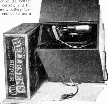
With the exception of the LT battery, the meter is self-contained. The components are secured to the top panel, and space is provided for the HT battery in the base of the container.
