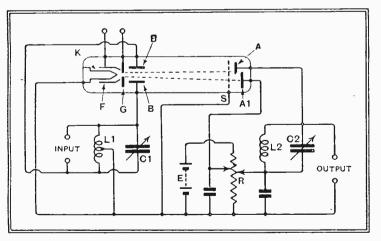
Fig. 1.—The simplest deflection valve circuit, as arranged for RF
