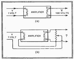
Fig. 1 (a) A straightforward amplifier. (b) The same, with the addition of degeneration. What happens is described in the text.
