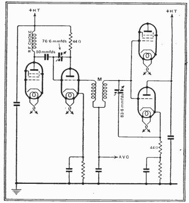
Fig. 2.—An ASC circuit which utilises two triodes to mistune the primary and secondary circuits in opposite directions.
