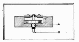
For good results with plain aluminium discs the distance between the pivot A and the cutting needle point B should be as short as possible.
