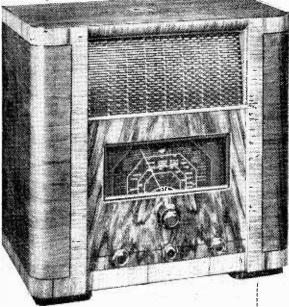
N the range of H.M.V. "All-World" receivers, comprising thirteen models, this set occupies a position between the multi-range sets capable of receiving television sound and the less expensive receivers with a single short-wave range. In common with the latter sets it has a short-wave band covering 16.5 to just over 50 metres, but in this case a stage of RF amplification is included which considerably increases the range and selectivity on all wavebands.
