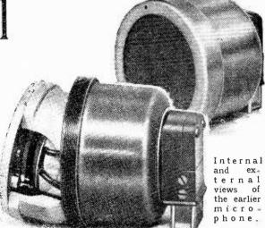
The moving-coil microphone was designed to avoid noise due to the wind when used out of doors. It was also inconspicuous as compared with a condenser microphone and its necessary preamplifier, and very much more robust.
