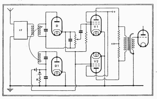
Fig. 4.—A system in which muting is controlled by the output of the IF amplifier of a superhet.
