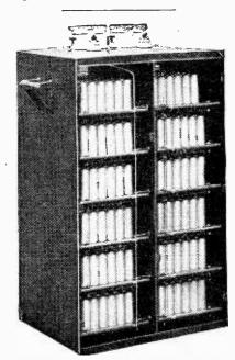
HIGH CAPACITY .-- A bank of T.C.C. wet electrolytic condensers totalling 2,500 mfds. designed for working at 600 volts DC.
