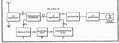
Fig. 1.-A schematic diagram showing the general arrangement of a receiver including automatic tuning.
