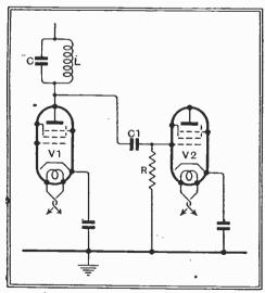
The basic tuned-anode circuit is shown in this diagram. For the highest efficiency the tuning condenser C consists merely of the valve and stray capacities.
