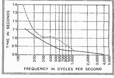
Fig. 4.- Reverberation curve of a mediumsize studio at Broadcasting House.
