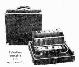
followed by a driver stage transformercoupled to two PP $_3/250$  valves in push-pull. There is also an HT valve rectifier. A multiratio output transformer is fitted to enable matching for one or for a bank of loud speakers. Incorporated in the case is a rotary transformer for battery operation.
