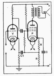
Method of emphasising bass response in a resistance-capacity coupled AF amplifier.
