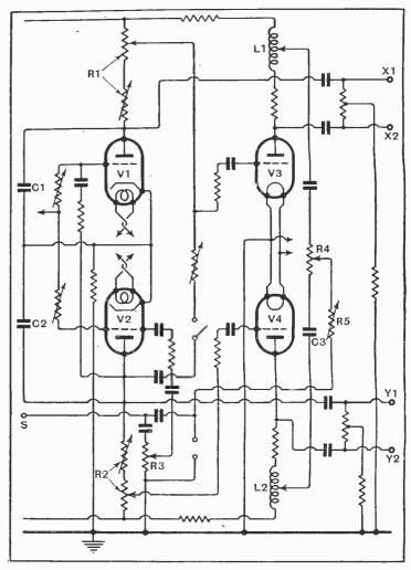
Time-base circuit with provision for intermittently extinguishing the cathode-ray beam.
