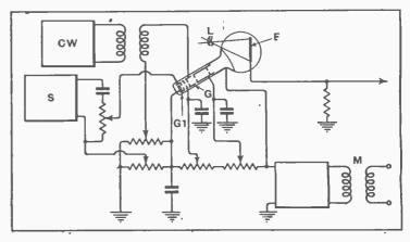
Modulating system for television transmitter using cathode-ray tube.
