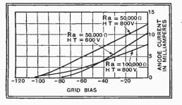
Fig. 4.-Dynamic characteristics of AC/L valve.
