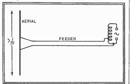
Fig. 4.—If an impedance-matched feeder is used the line may be any convenient length, but the end connections are important. Here is the usual method at the aerial end a divergent tapping of the correct dimensions. The other end is tapped the appropriate distance up the tuned circuit coil, or a variable coupling is used.
