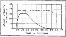
Fig. 2.—. . . reverberation causes the sound to persist after the end of the impulse from the source.
