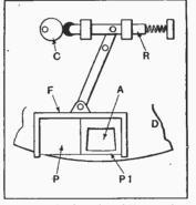
System of "interlaced " scanning using rotating disc.
