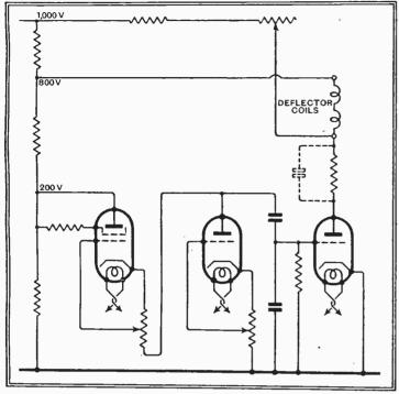
Fig. 3.--Simple magnetic scanning circuit with shift.
