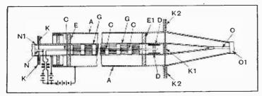
Design of valve intended for use at very high radio frequencies.
