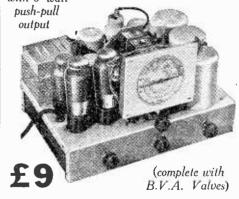
6 valve all-wave superheterodyne with similar specification, performance, etc., to above, but with large push-pull output giving  $5\frac{1}{2}$ -6 watts.
