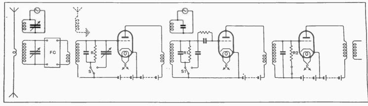
Method of receiving television and ordinary broadcast signals on a single receiver.
