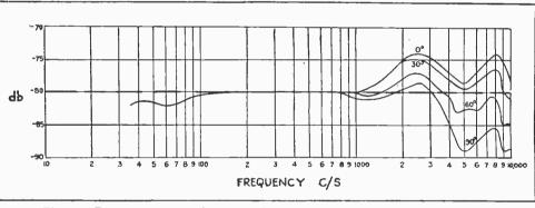
Fig. 1.--Response curves of the moving-coil microphone introduced in 1931.
