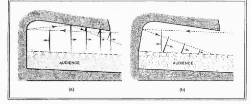
Fig. 2.—Diagrammatic sketch showing path of sound wave under the balcony of the redesigned Philips Theatre, (a) with vertical rear wall showing concentration of wave above the heads of the audience, (b) with rear wall sloping forward to direct sound downwards.
