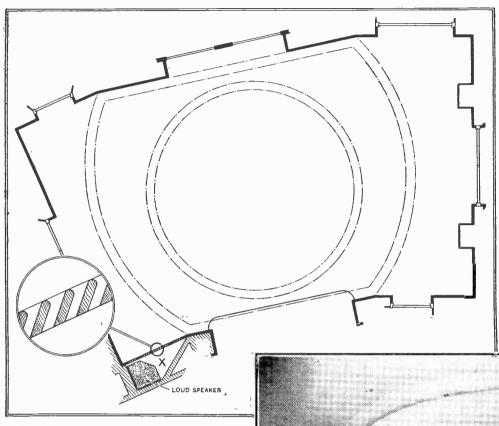
Fig. 7.-Plan of buffet showing position of concealed speaker. The arrangement of the vertical louvres in the panelling is shown in the inset.
