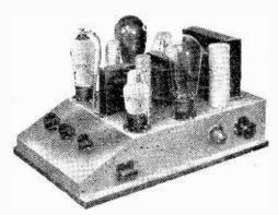
One of the constructor-type amplifiers designed by N. Partridge.
