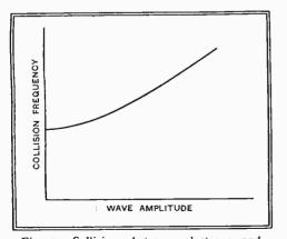
Fig. 1.—Collisions between electrons and air molecules increase in frequency when the radio-wave amplitude is increased.
