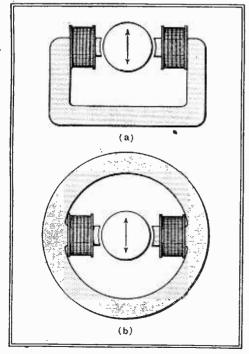
Fig. 1.—Two methods of mounting deflecting magnets on a cathode-ray tube ; the arrows indicate direction of deflection.
