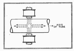
Fig. 5.—Illustrating de-focusing effect with push-pull deflection.
