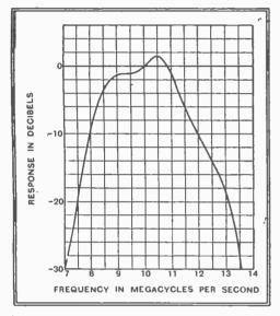
Fig. 8. The measured resonance curve of a five-stage amplifier having a gain of about 15,000 times is shown here.
