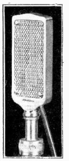
makes use of four parallel ribbons c on n e c t e d m series. It has a frequency r esponse from 50-10,000 cycles and a sensitivity of -45 db. The transformer is designed to match a 200-0hm line.
