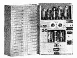
Wall-mounting amplifier made by Correx.
