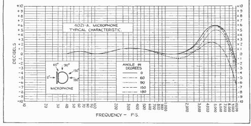
Fig. 2.-Response curves of the new directional microphone for five angles of sound incidence.
