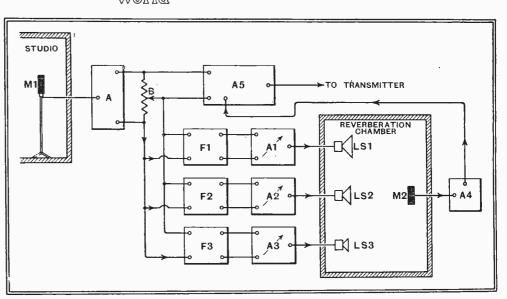
Fig. 7. General arrangement of the adjustable reverberation system of Roux-Gamzon-Sollima-Sarnette.
