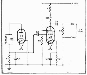
Fig. 3.—A stage of VF amplification can be used following the detector. Owing to the coupling condensers C2 and C4 the DC component is not retained.
