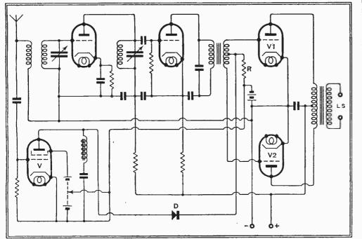
Fig. 3.—An arrangement comparable with Fig. 2, but which operates by applying a paralysing bias.
