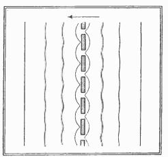
Fig. 5.—Illustrating the passage of a sound wave through cinema screen material.
