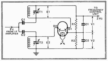
Fig. 2.—The circuit of a discriminator which provides a DC output, the polarity of which depends upon whether the intermediate frequency is too high or too low.
