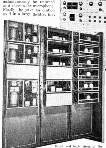
Front and Dack views of the three-circuit electrical reverberation control installed at Poste Parisien.
