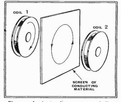
Fig. 2.—A sheet of copper or similar material acts as a shield by virtue of its high conductivity.
