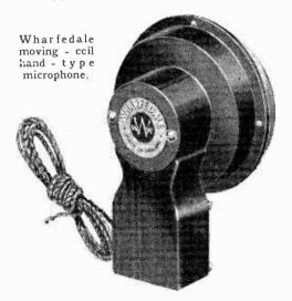
Alnico magnet and has a frequency response from 70 to 5,000 cycles. The sensitivity is -85 db., zero level being indicated by an output of 1 volt for a pressure cf 1 bar.
