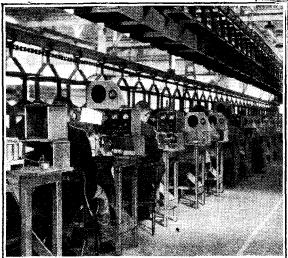
whole. Each is ensconced in a soundproof booth, which is fitted with an artificial aerial and a source of HF modulated by gramophone records on an automatic record-changer.
