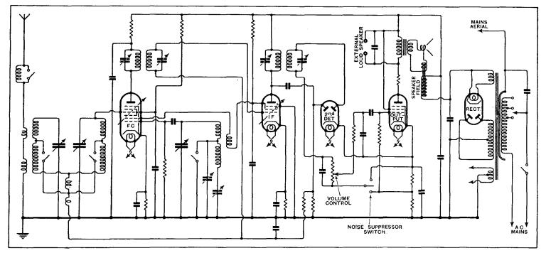
The aerial input and AVC circuits have been specially designed to give uniform sensitivity over both medium- and long-wave ranges.
