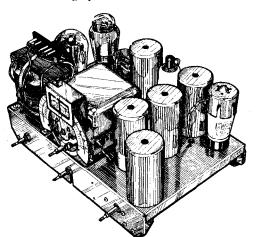
"The thoroughness of the workmanship can usually be judged by the exterior of the chassis." This drawing is of the chassis of one of the Murphy receivers.
