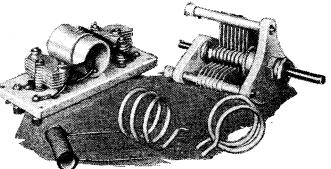
B.T.S. ultra-short-wave coils, condenser and IF unit.
