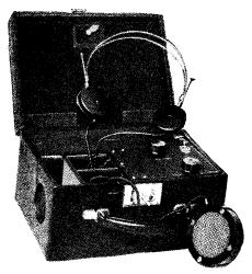
Fig. 14. Multitone Electric portable valvetype deaf-aid.
