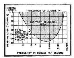
Fig. 5. Showing Fig. 1 plotted in a different manner which is suited to plotting measurements on deafness. The shaded areas are equal in both cases, as also are the vertical distances between the curves at the corresponding frequencies. Audiograms are always given in this form.
