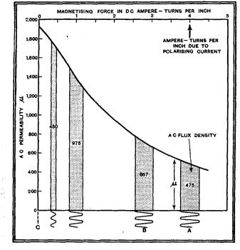
Fig. 1. Showing the fall in AC permeability when the core is polarised.
