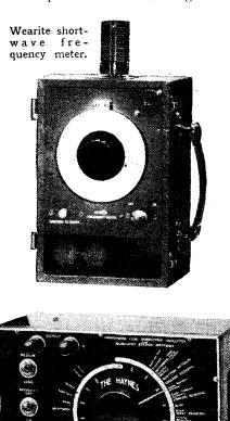
Haynes modulated oscillator for station identification.
