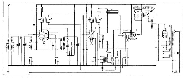
The three-valve circuit includes a combined detector-output valve, and an unusual refinement is the provision of a step-up input transformer for the pick-up.
