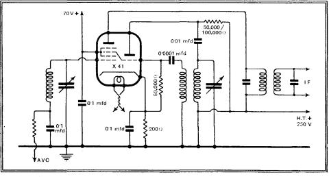
Fig. 1.—The recommended circuit connections for the triode-hexode frequency-changer are shown here. A tuned-anode oscillator circuit is advised for the best results.
