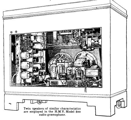
response at different parts of the room, the proximity of the walls to the back of the cabinet may also modify any cavity resonances which may be present.
