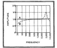
Fig. 1.—An ideal response curve compared with one having a pronounced peak as about 5,000 c.s
