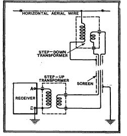
Fig. 5.—The theory of the transmission line downlead.
