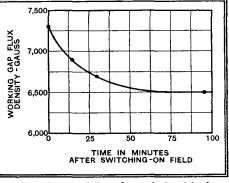
Fig. 1.—Showing time-flux relationship for energised magnet.
