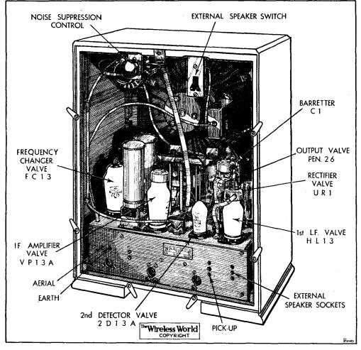
When the back of the set is removed the mains leads are automatically disconnected. Note the mains HF chokes behind the noise suppression control.
