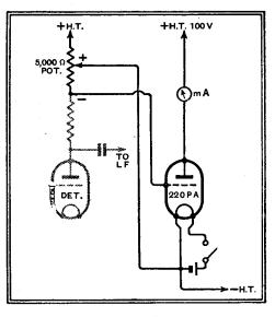
Circuit diagram of the indicator, showing connections to an existing receiver. Small voltage changes taking place in the anode circuit of a grid detector under the influence of an incoming signal are magnified, and cause easily discernible variations of the meter.
