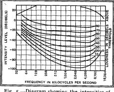
Fig. 5.—Diagram showing the intensities of sound required to give various degrees of loudness judged by a normal ear.
