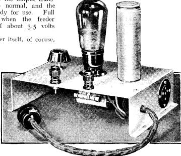
2 Ebonite shrouded terminals Belling-Lee "B" 1 4-way cable 12in., with twin 70/36 leads and 5-pin plug Goltone plug (Bulgin) Small quantity of No. 16 tinned copper wire, Sistoflex, Aluminium, etc. Screws: 1 6BA, ½in., 9 6BA, ¼in. 1 Valve Marconi or Osram MHL4
