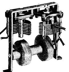
Litz-wound coils and air-spaced trimmers are used in the Eddystone 400/500 kc/s IF transformer.
