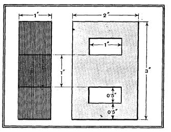
Fig. 2. Dimensions of core assumed in the worked example.
