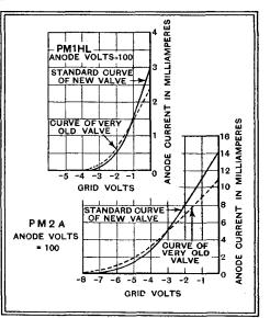
mutual conductance figure for the 1931 PMIHL was 1.4 milliampere/volt; this ancient specimen still has a mutual conductance of 0.9 mA/V. The figures for the PM 2 A are: standard of new valve 3.5; value for old valve 2.0 It will be seen from the curves that, despite their flatness, some kind of working could be obtained with the valves. I have seen many a valve in much worse shape after only a few hundred hours of use.
