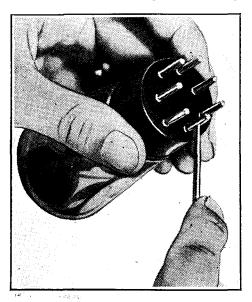
The safest way of restoring springiness to valve pins.
