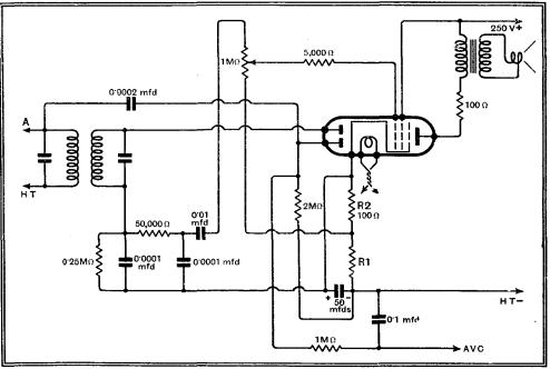
Fig. 2.—Typical connections for a duo-diode output pentode are given here. The AVC delay voltage is governed by the value of RI.
