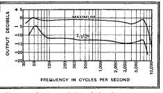
Fig. 2.—Characteristics of simple tone-compensated volume control, showing effectiveness of bass reinforcement.
