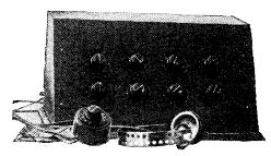
Fig. 13. Multitone Electric distributor unit for use in schools.
