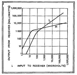
Fig. 2 .-- Outputs of low-level and high-level detector sets compared.
