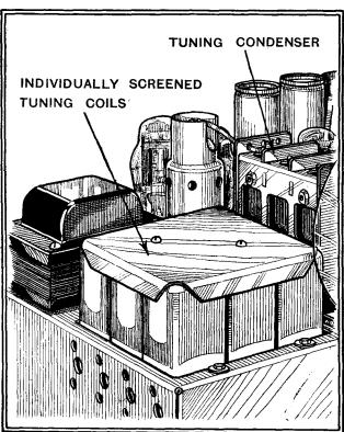
Individually screened coils are employed in this all-wave set in order to eliminate absorption spots
