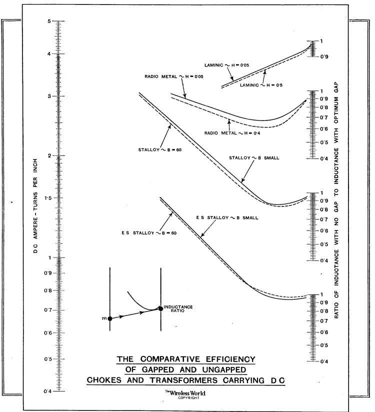
an essential figure for working out the detailed design for any specified value of inductance.
