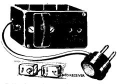
Belling-Lee radio power interference filter.
