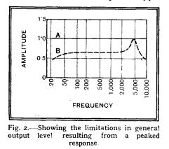
curve for, say, an intervalve transformer; it nowhere departs so far from A as to be easily distinguishable from it by ear, judging on the basis of balance of tone.
