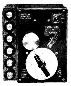
Weston modulated test oscillator.
