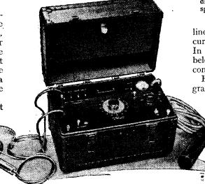
Fig. 4. The Western Electric 2B audiometer which is energised from the electric supply mains.
