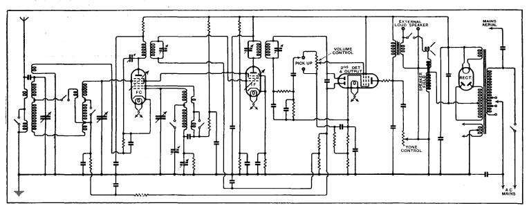
Complete circuit diagram. An image suppressor circuit is included in the input band-pass filter, which employs "mixed" coupling.
