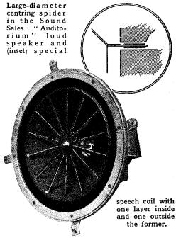
cone. This form of construction ensures that the movement of the coil and diaphragm is absolutely parallel to the axis and permits the development of large amplitudes. It also tends to keep the outer edge of the cone circular to prevent the effect known as "belling."
