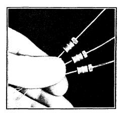
New Erie midget resistors with insulated sleeves.
