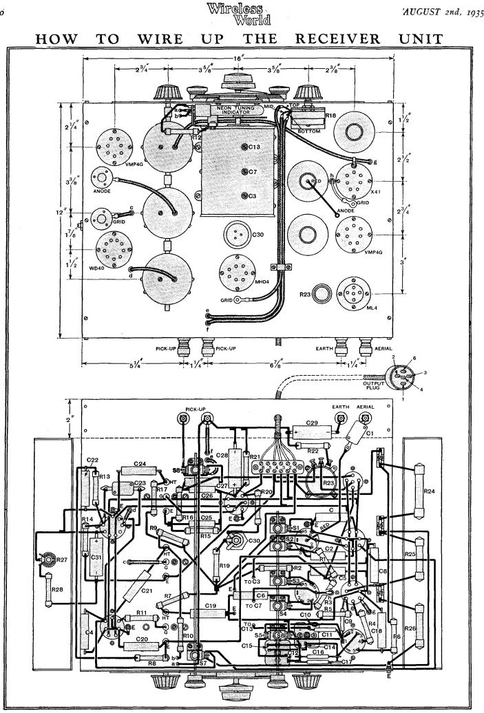
Full details of the wiring and layout of components are shown in these drawings. It is important that the layout of the wiring should be followed closely if unwanted couplings are not to be introduced.
