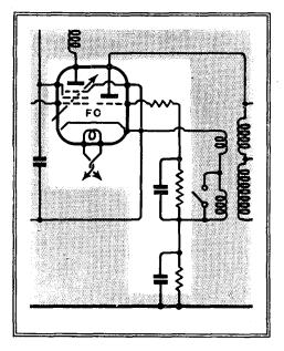
An advantage of the independent cathode; circuits of this kind are ruled out for battery valves.
