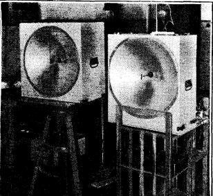
Ten-centimetre beam transmitter and receiver with reflectors.
