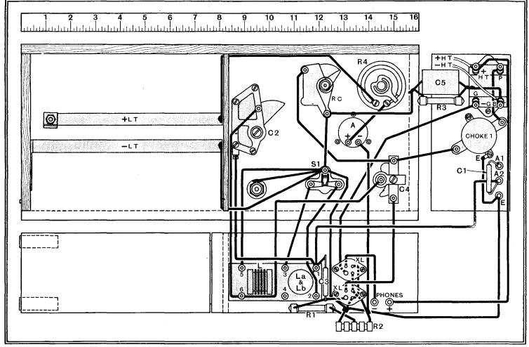
Practical wiring plan, with scale of inches for ascertaining dimensions and positions of components. Note that the bush of the slow-motion The inside back-to-front dimension of the cabinet is only  $3^{\frac{1}{16}}$  in. condenser drive knob (to the left of switch SI) is earthed. suitable for a Hartley circuit of which
