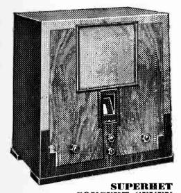
Electrically operated, for A.C. mains. Superheterodyne circuit employing variable mu valves. Seven Marconi valves (including rectifier). Delayed automatic volume control. Mush and static suppressor. Duplex tone control. Adjacent channel selectivity. Energised moving coil speaker. Optically magnified illuminated scale. Modern cabinet of finely figured woods.
