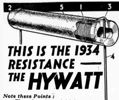
The wire element high grade iron free resistance wire (1) which is wound on a specially prepared porcelain former (2), the ends of the resistance being spot welded (3) to copper con-necting leads (4), and the whole resistance coated in "Vita" enamel (5).
