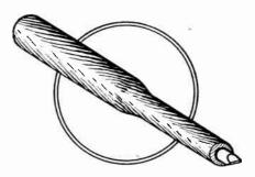
Fig. 14.—A special trimming screwdriver.
