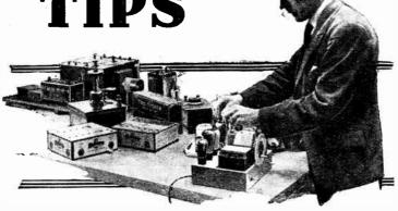
one valve is the production of violent motor-boating. Quite often, however, removal of one valve will produce motorboating, but on replacing this valve and removing the other, fairly normal working will be obtained.
