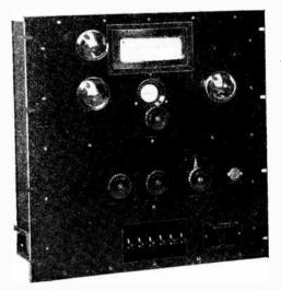
Fig. 6.—Measuring apparatus for routine maintenance tests on amplifiers and circuits.
