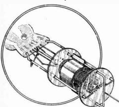
The electrode construction of a multiple diode valve for corrected A.V.C .- the Cossor D.D. Pen.
