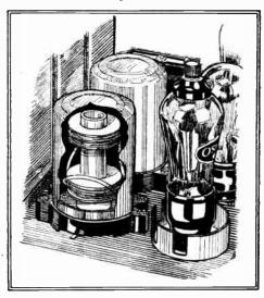
Two typical I.F. band-pass coils with adjustable coupling are shown in this illustration.
