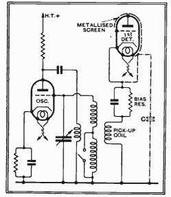
Fig. 1.—When the metallised bulb of a first detector valve is touched, signals will be weakened as a result of the added body capacity C.
