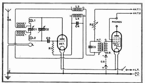
Fig. 1. The theoretical circuit diagram; values of components are:  $C_1 = 50$  mmfds. max.,  $C_3 = 0.0001$  mfd.,  $C_4$ , 0.01 mfd.,  $C_5$ , 0.001 mfd.,  $R_1 = 2$  megohms,  $R_2 = 50,000$  ohms variable.
