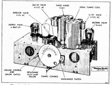
The chassis is mounted in the cabinet on rubber washers to minimise microphonic noise.
