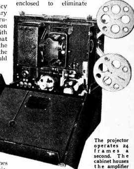
in the base noise, the volume control being brought out. The bracket carrying the feed and take-up spools also forms a rewinder, and can be accommodated inside the cabinet for transport.
