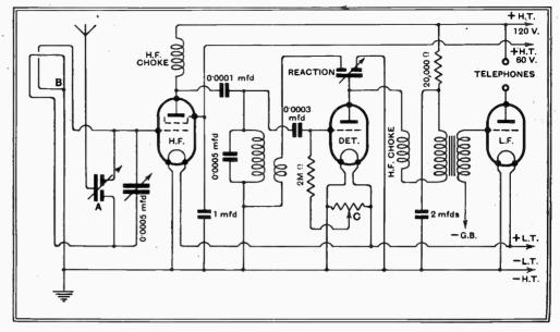
Fig. 2.—A three-valve circuit, consisting of an S.G. stage followed by a conventional detector and L.F. arrangement.
