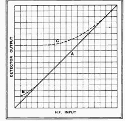
Fig. r.—Rectification characteristics (A) for a perfect detector with a single input voltage, (B) for the same detector to the stronger of two simultaneously applied voltages, and (C) to the weaker of two applied voltages. The large change in the last case should be noted.
