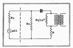
of the load in the valve anode circuit, which is the portion of the equivalent circuit to the right of the dotted line, falls to a very low value; consequently the majority of the available E.M.F. is lost in the valve resistance Rv, and the output at resonance is much less than would be the case if the E.M.F. across Ra remained constant. This explains the observed results without making the load on the secondary of the transformer a predominating factor.
