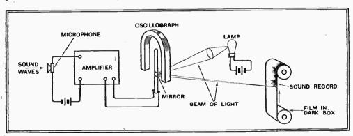
The principle of the "variable area" system of sound recording explained in diagrammatic form.
