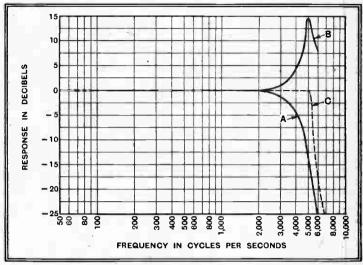
Fig. 3.—Curve A represents the effect upon quality of the sideband cutting of the receiver, while curve B shows the required shape of tone-correction curve to compensate for this.
