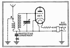
Fig. 1.—Skeleton diagram showing the need for complete isolation of the aerial-earth circuit in a D.C. set.
