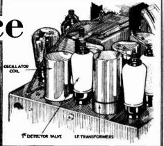
If whistles are to be avoided in a superhet with single dial control, careful choice must be made of the pre-selector circuits, the I.F. requency, and the H.F. valves. This illustration shows the essential components associated with the frequency changer.
