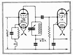
Fig. 1.—A tuned anode I.F. coupling can be used, but is not usually advisable, since the high-frequency detector output may reach the I.F. valve grid.
