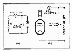
Fig. 2.—If current is normal, battery voltage must also be normal unless the resistance R in diagram (a) has undergone a change. The same reasoning may be applied to the valve circuit (b).
