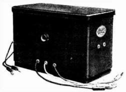
The Ferranti Class "B" converter, giving an output of about 2 watts. The L.T switch can be seen at the front of the case.
