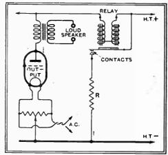
Fig. 2.—Preventing voltage rise; the artificial load resistance, R, remains connected across the H.T. supply until the valves begin to pass
