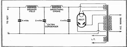
Fig. 1.--Correct positions for an extra smoothing choke and condenser.
