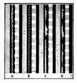
A -sound record of traffic noises; B--"Look out!"; C--brake on wheels; D--the synthetic record obtained, as explained in the article, by grafting one sound upon another.
