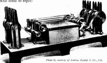
A four-film synchronous winder used for mixing sounds and applying them to "mute" pictures.
