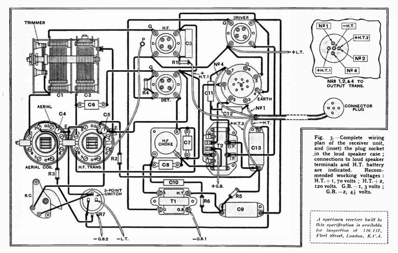
etc., the front panel must be temporarily removed, and also that the condenser should be mounted first, as it is secured in position by screws passing up through the platform; the heads of these screws will later be covered by the tuning coils. In mounting these coils, reasonable
