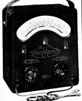
The Avoneter is the only combination testing instrument in the world that gives direct readings in Amps. Volts and Ohms willout the use of external shunts, multip'iers or transformers, and without calculations of any kind. (See Jull list of ranges above.) It is British made throughout.
