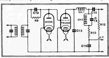
Fig. 2.—A simplified diagram showing the action of the second detector split between two valves. The tone-correction circuit in the anode of the triode should be noted.
