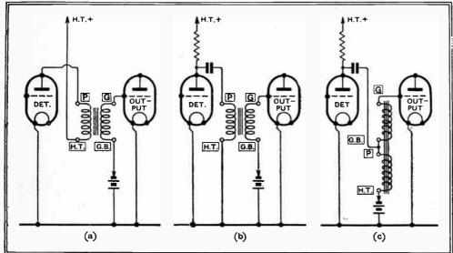
Fig. 1.-Normal transformer connections compared with those applicable in parallel-fed circuits.
