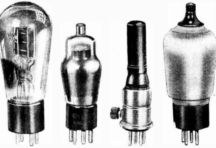
Typical new valves: (A) Mullard VP4, a variable - mu screened H.F. pentode; (B) Marconi double - diode triode, MHD4; (C) Mullard PM2B, twin Class "B" output valve; (D) Tungsram PX46 single Class "B" valve, (b) Infigstain 1 Ado single Class B valve, two of which will give 21 watts speech output; (E) Sylvania 6A7 Pentagrid; (F) Marconi Catkin pentode MPT4; (G) Tungsram SE2018 variable-mu A.C.-D.C. valve.
