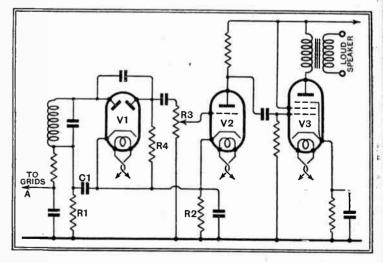
Fig. 1.—Circuit for a double-diode valve VI used for delayed A.V.C. The valve V2 is a straightforward triode L.F. amplifier coupled in the usual way to an output pentode,
