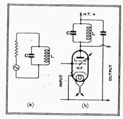
Fig. 1.—(a) The equivalent circuit of a tunedanode H.F. amplifier. The generator represents the voltages appearing in the anode circuit, and the resistance the anode A.C. valve resistance. (b) The equivalent practical tuned anode circuit.
