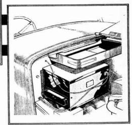
The Sparton Model 33 set fitted to a Talbot (Above) The remote control, clamped to the steering column, and (below) the receiver unit, mounted under the bonnet.
