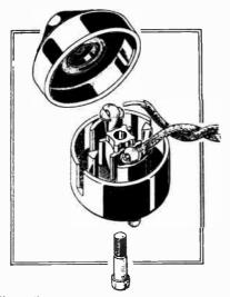
Clix wall plug fitted with self-centring pins.
