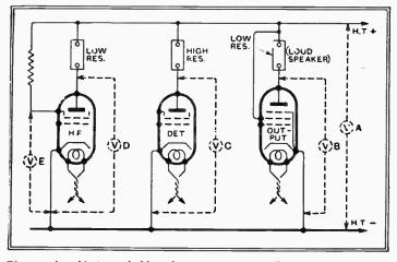
Fig. 1.-A guide to probable voltmeter errors: readings of anode voltage will be reasonably accurate where circuit resistances are low.
