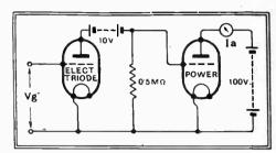
Fig. 6.—A typical amplifier circuit.
