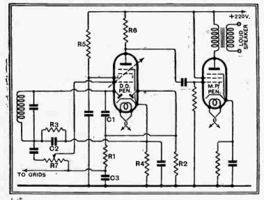
Fig. 2.—Suggested circuit for use with the new double-diode pentode. The variable-mu pentode contained within the same bulb as the double diode takes the place of the triode V2 in Fig. 1.
