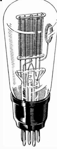
We show here a cut-away drawing of the screened Marconi triode Catkin Valve MH4 in comparison with an equivalent glass valve drawn to the same scale. Note how the grid and heater of the former are rigidly locked at both ends inside the metal anode, which, in its turn, is rubber mounted and metal-armoured, and compare this with the glass valve, with its fragile pinch, many bent wires and delicate joints.
