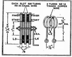
Fig. 3.—Dimensional drawing of former for coils L3 and L4, also details of small tuning coils L1 and L2.
