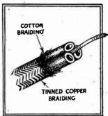
New Radiophone downlead: the conductor is centred by rubber tubes.
