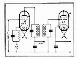
Fig. 2.—A band-pass I.F. coupling is the most satisfactory, for it gives high selectivity, and largely prevents unwanted frequencies from reaching the I.F. valve.
