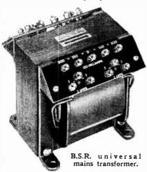
The rectifier was operated at 3.9 volts while the two 4-volt 2-amp, windings each gave 3.84 volts and the 5-amp, winding 3.89 volts. On half-load the voltages do not rise beyond the usual tolerance permitted for A.C.
