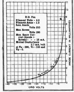
Fig. 3.—Grid volts-anode current curves of the Cossor D.D. Pen. The mutual conductance reaches the high figure of 2.7 mA.-volt.
