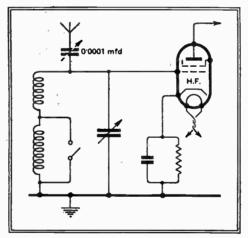
Fig. 1.—When an exceptionally short aerial is fitted, the simplest method of coupling is generally the most efficient.
