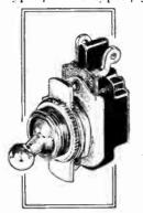
British radiophone on-off Q.M.B. switch.
