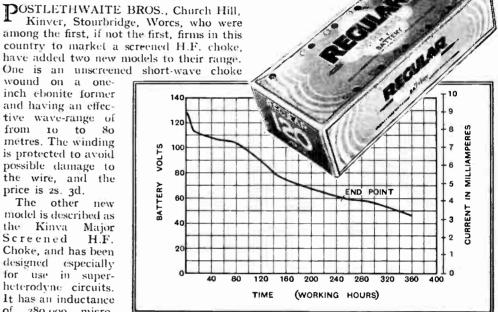
Discharge curve of "Regular" 120-volt H.T. battery.
