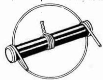
A tapped connection on a fixed resistor of the carbon type, which may in this way be converted into a potentiometer or variable resistance.
