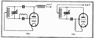
Fig. 3.—A simplification of Fig. 2 producing the well-known Hartley circuit with (a) series and (b) shunt feed.
