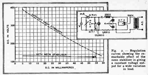
in circuit at X (see Fig. 2), which, of course, registers the total current taken by the receiver, the potentiometer for H.T. + 2 and the stabiliser. The reading remains almost steady at 60 mA., the greatest
