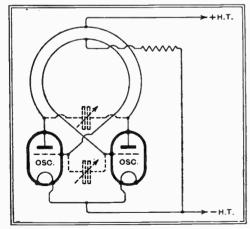
Fig. 5.—The Mesny push-pull oscillator successfully employed for wavelengths down to about three metres.
