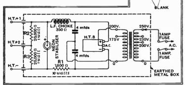
Fig. 1.—Circuit diagram. The connections of the base of the neon stabiliser are shown inset.
