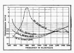
Fig. 4.—With a receiver having a highimpedance input, the arrangement shown in Fig. 2 is rather less effective.
