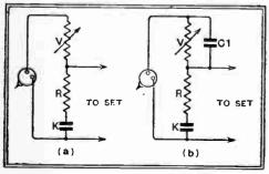
Fig. 3.—Methods of compensated volume control particularly suitable for use with pick-ups in gramophoue reproduction.
