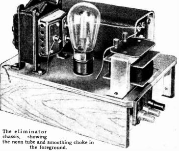
eliminator to 60 mA.—a current drain which is not likely to be reached during the peaks in any battery Class "B" receiver-a resistance R1 or 1,800 ohms must be included in the smoothing circuit.
