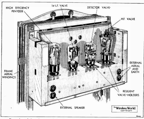
Rear view of the robust metal chassis, which can easily be removed from the cabinet.
