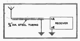
The above differs from the aerial system advocated by the G.P.O.; the use of leadsheathed wire, I find, is not so efficient at shielding as steel tubing, which does not reduce signal strength greatly.
