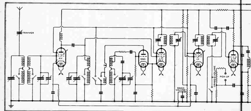
Schematic circuit diagram. Switch contacts are provided to short-circuit the loud speaker while the wave-range switch is in operation and to witch
