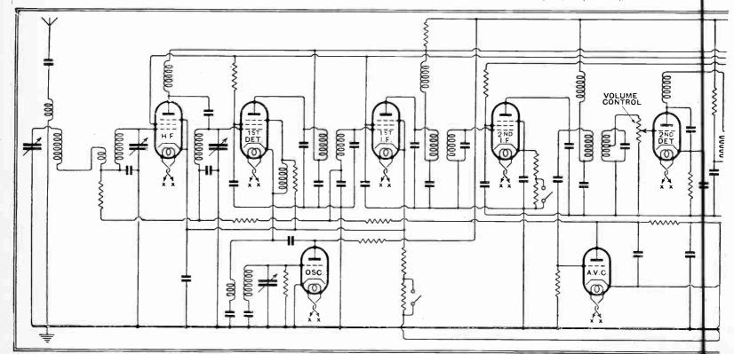
Simplifi d circuit diagram with waveband switching omitted. Tuning is facilitated by the use of a neon indicator and special interest a tacl
