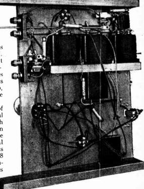
The under-baseboard, where the decoupling components and the distant - controlled switches are mounted.
