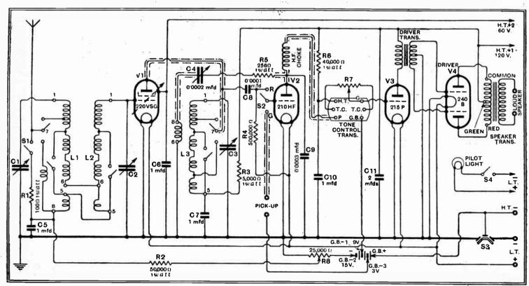
The complete circuit diagram. The switch S4 is contained within the tuning knob and connects the dial light only during the process of tuning. To prevent long leads and the risk of instability the switches S1 and S2 are distant-controlled.
