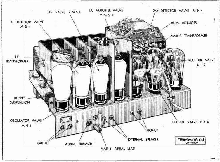
The chassis is mounted inside the cabinet on rubber shock absorbers.
