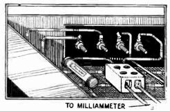
An example of the use of a porcelain connector for making a temporary addition to internal wiring.
