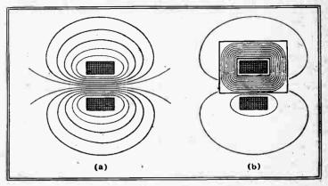
Fig. 3.—(a) The field inside a coil (seen in section) is intense, but weakens at increasing distances. (b) If the coil is provided with a closed iron core the field is restricted almost entirely to the iron.
