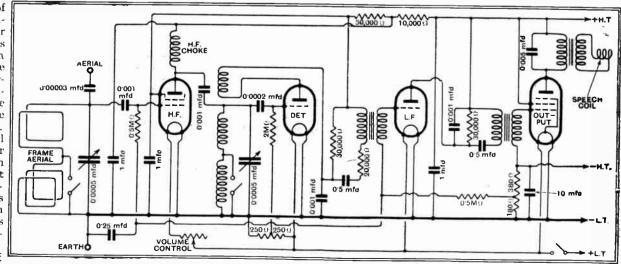
Complete circuit diagram. The anode and grid circuits are well decoupled, and there is a magnetic control of reaction.
