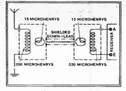
Fig. 7.—A matching circuit comparable with that of Fig. 5, but with double-wound transformers
