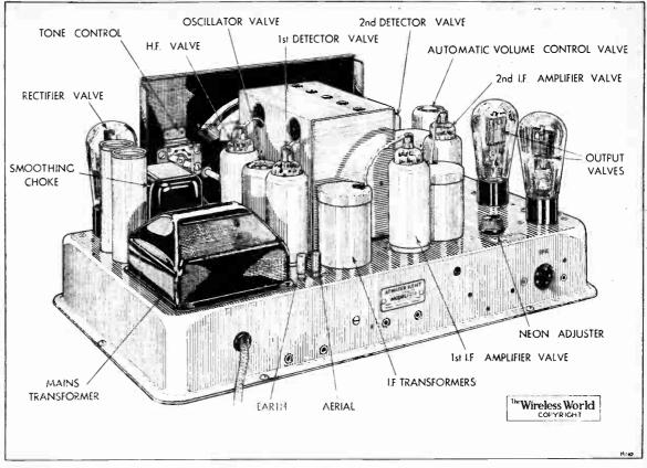
Rear view of chassis showing clean layout and accessibility of valves.
