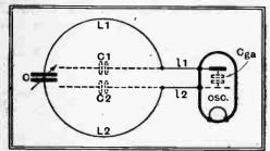
Fig. 7 (a).—The equivalent circuit of Fig. 7 with the self-capacities shown.
