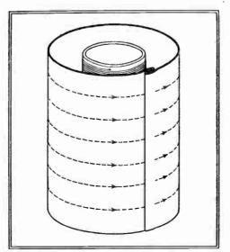
Fig. 7.—A cylindrical aluminium screen with a pressed seam may open-circuit the loop paths, owing to the high contact resistance, and so largely destroy the screening effect.
