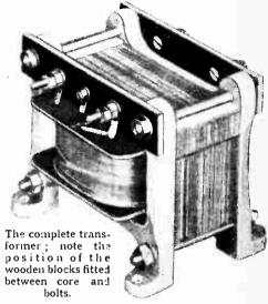
the bobbin, are put on to insulate primary from secondary.
