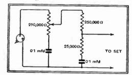
Fig. 4.—A further circuit for gramophone reproduction recommended for use with sensitive pick-ups.
