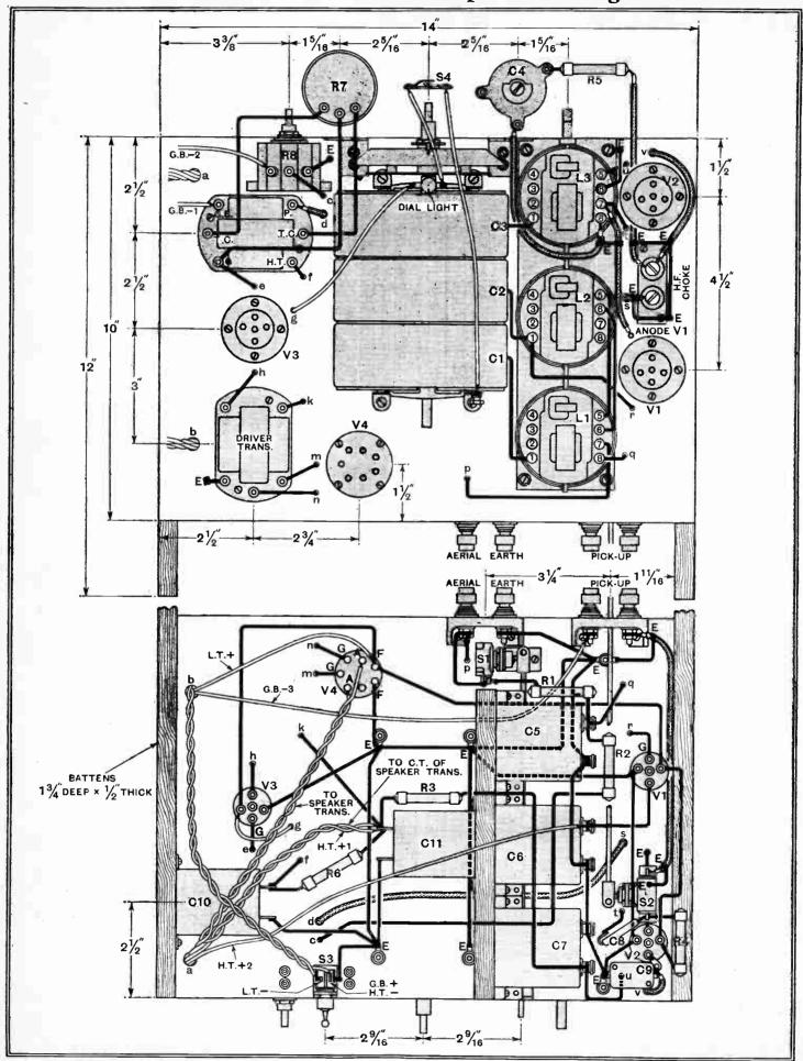
Details of the layout of components and wiring above and below the baseboard. The tone-control potentiometer and the reaction condenser, which are mounted on vertical brass strips, are here shown projected in front of the receiver.
