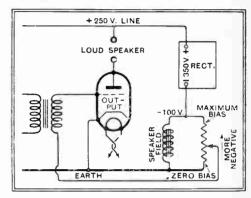
Fig. 2.—Distribution of voltages in a typical circuit where the speaker field is inserted in the H.T. negative lead. Voltages marked are with respect to the earth line.
