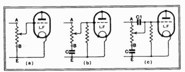
Fig. 1.—Simple circuits which provide for a compensating volume control.
