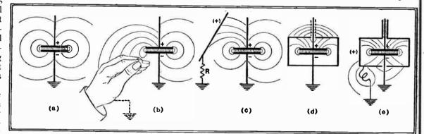
Fig. 1.—(a) The lines indicate the invisible "field" set up between the plates of a condenser when a difference of voltage exists. (b) Effect of proximity of a hand. (c) A stray lead produces a pronounced effect. (d) A condenser with a metal screen reduces stray field. (e) An inductive path from screen to earth may cause the screen to become ineffective.
