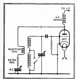
Fig. 1 .- An "anti-parasitic" device; the extra resistance, in series with the reaction coil, prevents a form of spurious oscillation which sometimes occurs at a frequency other than that to which the receiver circuits are tuned.
