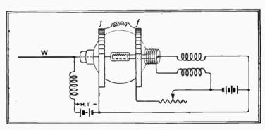
Fig. 14.—The author's "Magnetron" arrangement with which wavelengths of from 30 to 60 cms. are obtainable.
