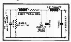
Fig. 2.—A special system of progressive smoothing is used in the "Modern A.C. Quality Amplifier." This simplified diagram of the power supply circuits shows how the parallel - connected field winding may be replaced by a loading resistance.
