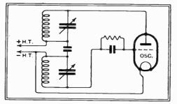
Fig. 2.—The circuit of Fig. 1 redrawn without the H.T. battery.
