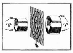
Fig. 6.—A wire gauze or mesh screen is a poor magnetic, although quite satisfactory, electric screen.
