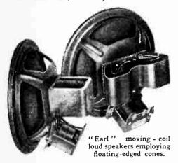
material chosen for the diaphragm, probably accounts for the absence of any sharp resonance in the higher frequencies. The output falls off gradually above 4,000 cycles, but there is still a useful response at 8,000 cycles with inputs of the order of 750 mW
