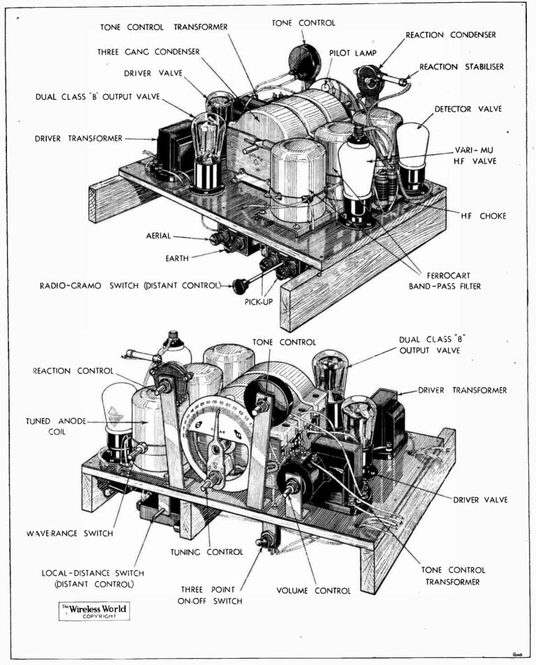
Two views of the receiver chassis. It will be seen that considerable flexibility of control is given by the inclusion of reaction, volume control, tone control, local-distance and gramo-radio switches.
