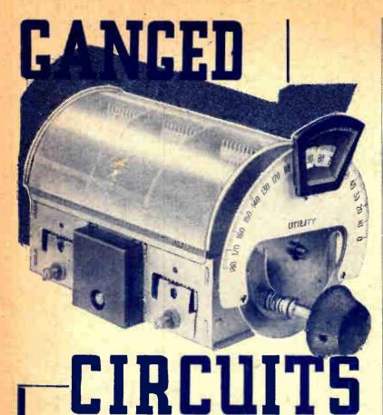
Nowadays most circuits are ganged. It is fairly easy to make accurately matched coils, but it is not as easy to make accurately ganged condensers. And disappointing hook-ups are usually due to the condensers.
