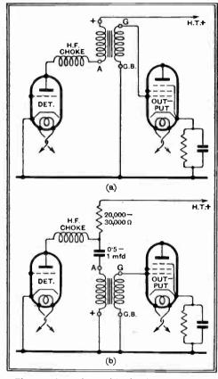
Fig. 2.—A receiver with simple transformer L.F. coupling, as in diagram (a), may almost invariably be converted to the parallel-feed system without impairing results,
