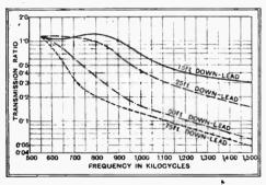
Fig. 1.—How signal strength is reduced by ordinary screened down-leads of different lengths. These curves were taken with a receiver having a low-impedance input circuit (comparable to the majority of British sets).
