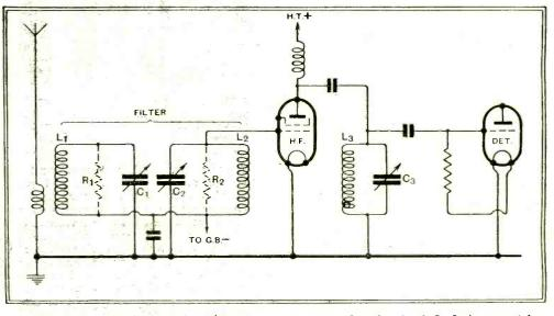
Fig. 2.—Adjusting a single-knob tuning system : to ensure that the circuit  $C_3$ ,  $L_3$  is accurately tuned to an incoming signal, the efficiency of the remaining tuned circuits may be temporarily reduced by adding parallel resistances of 5,000 ohms, or even less.
