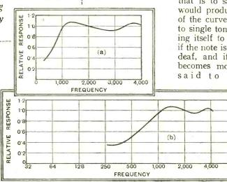
Fig. 1.—Response curves of the same loud speaker on (a) a linear frequency scale and (b) an octave or logarithmic frequency base. Curve (b) reveals that important information regarding the lower half of the musical scale is absent from curve (a).
