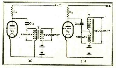
Fig. 35.—(a) Normal connection of transformer, in which primary and secondary are separate. (b) Auto-transformer connection, as used in the set, in which *bolh* windings form the secondary. The ratio is higher by one than in (a), using the same transformer.
