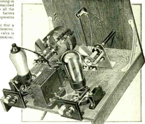
harmonics of the aerial system, but when these are particularly vicious, as is sometimes the case with certain aerials, the addition of a small coil in series with the aerial lead will overcome the trouble. A number 40 or 60 plug-in coil will prove efficacious in the majority of cases. Since the condenser just referred to serves to vary the aerial coupling, it is mounted in
