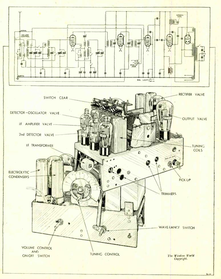
Circuit diagram and two views of the chassis-the upper showing the overhead switch gear.
