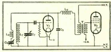
Fig. 32 .- Showing an alternative method of connecting the transformer. The steady anode current of  $V_2$  now passes through the primary, and this may be injurious to the fidelity of reproduction. the signal voltage across  $L_{\tau}C_{\tau}$ . In addition, the capacity
