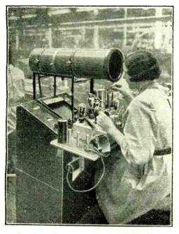
TESTING SUPERHETS BY CATHODE RAY. A photograph taken in the Ferranti Works at Hollinwood, Lancs, showing how the intermediate band-pass stage is tested by means of a special cathode ray equipment. An image of the tuning curve seen by the operative enables her to adjust the receiver accordingly.
