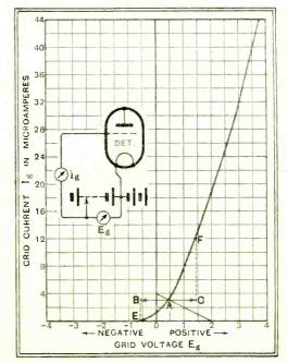
Fig. 26.—Curve showing the amount of grid current  $I_{\rm g}$  flowing for different values of grid voltage E . (Inset) A suitable circuit for measuring grid current for different values of grid voltage.
