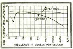
Fig. 3.—Curves showing variation in coil current when a loud speaker is used with one LS5A valve or one pentode. It is clear that there is no appreciable current variation with the pentode, which proves that the coil impedance is relatively negligible.
