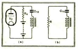
Fig. 33.—(a) The presence of  $V_2$  and  $R_1$ , in parallel, in series with  $C_{10}$  and the primary of the transformer prevent the low-frequency tuned circuit from resonating sharply; (b) shows the effective circuit,  $R_1$  and the valve resistance being amalgamated to give R.
