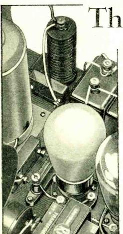
A typical modern detector stage, showing a metallised HL2 type value.
