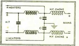
Fig. 5.—The inclusion of H.F. chokes in the mains leads removes whistles from a superheterodyne, and in some cases the connection of the local earth between condensers C gives increased efficiency.
