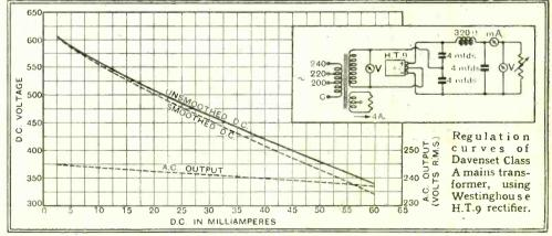
curves here reproduced show the rectified output before and after smoothing; in the one case correction has been made for the voltage dropped across the 320-ohm choke. the voltage available after From this smoothing can be calculated where chokes of different resistance are employed.
