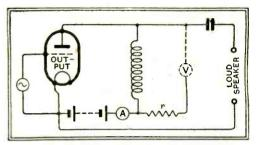
Fig. 4.—Typical output circuit including A, a milliammeter reading anode feed current, and V, a voltmeter in series with r, which is a measure of the anode feed current fluctuation. Distortion caused by anode rectification is not so unpleasant as that caused by grid current.
