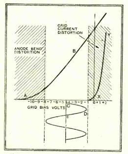
Fig. 1.—When a signal, CDE, is applied to a valve with a characteristic such as AB, the peaks must not enter the shaded danger zones of anode bend detection or grid current. A grid bias voltage of  $4\frac{1}{2}$  is seen to be necessary.
