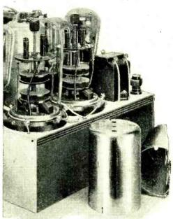
The method of coupling the coils of the intermediates is visible in this photo, where the screening covers have been removed.
