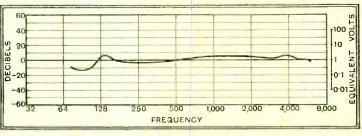
Fig. 3.—By crowding the units of the vertical scale and omitting the extreme ends, the decibel curve of Fig. 2 (b) can be made to appear substantially flat.
