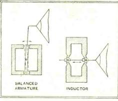
The inductor principle permits the development of larger amplitudes than the balanced armature, but is not always so sensitive.
