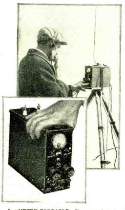
5-METRE PORTABLE. The new R.C.A.-Victor "Tranceiver," on which telephony can be transmitted or received on ultra-short waves at a moment's notice. Note the camera tripod. The weight of the instrument, including batteries, is only 22 lbs.
