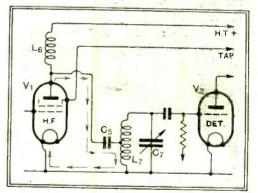
Fig. 25.—A portion of the circuit of the receiver of Fig. 9, the path of the signals round the anode circuit of  $V_1$  being marked out by arrows.
