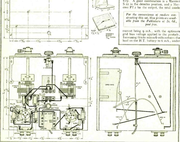
Layout of the components and the practical wiring plan, also dimensional details of condenser brackets and grid coil holder mounting. Panel drilling:  $A = \frac{7}{16}$  in. dia.;  $B = \frac{3}{8}$  in. dia.;  $C = \frac{1}{4}$  in. dia;  $D = \frac{1}{8}$  in. dia.
