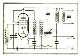
Fig. 2.—The connections of the self-neutralised pentode single - valve frequency changer used in *The Wircless World* Baby Superhets.
