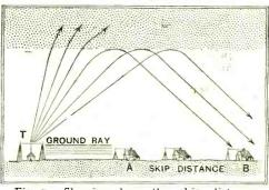
Fig. 7.—Showing how the skip distance occurs on short waves.
