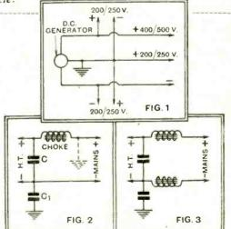
Fig. 1.—The three-phase system of D.C. mains supply, illustrating how the positive and negative earths occur. Fig. 2.—When the positive mains lead is earthed, the choke is effectively short-circuited by C and C<sub>1</sub> in series. Fig. 3.—It is usually advisable to include a choke in each mains lead, for the set is then not so greatly affected by the mains being earthed.
