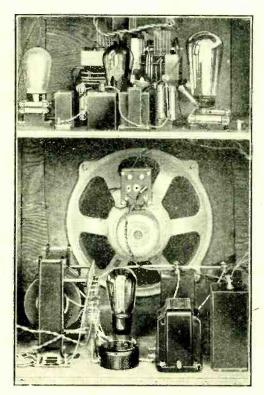
Showing the principal components of *The Wireless World* "Power Radio-Gram," the output stage of which is capable of a high volume level giving realistic reproduction.
