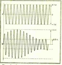
Fig: 28.—An unmodulated carrier of peak amplitude I volt is shown at (a) while represents the same carrier modulated. The amplitude now varies from 0.5 to 1.5 volts at the frequency of the note being trans-mitted.
