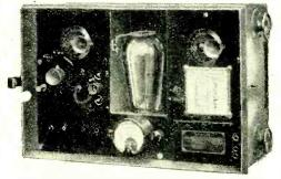
A MIDGET TRANSMITTER. A single pentode valve is used both for the generation of low power oscillations and for their subsequent amplification in this new Marconi A.D. 25A telegraph-telephone transmitter. It is fitted in the Bristol "Bulldog" fighter aircraft at the Paris Aero Show.
