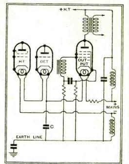
Fig. 4.—This skeleton circuit of a threevalve set illustrates the method of obtaining negative smoothing with an ordinary choke when indirectly heated valves are used.
