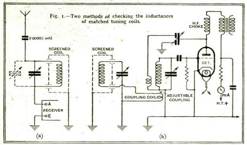
manner shown. The receiver is now accurately tuned to a transmission, and then the condenser across the test coil is adjusted so that the incoming signals are reduced to a The setting will be critical; minimum. when it has been located accurately a careful record should be made.
