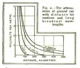
The curves apply to one kilowatt radiated where the intervening country is pastoral and sparsely wooded.
