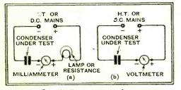
Fig. I.-Practically any type of meter can be used in testing fixed condensers, but the precaution of inserting a limiting resistance, as in diagram (a) should be observed if there is any risk of exceeding the current rating of the testing instrument.
