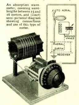
desirable to earth the rotor of the tuning condenser, as indicated by dotted lines in the diagram. When dealing with a battery set the meter will sometimes function satisfactorily when its coil is coupled to a loop formed in the earth lead. In a mains set this lead may be more or less "dead" from the "H.F." point of view, as there will be an alternative path to earth through the supply wires.
