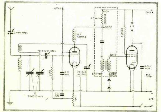
Theoretical circuit diagram of the receiver. The components enclosed by the dotted line are contained in the special L.F. coupling unit.
