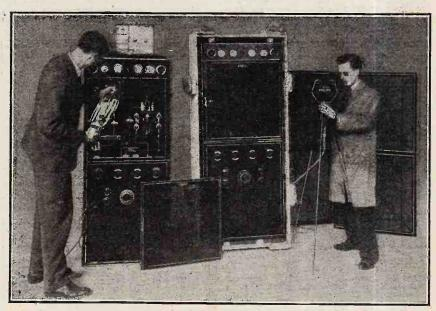
A COMPACT AMPLIFIER. Testing a Philips 500-watt amplifier which gives an output of 1½ kW. The engineer on the left is inserting a valve which takes a plate voltage of 4,000. The microphone on the right is similar to those in use at Hilversum and PCJ.
