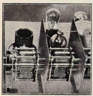
The input coupled circuit of "The Wireless World Four" which functions as an efficient pre-selector. The valve and coil screens are not shown.
