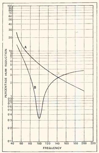
Fig. 7.—Curve A is for an ordinary choke-capacity smoothing circuit, with a choke inductance of 25 henrys, a resistance of 750 ohms, and a 2 mfd. condenser. Curve B is for a tuned smoothing circuit with the same constant as for curve A and the choke shunted by a 0.1 mfd. condenser. Note the high degree of smoothing obtained at 100 cycles.
