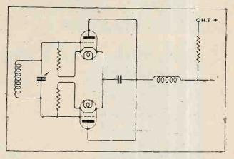
Fig. 3.—The push-pull power-grid detector. The two valves should be of the same type and preferably a matched pair. The two grid leaks should have the same value, and a resistance of 0.25 megohm or 0.5 megohm is suitable.
