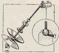
"Self-centre," fitted spindle for use on diaphragms. Weedon's adjustable
