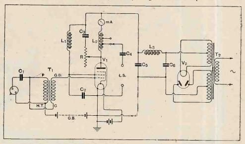
One-valve gramophone amplifier circuit on the lines of the Regional-One receiver.  $C_1$ , 0.05 mfd.;  $C_3$ , 0.01 mfd.; R, 30,000 ohms;  $C_4$  8 mfd.; G.B., 22 volts negative;  $V_1$ , PM24A and  $V_2$ , U5.
