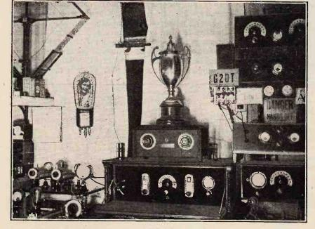
G2DT, owned and operated by Mr. E. T. Somerset at Dorking, Surrey. In the centre is the 7, 14 and 28 MC receiver with Reinartz-Grebe circuit and a screen-grid detector. On the receiver stands the frequency-monitor supporting the Wortley-Talbot challenge cup awarded by the R.S.G.B. in 1929-30 for early work on 5 metres. The transmitters comprise one for 56 MC, one TP.TG for 14 MC, and on the right is seen the 7 MC Hartley transmitter and a 28 MC 1-V-1 receiver.
