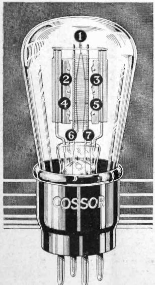
Cossor 210 DET., 2 volts, .1 amp. Impedance 13,000. Amplification Factor 15. Mutual Conductance 1.15 m.a./v. Normal working Anode Voltage 90-150. Price
