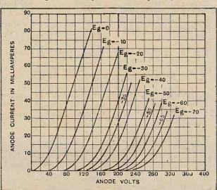
Fig. 1.—Curves connecting anode voltage and anode current in a triode. Current changes rapidly with changes in voltage. As the impedance in the anode circuit rises the voltage developed across it climbs slowly towards  $\mu$  times the voltage applied to the grid.
