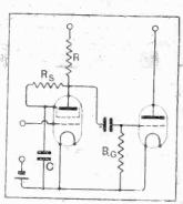
Fig. 4.—Automatic screening-grid compensation can be arranged by feeding the screen and anode through  $R_{\rm S}$  and R respectively.
