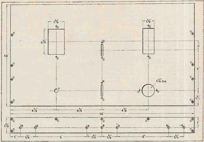
Drilling details of the front panel and the terminal strip. Sizes of holes are as follows: A, §in. dia.; B, 7/32in. dia.; C, §in. dia.; countersunk for No. 4 wood screws; D, §in. dia.
