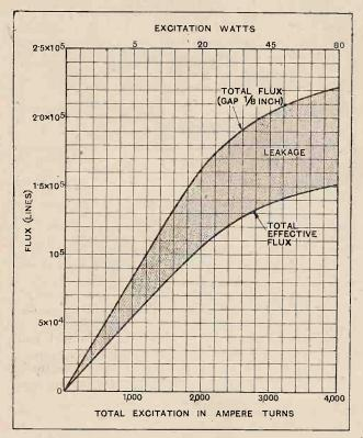
Fig. 6.—Total useful flux compared with the total flux plotted against excitation in ampere turns.
