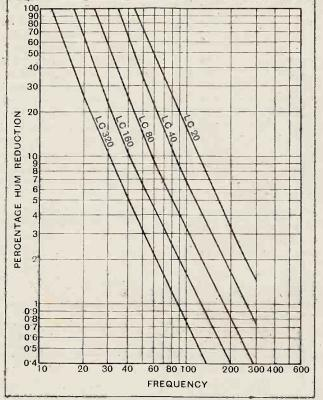
Fig. 3.—The approximate smoothing obtainable with any combination of inductance and capacity can be read off from these curves; the figures marked against each curve refer to the product of inductance in henrys and capacity in microfarads for that curve.
