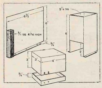
Details of the screening box for the I.F. transformer, the first S.G. valve cover and the vertical shield.
