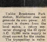
controlled by the master-oscillator system with a secondary coupling in the final power stage, which contains twelve water-cooled valves each capable of dissipating 20 kilowatts.
