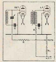
Fig. 1.--Variable "automatic" bias for an anode bend detector.
