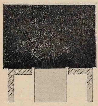
Fig. 2.—Photograph showing the external leakage and flux distribution of the magnet given in Fig. 1. The gap is in and the field distribution obtained is that which results before applying excitation.
