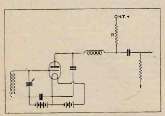
Fig. 1.—The anode detector has the merit of needing only a small anode current, and there is also little risk of hum. It does not give the best quality, however.
