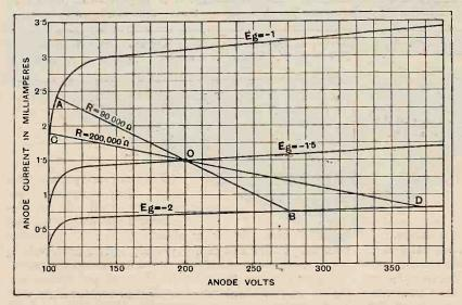
Fig. 1.—By drawing load lines across the anode volts/anode current curves of one of the latest screen grid valves it can be seen that for a given signal input, rectification and hence cross-modulation gets worse as the anode tuned circuit gets more efficient. The line AOB representing a tuned intervalve coupling of 90,000 ohms at resonance shows only slight rectification, while COD for a low-loss circuit of 200,000 ohms would give serious rectification.
