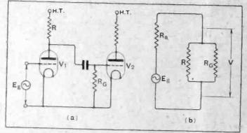
Fig. 1.—Circuit of a conventional resistance-capacity coupled L.F. stage (a). The equivalent circuit with the valve as a fictitious alternator is shown in (b).
