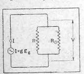
Fig. 2.—The screen-grid valve may be considered a constant current generator if the anode voltage is maintained above that on the screening grid. The amplification of a screen-grid resistance-coupled L.F. stage depends almost entirety upon mutual conductance and anode load resistance.
