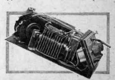
Internal arrangement of the eliminator components.
