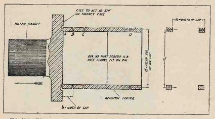
Fig. 4(a).—Diagrammatic sketch of differential search coil. The leads from the coils are flexed and brought out through the handle. They may be taken to terminals or to a switch which enables coils to be used separately or any pair connected in opposition. Greater accuracy accrues when the axial length of the coils is as small as possible. This is due to the flux density not being uniform.
