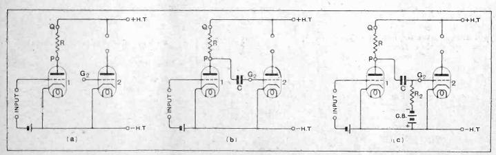
Fig. 2.—Diagrams explaining the process of coupling two valves in cascade.
