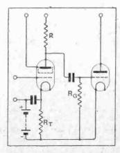
Fig. 3.—A trailing resistance R\ in association with a grid battery tends to keep the anode current constant, which in turn prevents the anode voltage from decreasing to a figure below that of the screening grid.
