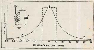
Fig. 2.—The voltage developed on the grid of the S.G. valve by Z., a station 50 kilocycles away from resonance may be sufficient to cause cross-modulation when the response curve of the input circuit is like XYZ. If the pre-H.F. volume control is adjusted until all traces of cross-modulation disappear it is possible that the voltage developed by the desired station will have become excessívely small.
