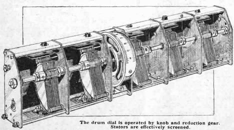
tion by means of four spacing bars running the entire length of the assembly. Easily removable shields clip over the individual sections and denser section. The plates are of brass and are shaped to follow a logarithmic tuning scale. Pigtail earthing is fitted to the centre shaft.
