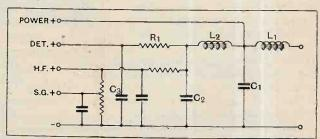
Fig. 2.—A series proportional smoothing circuit; with high amplification  $\mathbf{R}_1\mathbf{C}_3$  must be large to avoid feed-back, but if push-pull be used  $\mathbf{R}_1$  and  $\mathbf{C}_3$  can be omitted.
