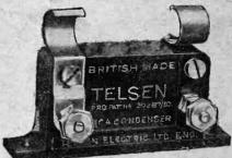
TELSEN FIXED (MICA) CONDENSERS. Shrouded in Genuine Bakelite, made in capacities up to 'oo2 mfd. Pro. Pat. No. 20287/30. '0003 supplied complete with Patent Grid Leak Clips to facilitate series or parallel connection. Can be mounted upright or flat. Tested on 500 volts. Price 1/- each.
