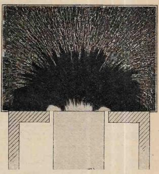
Fig. 3.-External leakage flux distribution with full excitation.
