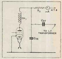
Fig. 1.—The "Band-Pass Four": correct position for a detector anode milliammeter.
