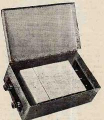
Interior of special anti-interference unit designed for use with M-L. machines Types H.E.A., L.E.A., H.F.A. and L.F.A.
