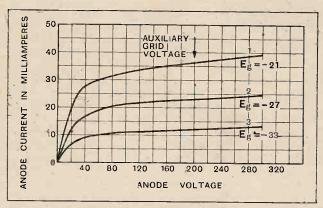
Fig. 2.—Curves connecting anode voltage and anode current in a pentode. The current changes very slowly with changes in voltage within the working range (nearly horizontal part of the curve). The voltage developed across a variable impedance in the anode circuit is nearly proportional to the value of the impedance; in other words, the A.C. current is nearly constant.
