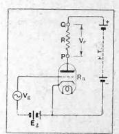
Fig. 1.—When a non-inductive resistance R is connected in the anode circuit of a valve, the theoretical value of the voltage amplification obtained is  $\mu$   $\frac{R}{R+R_{\rm h}}$  where  $\mu$  is the amplification factor of the valve and  $R_{\rm a}$  is its A.C. resistance.
