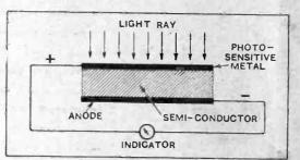
Diagrammatic representation of Herr B. Lange's photo-electric cell, for which enormous advantages are claimed.
