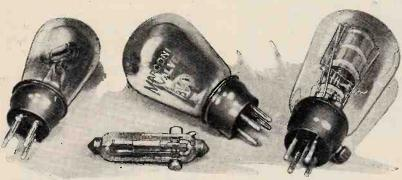
The Marconi-Osram QX, seen in the foreground, was one of the earliest special detector valves designed for anode rectification, and is shown in contrast with the Mazda A.C./Pen., a recently developed valve suitable for super power-grid detection. The DER and DESB valves, also shown in the illustration, were other very popular types used for rectification.
