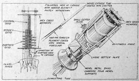
Showing the disposition of the three grids (left). On the right is seen the multipleelectrode structure firmly boited to the glass pinch. Two getter plates ensure a perfect vacuum.
