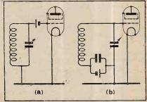
Fig. 2.-Methods of biasing an H.F. valve.
