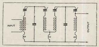
Fig. 3.—Will it come to this? A pre-selection band-pass filter with four ganged condensers. The mixed capacity and inductive coupling ensure a constant rectangular resonance curve over the waveband.
