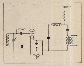
Fig. 2.—The correct grid potential is important with battery-type valves; this can be adjusted by the potentiometer P, which should have a resistance of some 400 ohms. If the grid be insufficiently positive distortion will occur, but if it be too positive the tuned circuit will be highly damped.
