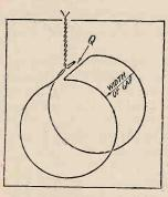
Fig. 4(b).—Alternative form of single turn differential coit. The space Q is left merely to show the construction of the coil.
