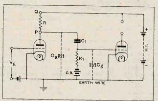
Fig. 1.—Resistance-capacity coupling of two valves in cascade. The imaginary condensers  $C_a$  and  $C_g$  represent the inter-electrode capacities of the valves as they affect the circuit at high frequencies.
