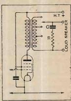
Fig. 5. — An equivalent circuit to that of Fig. 4, using a multi-ratio transformer in place of a tapped choke.
