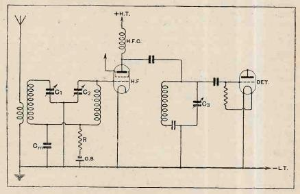
Fig. 3.—Arrangement of grid circuit components which allows a triple-ganged condenser to be used in a battery-operated receiver.
