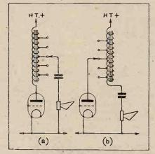
Fig. 1.—A tapped choke may be arranged as (a) a step-down or (b) a step-up coup-ling between the output valve and the loud speaker.
