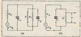
Fig. 3.—A.C. circuits equivalent to the intervalve circuit of Fig. 1 at high frequencies, showing the effect of the internal valve capacities. In (b) C! stands for  $C_n$  and  $C_n$  in parallel and  $R^i$  for R and  $R^i$  in parallel.
