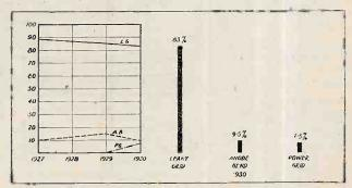
The introduction of power grid detection has checked the rise in popularity of the anode bend detector.
