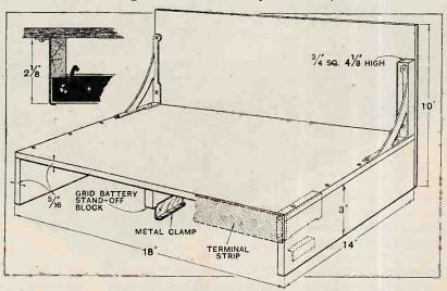
Details of the wooden frame giving the principal dimensions; note the supports on the underside for the large grid battery.
