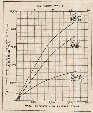
Fig. 7:—The effective flux density obtained in the air gap plotted against the excitation in ampere turns showing how the flux density varies with reduction in the length of the gap.
