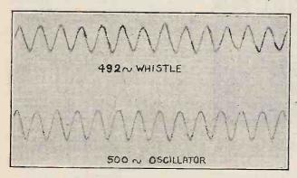
Oscillogram showing frequency and wave form of lowest whistled note obtained by G. A. V. Sowter, R.Sc., A.M.I.E.E.
