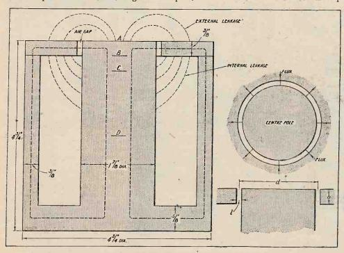
Fig. 1.—Dimensional drawing of a typical electromagnet such as was used for the measurement of flux density.
