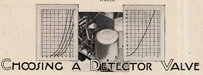
A Comparison of Anode and Grid=circuit Rectification.
