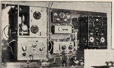
Compactness is a noticeable feature of the wireless gear on the Dornier X flying boat. The apparatus was made by the German firm of C. Lorenz.
