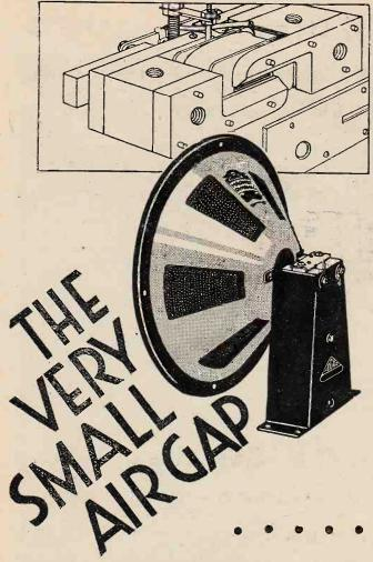
HE special design of the magnet system in the new , Hegra Magnet-Dynamic Speaker, enables a very small uniform air gap to be employed. This, together with pole shoes specially shaped to give a compensated field, ensures uniformity of armature response. At the same time, it is impossible for the armature to come into contact with the pole-pieces.
