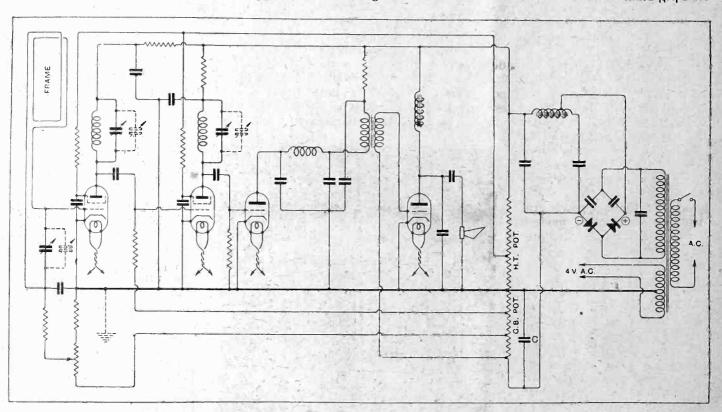
Circuit diagram, simplified by omission of certain features discussed in the text. An electrolytic condenser (C) is used for smoothing the blas voltage supply.
