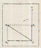
Fig. 4. — Rotating vectors showing the phase relationships of the currents in the circuit of Fig. 3 (b).
