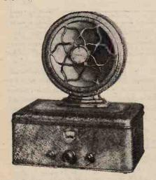
Crosley 26 H. receiver. A battery-operated set with three screen-grid H.F. valves and push-pull output.
