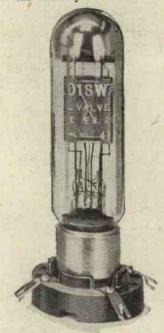
Ediswan super-power valve, type E.S. 75. The maximum anode voltage is 1,250, and the maximum anode dissipation 75 watts.
