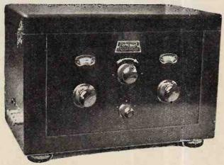
Pericaud E3 receiver with single screened H.F. stage and variometer plate coupling.
