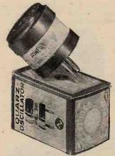
Libewe quartz crystal oscillator for trans-mitter control, or calibration and occa-sional check of a wavemeter.
