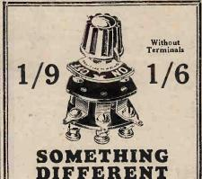
HERE is the switch for which every con-structor has been waiting. The Bakelite pointer knob is affixed to the spindle by a set screw in a brass bush. The spindle itself carries an insulated arm at the end of which is a spring loaded ball contact.
