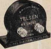
Telsen H.F. Chokes, designed to cover the whole wave-band range from 18 to 4,000 metres, extremely low self-capacity, shrouded in Genuine Bakelite. Inductance 150,000 microhenrys, resistance 400 ohms. Price 2/6 each.
