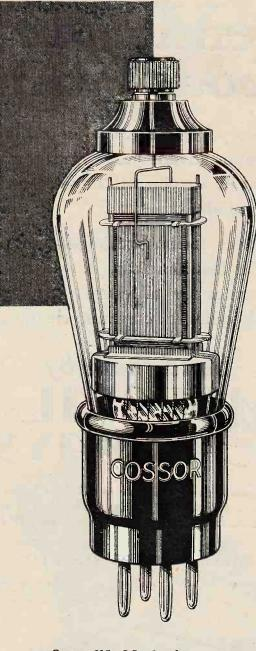
Cossor 215 S.G. 2 volts, '15 amp. Impedance 300,000. Amplification Factor 330. Mutual Conductance 11 m.a/v. Normal working Anode Volts 120. Positive Voltage on Screen 60-80. Price 20/-
