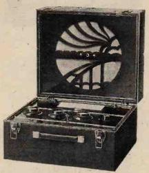
H.S.P. portable, with three separately tuned circuits.
