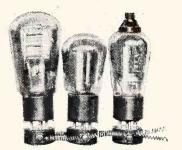
A trio of Six-Sixty valves: power output, general purpose and screen grid types.
