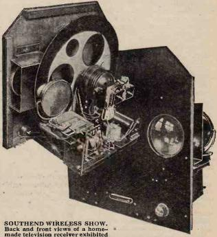
Back and front views of a homemade television receiver exhibited by Mr. A. Knipe. It is fitted with the standard arrangement of toothed wheel synchronisation. The cathode of the neon lamp glows on both sides, a concave mirror being provided to bring the light emitted from the reverse of the electrode to the scanning disc.
