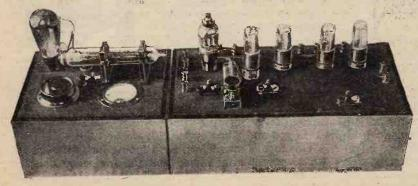
The new Lucas-Sullivan quartz frequency standardising apparatus (H. W. Sullivan, Ltd.), for frequencies between 50 and 3,000 k.c.
