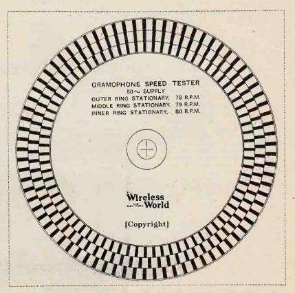
Paste the gramophone tester on to a piece of stiff card and carefully cut round the circumference. Punch a hole at the centre just large enough to admit the gramophone spindle. When placed on the revolving turntable and viewed by the light of a neon lamp connected to a 50 cycle A.C. supply the ring appearing stationary will indicate the running speed.
