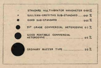
Fig. 1.—The relative inaccuracies of various types of wavemeter • are shown proportional to the areas of the circles.
