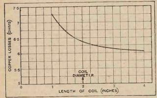
Fig. 1.—Relation between copper losses and length of coll. The inductance is 250 microhenrys and the diameter 2in.
