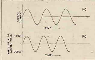
Fig. 2.—(a) Represents the A.C. current flowing through the windings of the electromagnet of Fig. 1: (b) represents the resulting frequency variations in the carrier wave.
