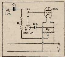
Fig. 1.—Gramophone pick-up connections for "The Wireless World" Kit Set.
