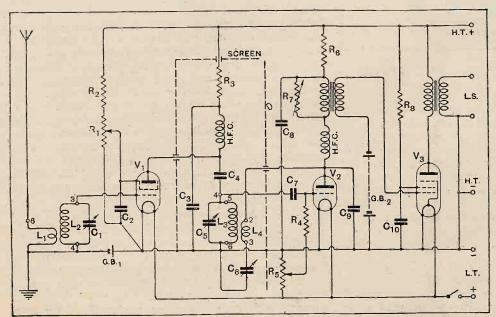
Fig. 1.—The theoretical circuit values are as follows:  $C_1$  and  $C_5=0.00015$  mfd.,  $C_2$  and  $C_3=0.01$  mfd.,  $C_4$  and  $C_9=0.0002$  mfd.,  $C_5=0.00075$  mfd.,  $C_8=2$  mfds.,  $C_{10}=1$  mfd.,  $R_1=30,000$  ohms,  $R_2$ ,  $R_3$  and  $R_6=20,000$  ohms,  $R_4=5$  megohms,  $R_5=Polar$  semi-fixed potentiometer,  $R_7=200,000$  ohms,  $R_8=5,000$  ohms.
