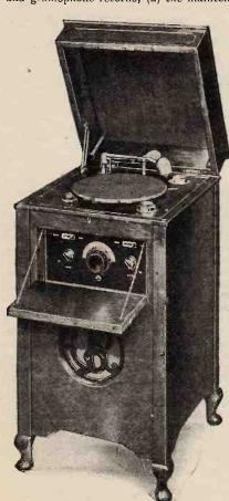
General view of the Clarith radio-gramophone, showing simplified control panel and moving coil loud speaker grille.
