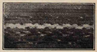
Fig. 8.—Microphotograph showing wear of record groove caused by badly worn needle.
