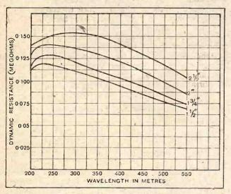
Fig. 3.—Dynamic resistance of typical tuned circuit incorporating 200-microhenry colls.
