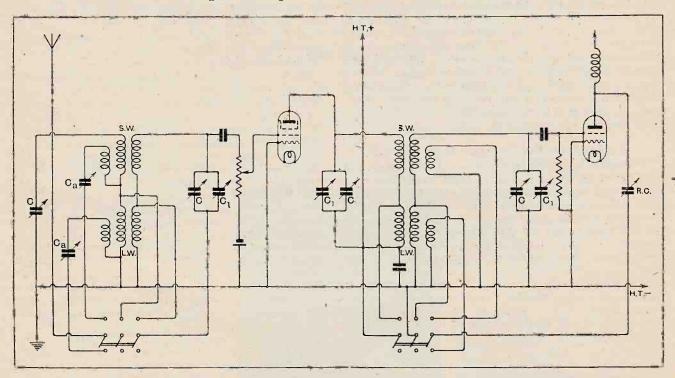
Fig. 7.—Circuit showing ganged filters, equalising condensers and a suggested method of waveband switching. C, ganged tuning condensers 0.00035 mfd.:  $C_1$ , equalising condensers of 50 mmfd. and  $C_2$ , series aerial condensers.
