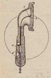
Internal construction showing (a) Contacting plate. (b) Diaphragm. (c) Flexible lead. (d) Shunt resistance.
