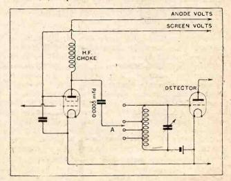
Fig. 4.—Tuned grid H.F. coupling, using tapped coil. By connecting the lead A to different tappings, selectivity, amplification and stability can be varied until the best compromise is found.
