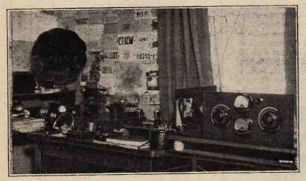
A COMPACT STATION.—G 2BY owned by Mr. H. C. Whatley at 37, Paddenswick Road, Hammersmith, W.6. The input is 10 watts in a T.P.-T.G. circuit. The H.T. supply is 400 volts maximum from an M-L rotary converter driven from accumulators.
