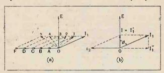
Fig. 4.—(a) Vector diagram showing that the resultant current is least when in phase with the voltage. (b) Vector diagram for parallel circuit tuned to resonance.
