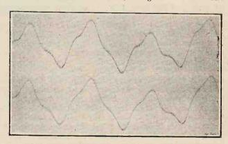
Fig. 5.—Curves showing the movement of the pick-up armature with a new needle (upper curve) and a worn needle (lower curve).
