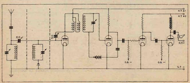
Fig. 2,-A "Wireless World Diary" circuit with two low-gain L.F. stages, modified by the addition of an H.F. amplifying valve.
