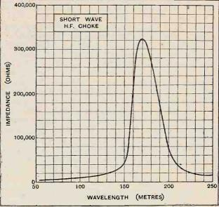
Fig. 2.—Impedence curve of a typical short-wave H.F. choke with a shunt capacity of 8  $\mu\mu$ F.
