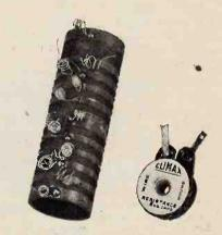
Climax 20,000-ohm wire-wound potential divider and 600-ohm decoupling resistance.
