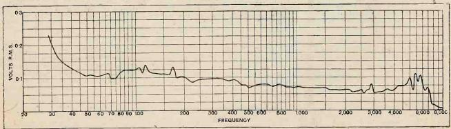
Output characteristic of the Burndept needle armature pick-up taken with Columbia De Luxe needle and 10,000 ohms shunt resistance.
