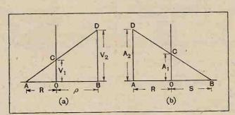
Fig. 2a.—Extended range  $V_2$  of voltmeter may be increased by the use of the larger series resistance  $\rho$ . Fig. 2b.—Extended range  $A_2$  of voltmeter may be increased by diminishing the value of the shunt resistance S.
