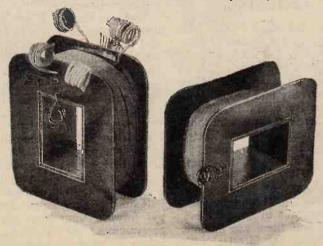
The two bobbins; one finished, the other only partly wound. Note the method of finishing off the thick wire coils.
