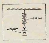
Fig. 4.—Weight and spring arrangement for illustrating electrical oscillations in a tuned circuit.
