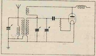
Fig. 1 .- A filter circuit preceding a leaky-grid detector.
