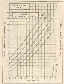
Average values under working conditions: A.C. resistance, 4,450 ohms; amplification factor, 5.5; mutual conductance, 1.2 mA/volt.
