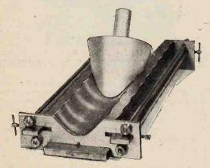
Fig. 4.—New needle the end of which has been devised to fit snugly into an 8,000 cycle groove, resting against the contours of a 4,000 cycle groove.
