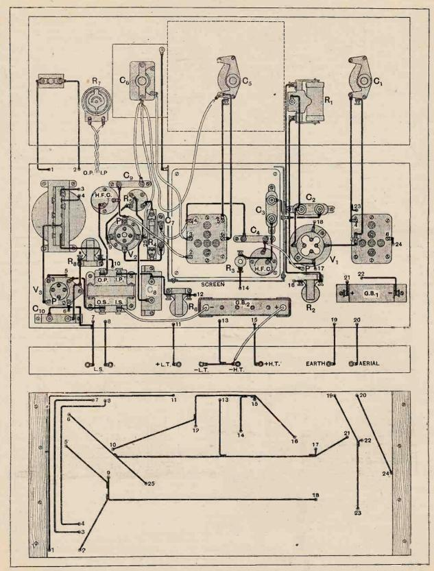
Fig. 7.—Practical wiring plan. Wires passing through the baseboard are lettered to facilitate tracing their path as shown on the under-deck plan.
