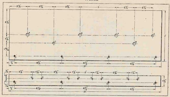
Fig. 5.—Dimensional data of panel and terminal strip. Sizes of holes are as follows: A = 7/16in. dia., B = 3/8in. dia., C = 5/16in. dia., D = 5/32in. dia., E = 1/8in. dia., countersunk for No. 4 wood screws.
