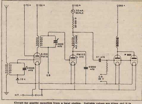
Circuit for quality reception from a local station. Suitable values are given and it is assumed that when operated from an eliminator the voltage regulating resistances will be arranged to avoid interstage coupling.
