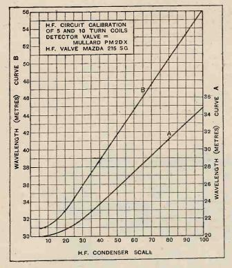
Fig. 8.—Calibration curves of the H.F. coil with reaction adjusted to cause the stage to oscilitate weakly.
