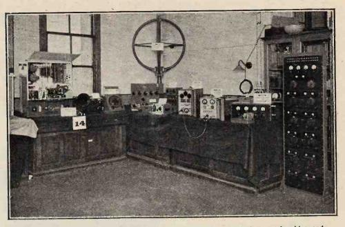
A general view of the Marconi exhibit. On the extreme left is a telephone set for ships, and next to it a marine receiver with a wavelength range of from 15 to 20,000 metres. In the corner is the fixed frame aerial used with the direction-finder seen on the right of the left-hand bench.
