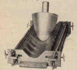
Fig. 6.—Badly worn needle riding on top of the groove walls. This gives rise to a scraping noise while the needle tip is free to wobble in the groove.
