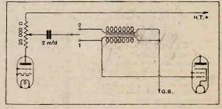
Switch in position (1) gives resistance coupling. As the resistance is only 25,000 ohms the output from the detector does not overload the pentode and no further volume control is needed. The high inductance of the transformer secondary is used instead of a grid leak. This coupling is used for the more powerful
