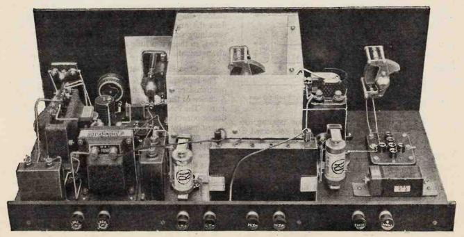
Rear view of set with coils and valves removed.
