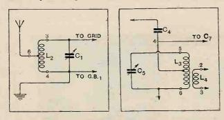
Fig. 3.—Theoretical connections of the aerial grid coil (a) and tuned grid H.F. coil (b) for use on the medium broadcast waveband.
