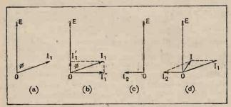
Fig. 2.—(a) and (b) vector diagrams for inductive branch of Fig. 1. (c) for condenser branch and (d) for the complete circuit.
