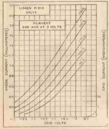
Average values under working conditions: A.C. resistance 50,000 ohms; amplification factor, 25; mutual conductance, 0.5 mA/volt.
