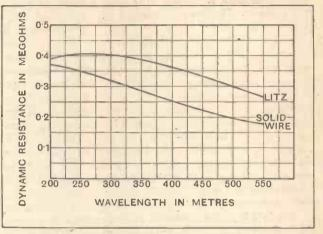
Fig. 3.—Dynamic resistance of tuned circuit with condenser and decapped valve in parallel with the coll.
