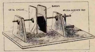
Layout of the coil winder mentioned in the text. Metal end plates are required to hold the bobbin and prevent bulging.
