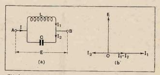
Fig. 2.—(a) Parallel circuit assumed to possess no resistance. (b) Vectors showing the phase relationships of the three currents I,  $I_1$  and  $I_2$ .
