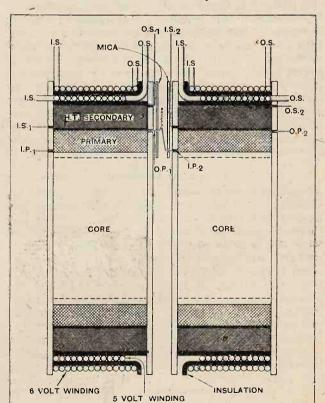
Sectioned drawings of the two bobbins showing the disposition of
