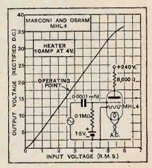
The distortionless curve of the MHL4 valve used as a "power" detector working on the leaky-grid principle. The circuit constants are given. The anode current is 14 mA. and the change in current on tuning in the signal is 2 mA for optimum rectification.
