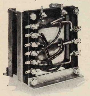
This view of the finished transformer shows clearly the manner in which the terminal battens are attached to the holding-down bolts.
