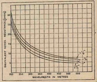
Fig. 2.—Equivalent series resistance of complete tuned circuit embodying 200-microhenry coils.
