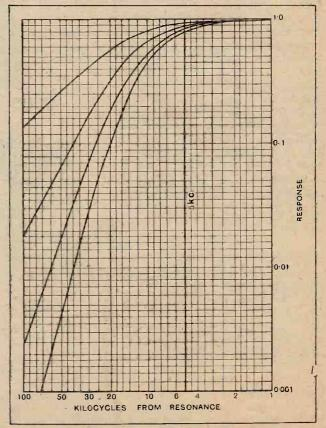
Fig. 6.—Resonance curves of 1, 2, 3 and 4 tuned circuits, using 2in. coil at 225 metres.
