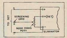
Fig. 1.—Critical adjustment of climinator output voltage is obtained by adding an external high-resistance potentiometer.
