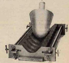
Fig. 2.—Large scale model of a steel needle moving in the groove on the record. The furrows represent a note of 4,000 cycles per second.
