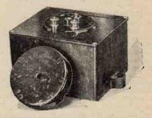
Dubilier anti-interference unit Type BRI, an absorption rejector designed to reduce interference from 2LO.
