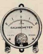
A useful laboratory instrument. A new moving coil calibrated pointer galvanometer, shown by Messrs. Crompton Parkinson, Ltd., with centratero and giving full scale deflection at 2 mA. and 80 mV.
