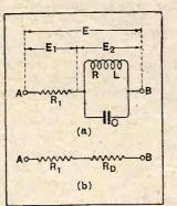
Fig. 3.—(a) Tuned circuit in series with a fixed resistance. (b) Equivalent circuit at the resonant frequency;  $R_D = \frac{L}{CR} \text{ ohms.}$
