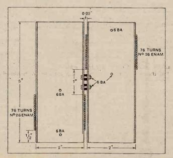
Fig. 6.—Dimensions of medium-wave colls which have proved successful in band pass filters. The inductance of each coil is 240 microhenries.
