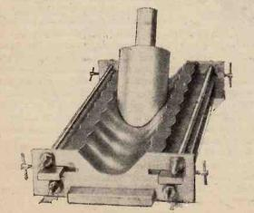
Fig. 7.—Worn Tungstyle needle where the width of the groove is greater than the diameter of the needle.
