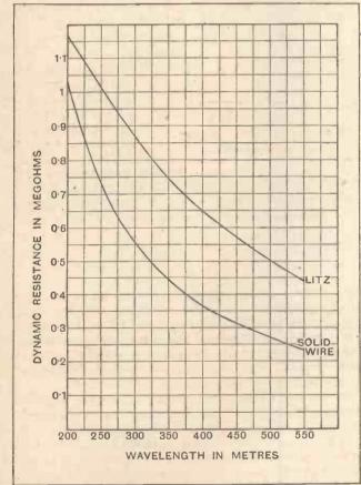
Fig. 2.—Theoretical dynamic resistance of tuned circuit, taking only the copper losses of the coil into consideration.
