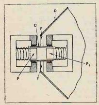
Fig. 2.—A moving coll with two pot magnets so arranged that the electrodynamic effects are additive. (No. 312,950.)
