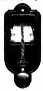
The Igranic drum condenser control with illuminating lamp behind the aperture.
