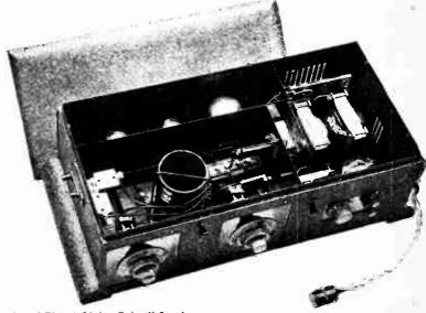
Interior of Ekco "Mains Drive" 3-valve receiver.
