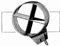
Short wave coil by Messrs. D.X. Coils, Ltd.
