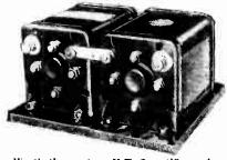
Westinghouse type H.T. 2 rectifier unit : output 0.1 amp. at 350 volts for supplying anode current to L.S.5.A valves.
