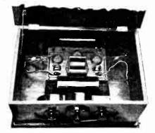
Interior of Brownie Dominion Three with valves and batteries removed.
