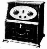
An example of advanced set design: the Pye 3-valve receiver with screened-grid high-frequency and pentode output valve.
