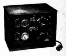
Exide combined H.T. and L.T. trickle charger with meters for checking charging rates. By means of a special switch the mains are never connected to the receiver.
