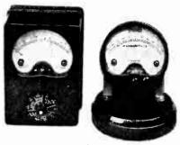
Ferranti valve-tester (left) which checks valve voltages and currents in situ in a receiver. On the right is a sensitive microammeter with centre zero.
