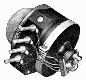
Fig. 2.—Antimicrophonic valve holder used in Marconi shortwave set. The base and glass bulb of the valve are supported in stockinette providing the highest degree of insulation from shock. Note the flexible leads.
