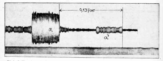
Fig. 1 .- Oscillograph record of Morse " dot " sent from Rio de Janeiro on 15.66 metres and received at Geltow, Germany.
