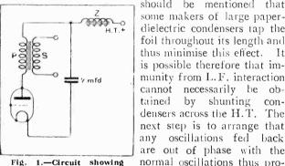
Fig. 1.—Circuit showing method of preventing L.F. back-coupling by the inter-position in each H.T. lead of a L.F. choke.
