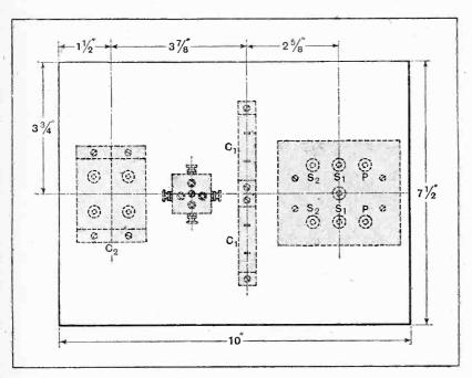
Fig. 10.-Layout of the parts for the rectifier.
