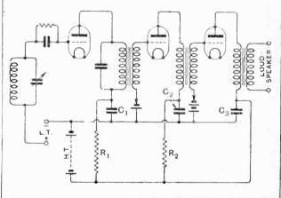
Fig. 2.—A receiver fed from a common H.T. battery through resistances. It is claimed that the tendency to L.F oscillation is eliminated.  $C_1$ ,  $C_2$  and  $C_3$  are 2 mfd. and  $R_1$  and  $R_2$  are of the order of 25,000 ohms. Tappings are avoided on the H.T. battery which is thus evenly exhausted.
