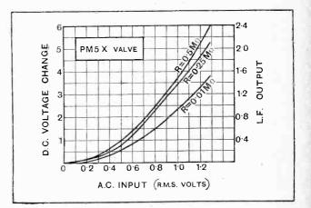
Fig. 5.-Voltage changes produced with the PM5X valve used as an anode bend rectifier.
