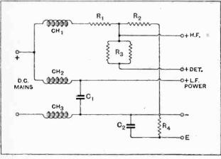
Fig. 4.—When the mains are very rough an additional choking coll may have to be connected as shown at CH<sub>3</sub>.
