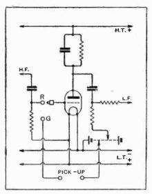
Detector circuit connections for using gramophone pick-up in tuned anode receiver.
