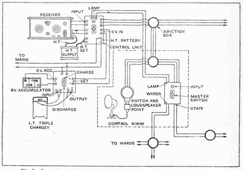
Fig. 2 .- Connections of the control apparatus in the Burndept "Auto Broadcast" system.
