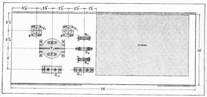
Fig. 5 .- Position of the parts on the baseboard.
