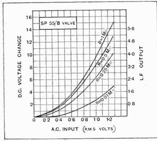
Fig. 4.—Rectification obtained with the SP.55B valve. B I 7
