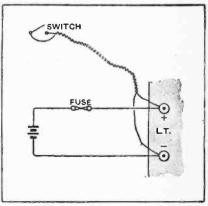
Switching off L.T. by means of a fuse.
