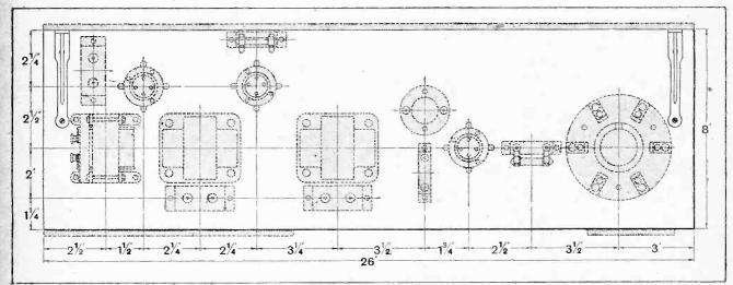
Fig. 7.-Dimensional layout of components on baseboard.
