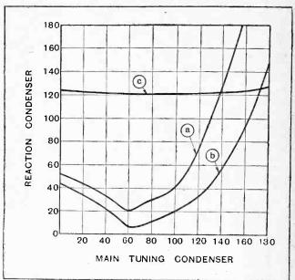
Fig. 4.—Experimental curves of relation between reaction and tuning controls; (a) small capacity, large coil and loose coupling,
