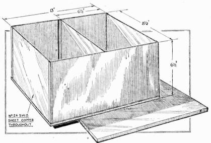
Fig. 2 .- Details of the copper box and lid.
