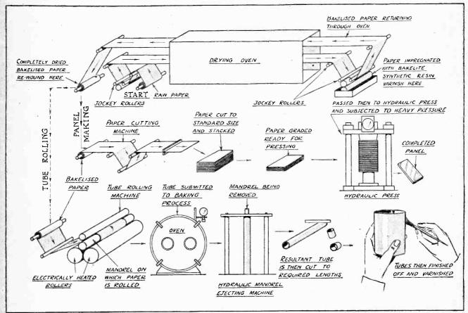
Fig. 2.-Schematic drawing showing the successive manufacturing processes employed in the production of Paxolin boards and tubes.
