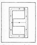
Fig. 4.—Iron core laminations of typical shape showing mean length of magnetic circuit. a special construction of the iron circuit. However, the value of inductance obtained is in general just as constant and definite as before, and it would appear that for reasonably small voltages there is not very much distortion occasioned by this flow of current.
