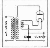
The unidirectional conductin a battery eliminator causes successive charges to be trapped in condenser C.
