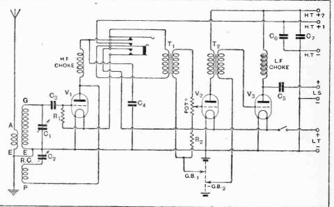
Fig. 1.—Complete circuit diagram.  $C_1 = 0.0005 \text{ mfd.}$ ,  $C_2 = 0.0003 \text{ mfd.}$ ,  $C_3$ ,  $C_4 = 0.0003 \text{ mfd.}$ ,  $C_5$ ,  $C_8$ ,  $C_7 = 2 \text{ mfds.}$ ,  $R_1 = 2 \text{ megohms}$ ,  $R_2 = 0.5 \text{ megohm.}$
