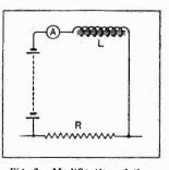
Fig. 3.—Modification of the inductance arm of the hridge for measuring the effect of a steady D.C. "polarising" current.
