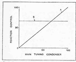
Fig. 3.—Two ideal conditions of reaction control; A, in which reaction setting is exactly proportional to tuning condenser setting, and, B, constant over the whole of the tuning scale.
