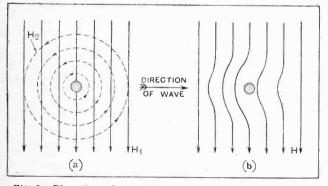
Fig. 5.—Distortion of magnetic field in the vicinity of a tree;  $H_1 = field$  due to transmitter,  $H_2 = field$  due to tree, H = resultant field.
