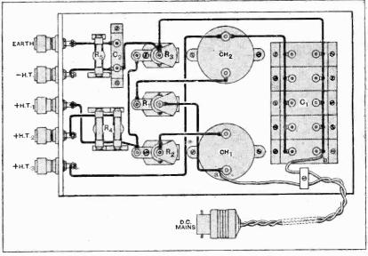
Fig, 9.-Wiring diagram of the D.C. eliminator.
