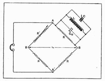
Fig. 1.—Bridge circuit for investigating the properties of ironcored inductance windings.
