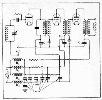
Fig. 5.—The anode-feed resistance scheme as applied to a D.C. H.T. eliminator. The important claim is made that no "motor-boating" can occur and that the amplification curve is the same as in the ideal case where separate H.T. batteries are used for each anode
