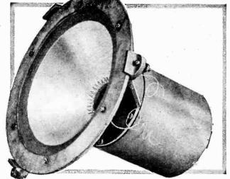
A completed loud-speaker. (The front projecting lugs are no longer provided as will be seen in the set of castings shown earlier.)
