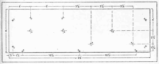
Fig. 6.—Drilling details of front panel. Sizes of holes are as follow:—A, 3/8in. dia.; B, 1/8in. dia., countersunk for No. 4 wood screws; C, 1/8in. dia., countersunk for 6B.A. screws; D, 3/32in. dia.
