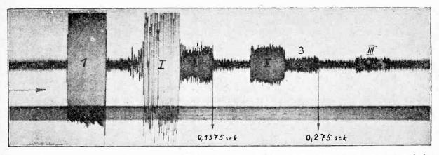
Fig. 3.—Oscillograph record of two "dots" sent from Rio de Janeiro and received at Geltow; the record shows two groups of echoes produced by waves which have travelled once and twice round the earth respectively.
