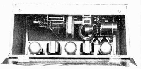
Plan view of interior from back of set; the tuning and reaction coils are assembled in the top right-hand corner.
