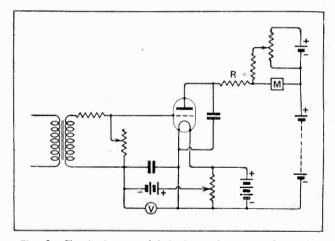
Fig. 2.—Circuit for examining the performance of a valve adjusted as an anode bend rectifier. Alternating input potentials are obtained from a 50-cycle alternating supply and the change of anode current is observed on the microammeter M set for reading from zero.
