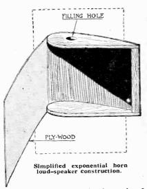
These can be conveniently made of 3-ply wood in the form of boxes, as shown in the sketch. To prevent the interior from resonating the box should be filled with dry sand through a filling hole in the top; internal battens may be necessary if the sides show any tendency to bulge.— R. W.
