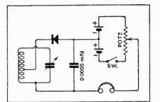
Fig. 2. Potentiometer connections giving positive or negative bias.
