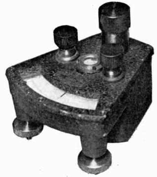
Fig. 5.—Pye suspension type moving-coil galvanometer with pointer and scale, in which readings as small as 0.25 microampere can be taken. This instrument is marketed at a very popular price.
