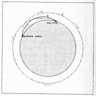
Fig. 2.—Showing track of waves producing the deflections a and a' in the record in Fig. 1.
