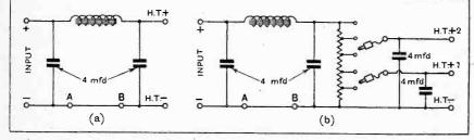
Fig. 1 .- Smoothing circuit and potential divider for use with the "A.C. Trickle Charger."
