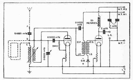
Fig. 1.-Two-valve receiver for use with frame or open aerial.
