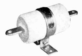
Fig. 8.—A 0.015 mfd. transmitting condenser selling at a popular price and made by the Dubilier Company. It is capable of passing 5 amps when used on 100 metre transmission.
