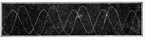
Fig. 3.—Oscillograph photograph of input and output waves of amplifier shown in Fig. 2. There is no evidence of wave-form distortion.
