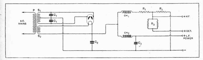
Fig. 6 .- Connections of the complete eliminator for working off A.C. mains.
