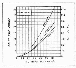
Fig. 3.—D.C. potential changes produced by various values of A.C. potential applied to the grid of a B8 valve arranged as an anode bend detector.
