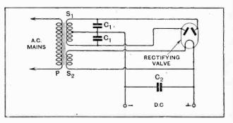
Fig. 5.—A rectifying unit. Condensers  $G_1$  are of 0.1 mfd. each, and  $G_2$  of 4 mfd.
