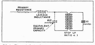
Fig. 6.—The equivalent primary capacity transferred from the secondary is increased as the square of the step-up ratio.
