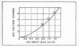
Fig. 6.—A typical graph showing the relation between input H.F. potential and the rectified voltage output of an anode bend detector. Note the curvature of the graph for small input potentials, a condition which will give rise to distortion.
