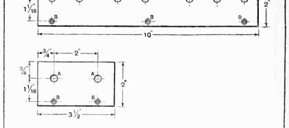
Fig. 8.—Drilling details of terminal strip; A, 5/16in. dia.; B, 1/8in. dia., counter-sunk for No. 4 wood screws.
