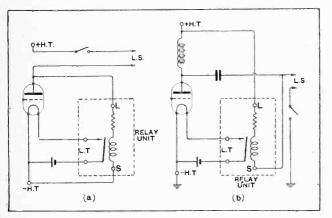
Fig. 3.—Circuit connections of the "Teletrol" system; (a) for loud-speakers connected directly in the anode circuit and (b) for choke-capacity output.
