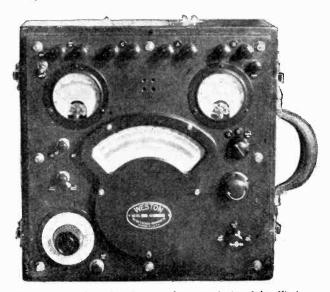
Fig. 4.—Valve characteristic recorder manufactured by Weston Electrical Instrument Company. A.C. resistance, magnification factor, and mutual conductance, are shown as dial readings.
