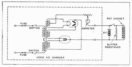
Fig. 1.-Method of energising 6-volt field winding of moving-coil loud-speaker from A.C. mains.
