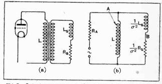
Fig. 7.—Output transformer feeding into a loud-speaker represented in (a) by  $L_s$  and  $R_s$ . The equivalent primary circuit is indicated in diagram (b).
