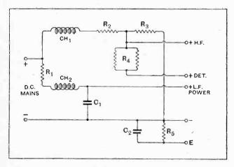
Fig. 3.—An eliminator for attachment to direct current mains for the "Everyman Four" receiver. Resistance  $R_1$  may be of 5000 ohms when the mains voltage is 240 and the full amount is not required across the L.F. and power valves. Values for resistances  $R_2$  and  $R_3$  are given in the text.  $R_1$  comprises two o.5 megohm resistances in parallel, and  $R_3$  is of 0.25 megohm. B 11
