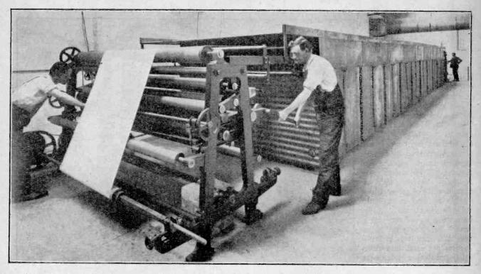
Fig. 3.-Paxolin paper varnishing machine equipped with steam-heated oven 75ft. long.
