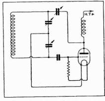
Twin condenser for overcoming hand-capacity in the Hartley circuit.
