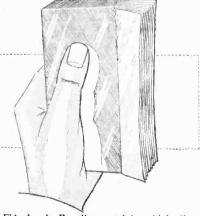
Fig. 1.—A Paxolin panel in which the pressing process has not been applied to the extreme edge; note the laminations.
