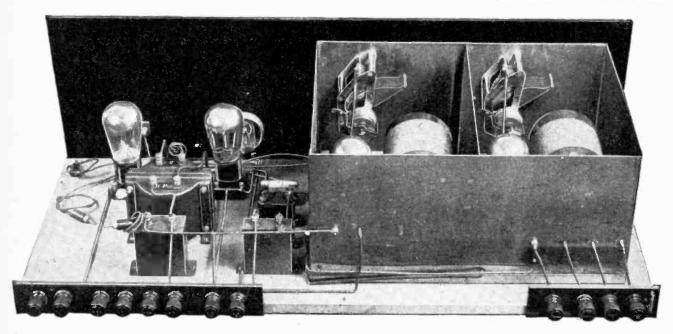
The finished set complete with coils and valves.
