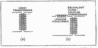
Fig. 5. — Transformer (a) with magnetic leakage, and (b), the equivalent circuit with leakage inductance referred to one winding.
