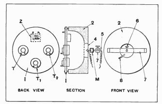
Fig. 7.—Constructional details of carbon microphone and telephone unit.
