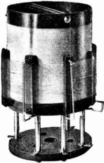
The long-wave coil for the "All-Wave Four" with base piece,
