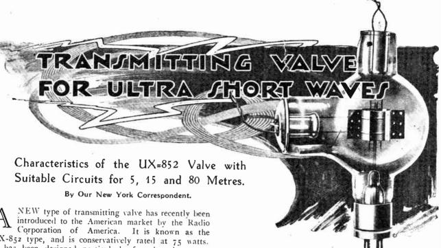
NEW type of transmitting valve has recently been introduced to the American market by the Radio Corporation of America. It is known as the UX-852 type, and is conservatively rated at 75 watts. It has been designed particularly for ultra-short-wave work, and it is free from excessive strains, can be wired very easily, and is relatively cool in operation. It is capable of oscillating at frequencies even below one metre.
