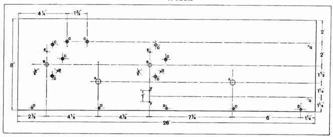
Fig. 7.—Details of chonite front panel. The holes have the following diameters:—A, 7/16in. dia.; B, 5/16in. dia.; C, 5/32 dia. countersunk for No. 4 B.A. screws; D, 1/8 dia. countersunk for No. 4 wood screws; E, tapped holes for dials; F, 3/32 dia.; G, tapped 6 B.A. + 1/8in. deep.
