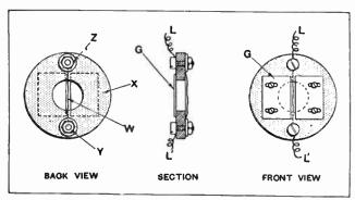
Fig. 3.--Constructional details of the hot-wire microphone.
