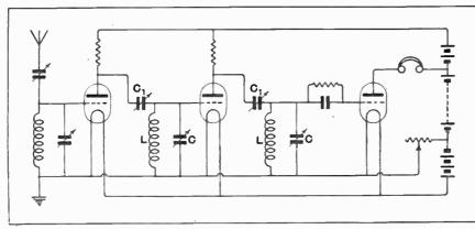
H.F. amplifier combining tuned and resistance intervalve couplings (No. 272,294.)
