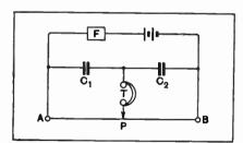
Fig. 1.-A simple capacity bridge.
