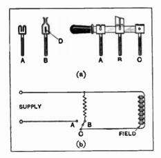
Fig. 2.—Safeguarding loud-speaker field windings.
