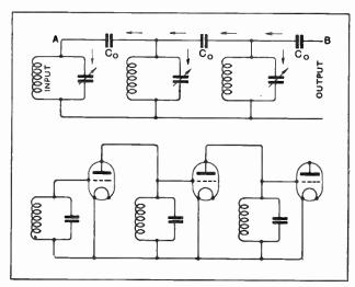
Fig. 1.—Illustrating the energy feed back due to the valve capacity Co of the grid-anode circuits. Unless the energy in its return path is a ufficiently attenuated the set will oscillate.
