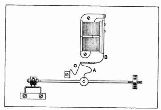
Fig. 4.—Operating panet (B) engaging spring catches (A) and (C).
