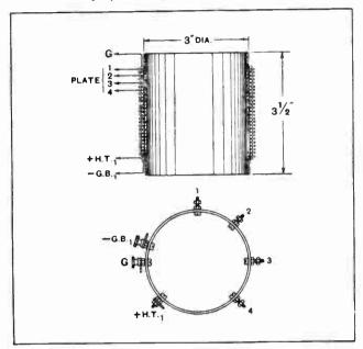
Fig. 5. — Winding details of the intervalve transformer. Terminal G and screws 1, 2, 3, 4, are at the upper end of the coil; terminals — GB, and + H.T., are at the bottom. The secondary has 68 turns of 27,42 Litzendraht, and the primary comprises 68 turns of No. 40 D.S.C., tapped at 38, 48, and 58 turns.
