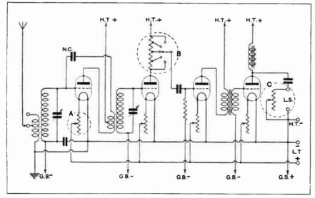
Fig. 1.—Typical receiving circuit showing alternative volume controls.
