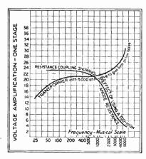
The Curves show the distortion effects in the amplification—frequency curves of a good transformer, a high anode resistance unit and the "Cosmos" Resistance Unit using low anode resistances and large coupling condenser.
