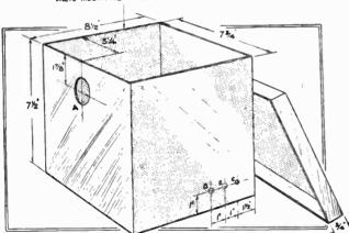
Fig. 9.—The copper screening box, with holes for terminals, connecting wires, valve, and the toning condenser and volome control. A, hole 131n. dia. for valve; B, holes 3 81n. dia. for ebonite bushes to take aerial terminals; C, hole 7/32in. dia. for earth terminal.
