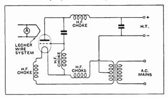
Fig. 3.—Circuit for wavelengths below 5 metres
