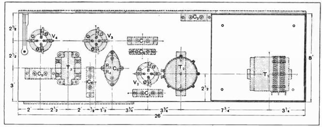
Fig. 8.-Arrangement of parts on the baseboard
