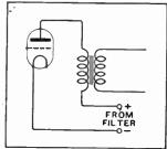
Fig. 3.—Typical output circuit of receiver.
