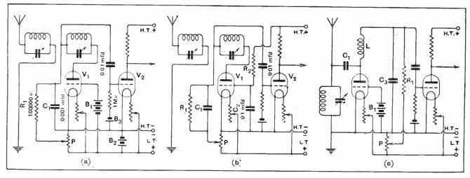
Fig. 2.—Using a three-electrode valve as a two-electrode rectifier
