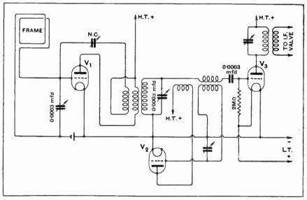
Fig. 2.—Adding a stage of H.F. amplification to a superheterodyne receiver.
