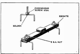
Fig. 1.-Ebonite arm and connecting links.
