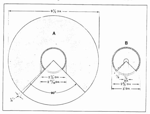
Fig. 3.-Method of marking out paper for diaphragm, A, and reinforcing cone, B.
