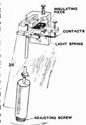
Constructional details of a pendulum used for releasing the rotating cylinder at two-second intervals
