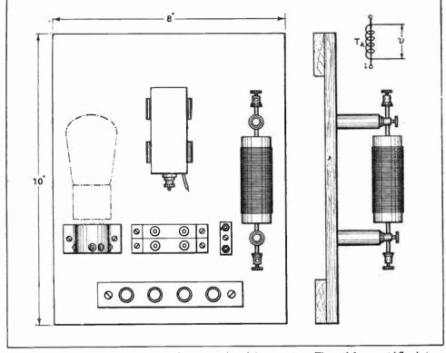
Fig. 2.—Layout of the valve and transformer portion of the ammeter. The aerial current i flowing through the primary rod of the transformer  $T_A$  produces a voltage v across the secondary which is measured by the valve.
