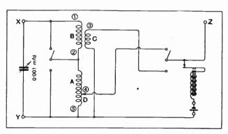
Fig. 1.—Theoretical diagram. The numbers and letters correspond with the wiring diagram in Fig. 4.
