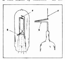
The use of a bimetallic strip for maintaining valve filament basin.
