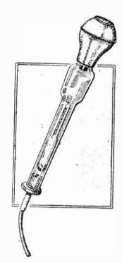
Acid is withdrawn from a cell by suction and the gravity readily revealed by the hydrometer.
