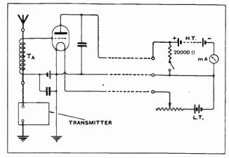
Fig. 1.—Circuit arrangement of the remote indicating aerial ammeter. The receiving set H.T. and L.T. batteries may be used for the ammeter as well if desired.
