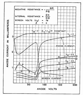
Fig. 6.—Characteristic curve of the Osram screen grid valve, showing anode current, screen current and total current for various values of anole voltage and a screen voltage of 79. The total current or electron emission is the screen current plus the anode current,  $I_a + I_a$ , which is substantially constant. The negative resistance  $-\frac{QR}{PQ} = -7 \times 10^4$  ohms.
