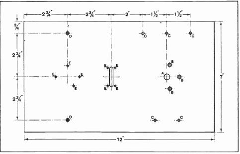
Fig. 3.-Arrangement of parts on the panel.
