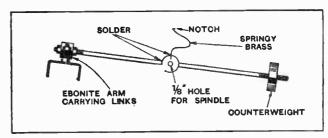
Fig. 2.-Plyoted arm with counterweight and spring catch.
