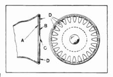
Loud-speaker attachment to reduce distortion and blasting. (No. 270,073.)
