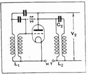
Fig. 13.—The circuit of Fig. 12 r drawn and simplified to show essential features.
