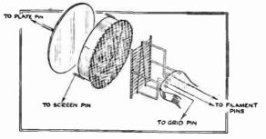
Fig. 3.—Arrangement of the electrodes of the new Marcon and Osram Screened Valve.
