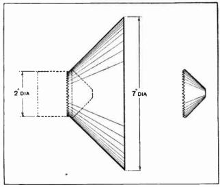
Fig. 4.-Leading dimensions of finished diaphragm.
