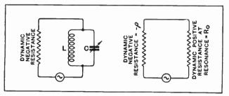
Fig. 7.—Hustrating the negative resistance effect of the screen grid vaive. For oscillation  $R_0-\rho$  must be negative. At a frequency of a million (300 metres) oscillation will not occur with a low loss coil unless resistance amounting to a few times the coil resistance is added.
