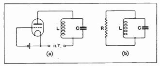
1.—The internal resistance of a valve exercises a damping effect on tuned circuits connected in the anode circuit.
