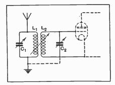
Fig. 3.—The simple loose-coupler is still one of the best methods of obtaining selectivity.
