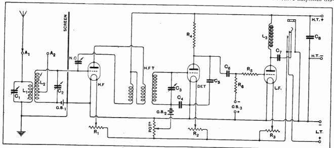
Fig. 1.—The circuit diagram. C<sub>1</sub>, C<sub>2</sub>, C<sub>3</sub>, 0.0005 mfd.; C<sub>4</sub>, 0.25 mfd.; C<sub>5</sub>, 0.0001 mfd.; C<sub>6</sub>, 0.005 mfd.; C<sub>7</sub>, C<sub>6</sub>, 2 mfds.; R<sub>1</sub>, R<sub>2</sub>, 30 ohms; R<sub>3</sub>, 6 ohms; R<sub>4</sub>, 250,000 ohms; R<sub>5</sub>, 0.25 megohm; R<sub>6</sub>, 2 megohms; L<sub>3</sub> is the output choke.
