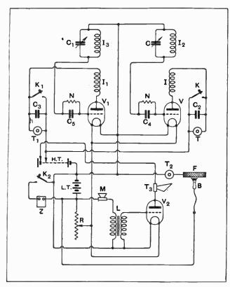
Fig. 5.-Circuit diagram of interference tester.
