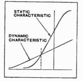
Fig. 4.—Curves showing correct setting of grid blas for a power valve with an inductive load in the anode
