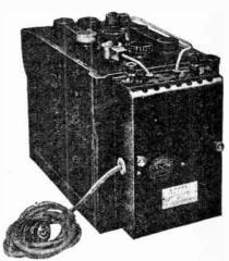
A convenient form of Kupox battery charger. It is bridged across the battery terminals and the electric light adaptor is connected to the supply when the battery requires recharging.
