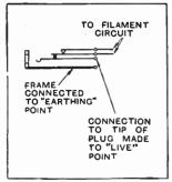
Fig. 2.—Typical jack for stageswitching. The frame should be connected to a point of "earth" potential which may be + H.T.
