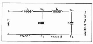
Fig. 11.-Circuit of two-stage filter.
