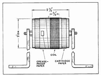
Fig. 5.-Method of winding the moving coll.
