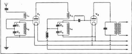
Receiver with constant coupling in aerial and intervalve circuits. (No. 256,967.)
