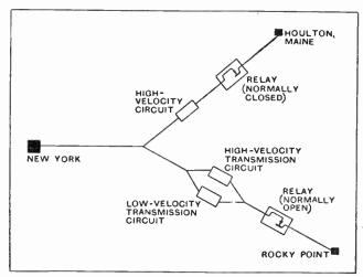
Fig. 1.—Arrangement of voice-operated relays in transmission circuits between New York and the transmitting and receiving stations at Rocky Point and Houlton, Maine.
