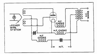
Fig. 2.—Transmitting circuit for wavelengths between 5 and 15 metres,
