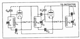
Fig. 12.—Two-stage amplifier with centre-tapped coils.
