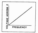
Fig. 5.—The characteristic or amplification curve for a ocreened valve with a pure inductance.
