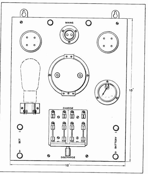
Fig. 2.-Layout of components on the charging board.
