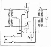
Push-pull amplifier with filaments in series. (No. 271,222.)
