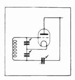
Fig. 11.—" Bridge" circuit with divided tuning condenser.
