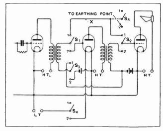
Fig. 4.—Ideal stage switching arrangement operating according to the scheme of Fig. 1(b). The lead  $\hat{X}$ , which connects across the optional stage, is completely isolated when not in use, or may be "earthed" by a switch  $S_5$ .
