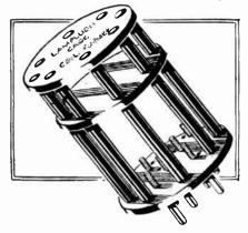
Lamplugh former for H.F. transformer construction.
