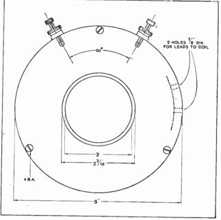
Fig. 1(b).-End elevation of field magnet.
