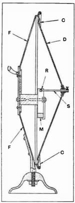
Constructional details of conical diaphragm loud-speaker embodying a modified method of clamping at the rim. (No. 252,685.)
