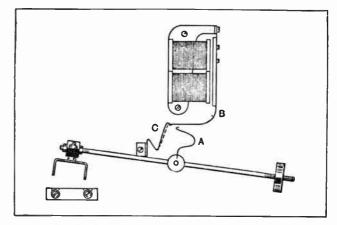
Fig. 5.—Operating panel releasing spring catches.
