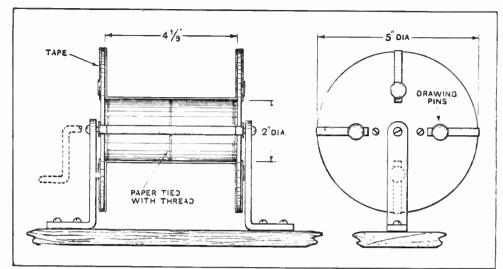
Fig. 2 .- Winder for field magnet coil.
