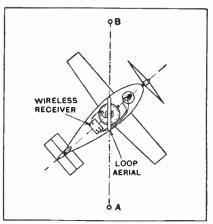
Rotating frame receiver for use in aerial navigation. (No. 265,940.
