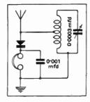
Fig. 1.—Simple crystal set using centre-tapped coil.
