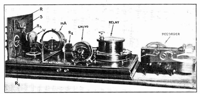
Fig. 1.—General view of audio-resonant recording apparatus.
