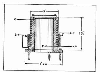
Fig. 8.—Section through the long-wave H.F. transformer, showing arrangement of windings. A crossbar of i-in. ebonite tube is fitted.
