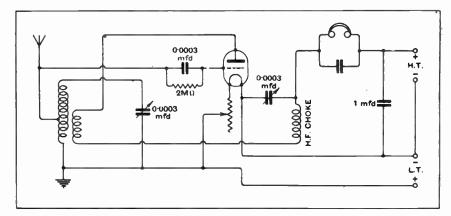
Fig. 1 .- A sensitive and selective single valve circuit.
