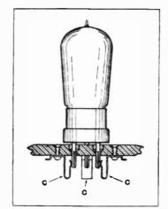
Contact can be made only with the spring connectors when the pins have passed through the locating holes. Accidental contact between the filament pins and the H.T. supply is thus avoided.
