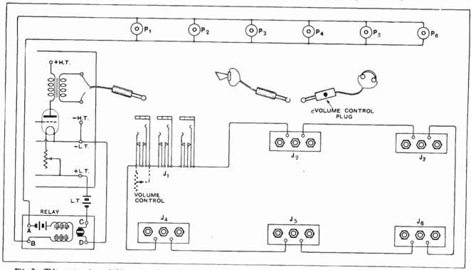
Fig. 2.—This system is probably more suitable for the average household. It should be noted that the connection boxes  $J_2$  to  $J_3$  are precisely similar to  $J_1$ .
