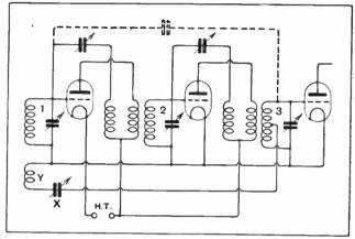
Fig. 15.—Compensating for capacity coupling between circuits 1 and 3 by means of a subsidiary circuit XY.
