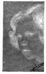
Half-tone image prepared with a 40 line screen, the varying widths of lines and spaces producing light and shade. The image is recorded by the gum-bichromate process on a thin copper foil, so that when bent round the cylinder of a picture transmitter and traversed by a metal point a circuit is interrupted by the gum deposit, which in turn "keys" the wireless transmitter.
