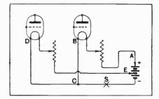
Fig. 2.—Illustrating a possible source of danger when connecting two-volt and sixvolt valves to a common L.T. battery.
