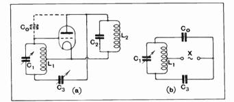
Fig. 11.-The "bridge" method of neutralisation due to Rice.
