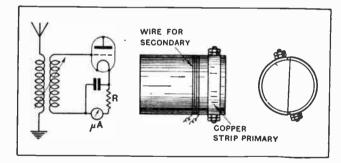
Actually a W.E. "Peanut" valve, with grid and plate connected together, was used as a diode. This arrangement has the advantage that the calibration is independent of the filament temperature, provided the valve is run bright enough to give sufficient emission. It has the disadvantage of requiring more power than either type of triode voltmeter.
