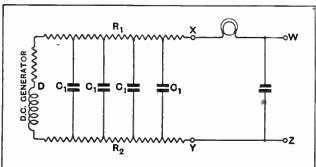
Fig. 2.—Distributed resistance and capacity in the mains assists in smoothing the current supplied.
