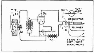
Fig. 6.—Circult system for producing an artificial source of interference.
