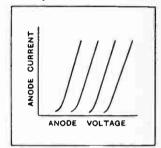
Fig. 8a. — Characteristic curves of three electrode valve for various values of grid hias. The curvature is opposite from that of Fig. 6 and the slope is much greater.
