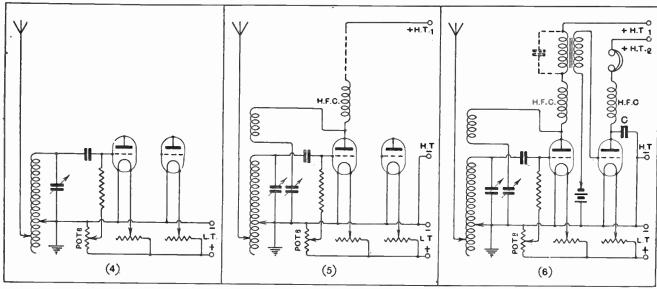
A grid condenser is inserted, and the low potential end of its leak is joined to the silder of a potentiometer, the resistance element of which is connected across the low-tension battery.
