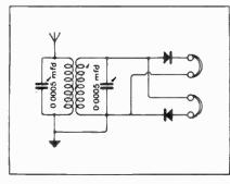
Fig. 1.—Crystal receiver designed for fullwave rectification
