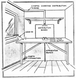
A suggested arrangement of the receiver room. The wooden casing for the distribution wires should be specially noted.
