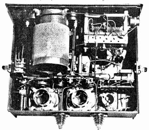
A number of bamboo Fig. 2.—Interior of transmitter. The long-wave tuning coils are on the left and the short-wave on the right
