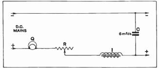
Fig. 8.—Smoothing circuit for obtaining H.T. supply from D.C.
