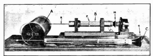
Fig. 2.—Three experimental hot-wire microphones and resonators.
