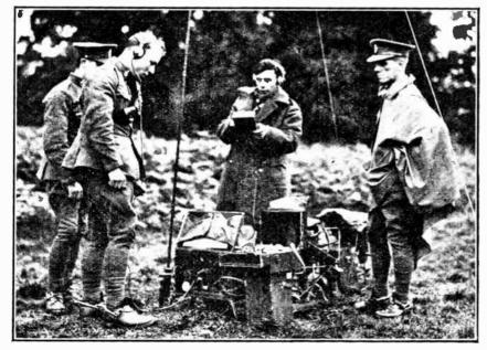
THE MILITARY PORTABLE IN ACTION. The apparatus used by the 54th East Anglian Divisional Signals can be quickly set up and dismantled. Note the fishing-rod aerial mast supported by a bayonet, which also acts as "earth."
