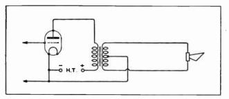
Fig. 3.—By means of a step-down output transformer with centretapped sccondary, opposite voltages of low value are produced on the loud-speaker leads, thus cancelling the electrostatic fields. Twin leads must be used, otherwise an increased electromagnetic effect is probable.
