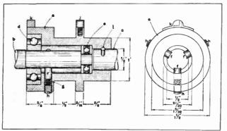
Sectional view of the clutch. (a) Turned brass housing. (b) End of shaft of clockwork motor. (c) Cylinder shaft. (d) Ball race. (e) Thrust race. (f) Fibre plungers. (g) Tension springs. (h) Adjusting screws. (j) Stop to arrest rotation. (k) Cam for two-way switch. (l) Securing pin.
