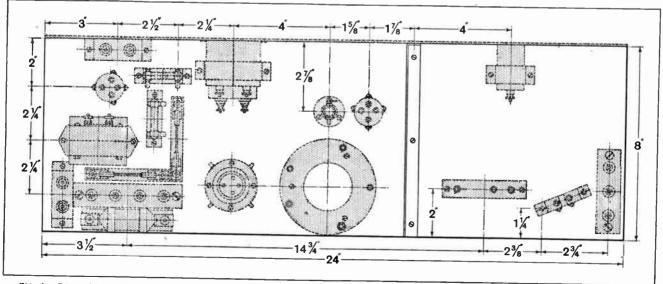
Fig. 6.—Disposition of components on the baseboard. The bias battery  $GB_2$  and the by-pass condenser  $C_4$  are secured in position by the same metal strap.
