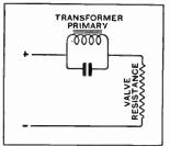
Fig. 4.—Equivalent circuit of output from receiver.
