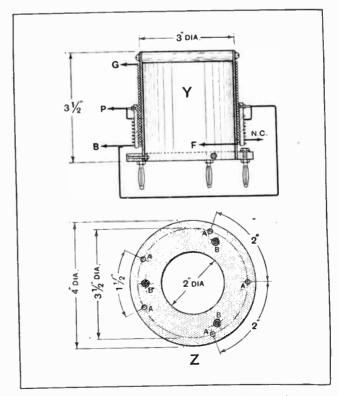
Fig. 4.—Y, Details of the short-wave H.F. transformer. Z, Transformer base. Position of holes for sockets are sbown at A, and those for the holding-down screws at B
