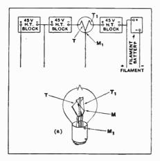
Protecting lamp with midpoint tapped filament connected in series with the anode batteries. (No. 252,181.)
