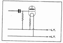
Fig. 1.—Obtaining grid bias by connecting the filament resistor in the negative L.T. lead.
