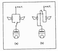
Fig. 2.-Alternative method of switching loud-speakers.
