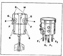
Method of supporting and connecting up the filaments, grids and plates of multi-electrode-valves. (No. 271,558.)
