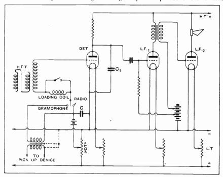
Fig. 1.—Showing method of connecting a gramophone pick-up device to a conventional receiver. C is the usual by-pass condenser across the potentiometer and grid bias battery, while C<sub>1</sub>, the anode by-pass condenser, may be removed when the detector valve is converted into an L.F. amplifier.
