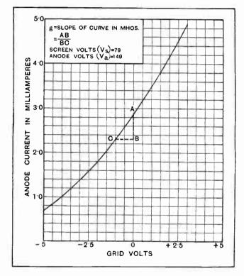
Fig. 8.—Curve showing the mutual conductance of the Osram screen valve.
