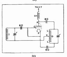
Circuits of stabilised H.F. amplifier. (No. 270,531.)
