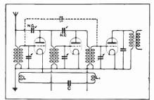
Auxiliary circuit for neutralising residual coupling effects. (No. 271,253.)
