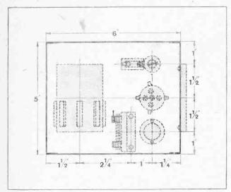
Fig. 3.-Layout of apparatus on baseboard of radio receiver.
