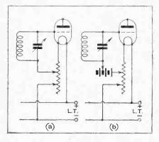
Fig. 1.—Connecting a filament rheostat to control grid hias.
