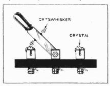
S.P.D.T. knife switch converted to a crystal detector.
