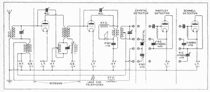
Fig. 6 .- Schematic diagram showing how the crystal in Fig. 5 may be replaced by well-known reacting valve detectors.
