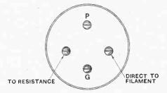
Fig. 6.—Conventional method of connecting internal filament resistance.
