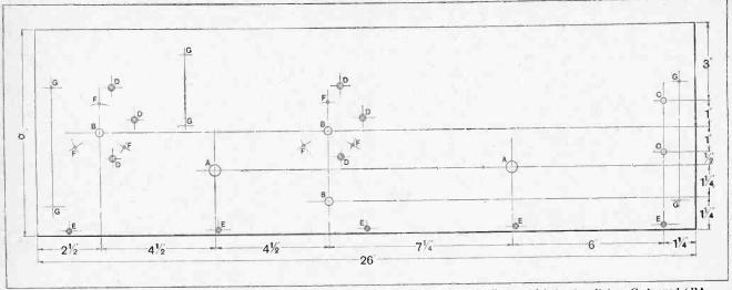
Fig. 5.—Details of ebonite front panel. A, 7/16"; B, 5/16"; C, 7/32"; D, 5/32"; E, 1/8"; F, tapped holes for dials; G, tapped 6BA for brackets and screen.
