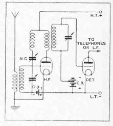
Fig. 2.—An H.F. and detector combination with lightly damped circuits.
