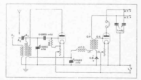
Fig. 1.—A sensitive arrangement of two valves.
