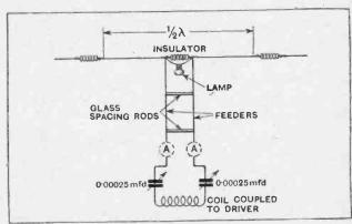
Fig. 3.—Hertz aerial with twin feeders. The lamp is removed and ammeters inserted in each feeder after wavelength adjustment.
