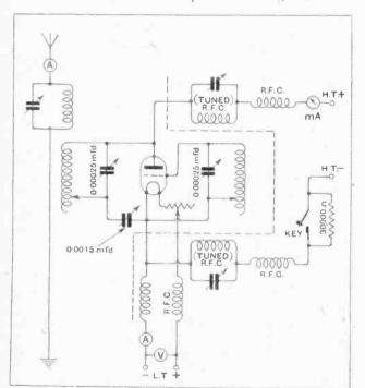
Fig. 1.—Complete circuit diagram of transmitter arranged for third narmonic excitation. The portion to the right of the dotted line is built as a separate unit.
