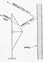
Fig. 2.—Direct and reflected waves from cone loud-speaker.
