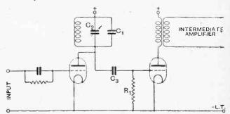
Fig. 1.—Connections of tuned-anode circuit with auxiliary condenser for changing the intermediate frequency.
