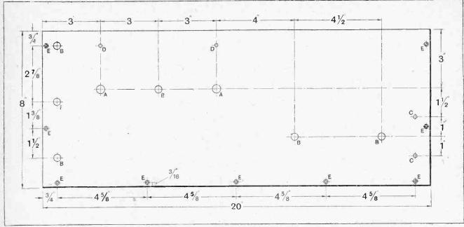
Fig. 2.—Dimensional details of the front panel. Drilling sizes are as follow: A, 7/16in. dia.; B, 3/8in. dia.; C, 3/16in. dia.; D, 5/32in. dia.; E, 1/8in. dia.; and countersunk for No. 4 wood screws.
