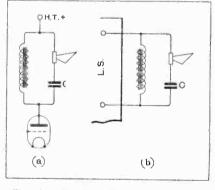
Fig. 1.—(a) A choke-capacity output circuit. At (b) its connections to the loud speaker terminals of an existing set are shown.
