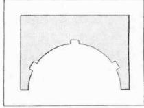
Cardboard jig for assembling spacing strips on H.F. transformers.
