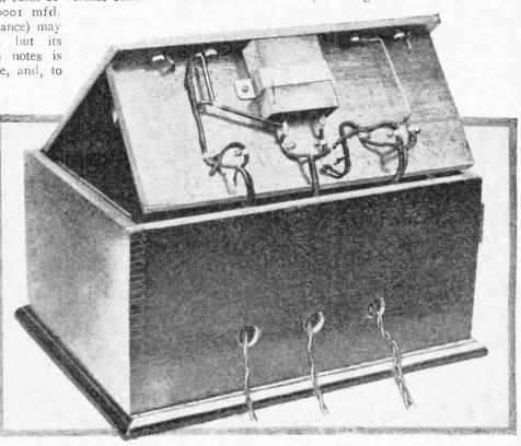
The set partly removed from the cabinet. The method of securing the flexible leads is clearly shown.
