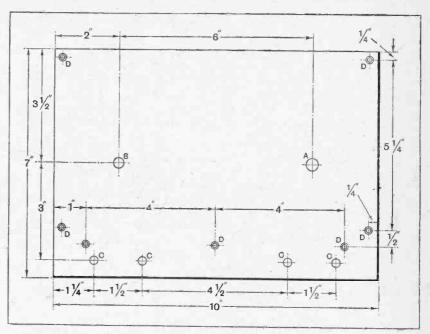
Fig. 2.—Drilling details of top panel. A, 3 8in. dia.; B, 5/16in. dia.; C, 1/4in. dia.; D, 1/8in. dia., countersunk for No. 4 wood screws.
