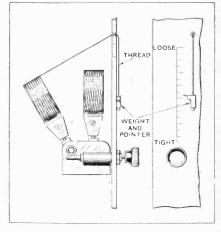
Coupling indicator for coils mounted behind the panel.
