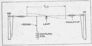
Fig. 2.—Half-wave Hertz aerial with single feeder. The dotted line indicates the voltage distribution.
