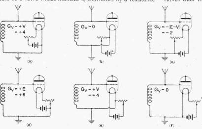
Fig. 1.—Six methods of connecting filament battery, filament resistance and grid return lead to obtain various values of grid bias. V=normal filament voltage=4; E=voltage of L.T. battery=6.
