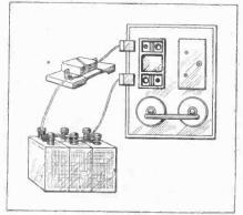
Fig. 4,-Charging batteries from the mains.
