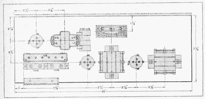
Fig. 3 .- Details of the baseboard layout.
