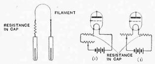
Fig. 4 .- Special case of peranent resistance in series with the valve filament.
