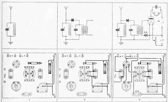
Aerial and earth are joined to an inductance coil, across which is connected a variable tuning condenser.
