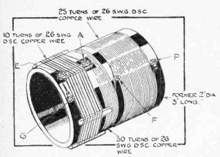
Fig. 5.—Details of the tuning coil. E=earth; B=aerial; G=grid; P=plate.
