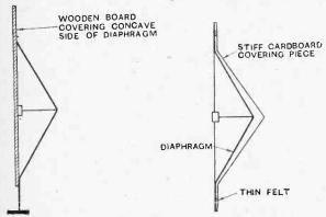
Fig. 6.—Experiment to show suppression of low tones by closing one side of diaphragm
