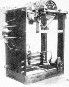
The circuit chosen, after many trials, is the runed grid and plate arrangement, commonly known as the Armstrong circuit (Fig. 1).
