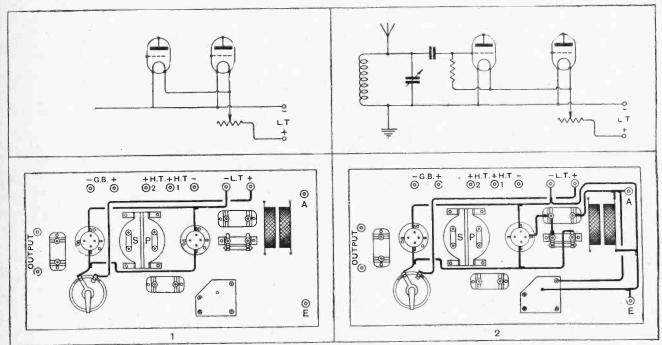
The filament circuits are wired in the usual manner. In this particular case a single rheostat issued to control both valves
