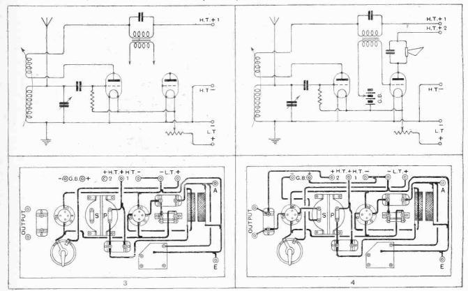
The plate circuit of the detector valve is completed through the reaction coil, the primary of the L.F. transformer, and the H.T. battery.
