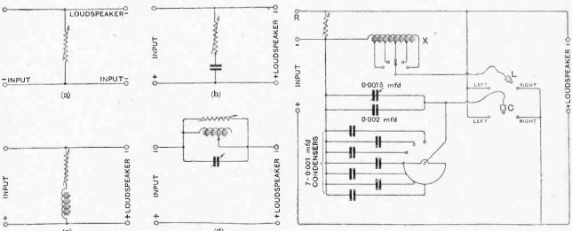
Fig. 1. Fig. 2. Fig. 1.—Universal tone control circuits. Fig. 2.—Complete circuit diagram. Positions of sockets for the circuits in Fig. 1. are as follow: (a) L. centre, C, centre; (b) L, centre, C, right; (c) L, right, C, centre; (d) L, left, C, left. in circuits (a), (b) and (c) the "Input" terminal is joined to R.
