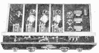
Seven valve "Howard" neutrodyne receiver with top shield removed. The condensers tuning the three H.F. stages are interconnected by a link motion between the front panel and screening hox. The three L.F. stages are coupled by one 2 to 1 and two 1 to 1 ratio transformers.
