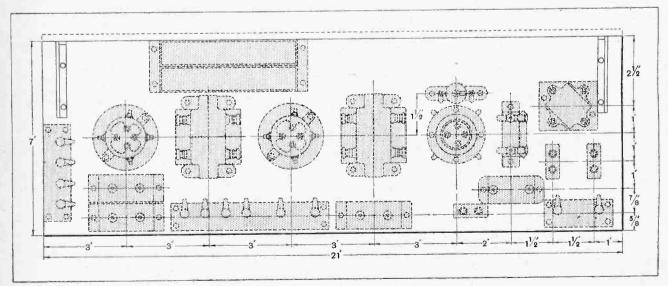
Fig. 3.-Layout of components on baseboard.
