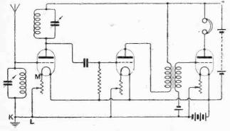
Fig. 3.—Typical three-valve receiving circuit.
