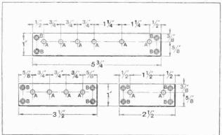
Fig. 4.—Terminal strips. A, 7/32in. dia.; B, 1/8in. dia., countersunk for No. 4 wood screws.
