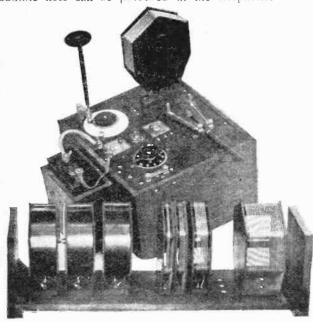
Fig. 2.—General view of wavemeter showing method of constructing short-wave coils.
