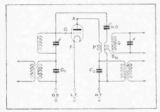
Fig. 1.—Single stage reflex amplifying valve with neutralised H.F. coupling.
