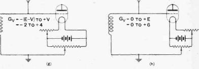
Fig. 2.—Range or voltages available with the addition of a potentiometer.
