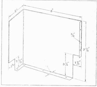
Fig. 4 .- The copper or aluminium screen.
