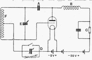
Fig. 1.-Circuit diagram of the wavemeter.
