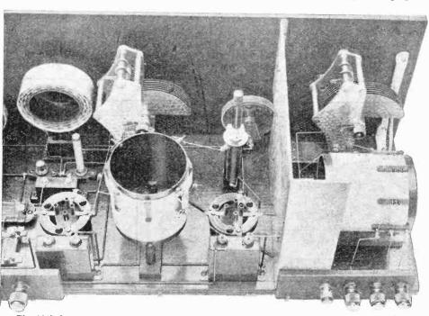
The high-frequency and detector circuits; on the right is the aerial coil, tuning condenser, connection strip and screen. Behind the right-hand valve-holder is the balancing condenser and volume control rheostat, while to the left can be seen the Daventry plug-in type coil.
