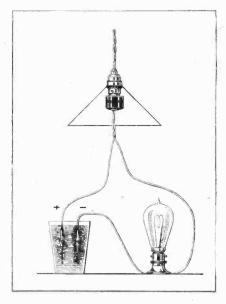
Fig. 2.-Testing mains for polarity.
