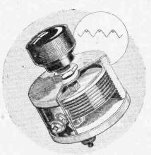
Totally enclosed rheostat in which the resistance wire is carried in a spiral groove so that maximum to minimum adjustment is spread out over seven complete turns of the knob.
