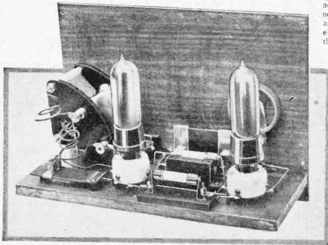
View of the underside of the panel, also showing layout of components on the sub-panel. The negative loud-speaker socket is that connected to the plate of the valve.
