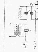
Fig. 2.—Neutralised tuned anode coupling.
