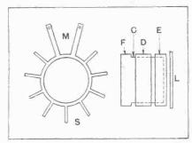
Former for winding double-weave coils No. 254,390).
