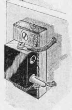
Fig. 5.—Mounting of the coil holder.
