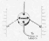
Method of bracing aerial down-lead
