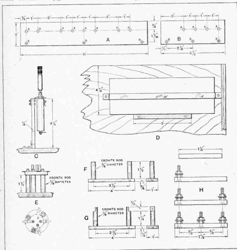
Fig. 3.—A and B, details of ebonite terminal strips: A, 7/32" diameter; B, 1/8" diameter. C: method of fixing balancing condenser. The upright piece is of ebonite and the two brackets of brass. D: method of fixing grid-bias battery to back of cabinet. E: valve-holder supports. F: base for aerial-grid coil. G: base for intervalve transformer. H: details of ebonite spacers.
