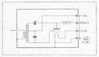
Fig. 2.-Showing the circuit of the radio receiver.
