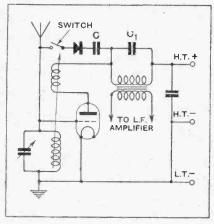
Fig. 1.—Changing from valve to crystal detection.
