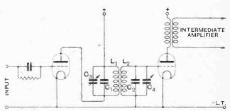
Fig 2.—Tuned transformer for coupling valves in the intermediate amplifier with auxiliary frequency changing condensers.
