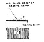
Fig. 2. Method of making tappings.
