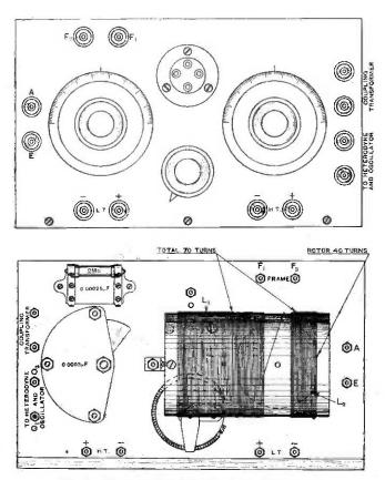
Fig. 4. Constructional details of the detector unit.
