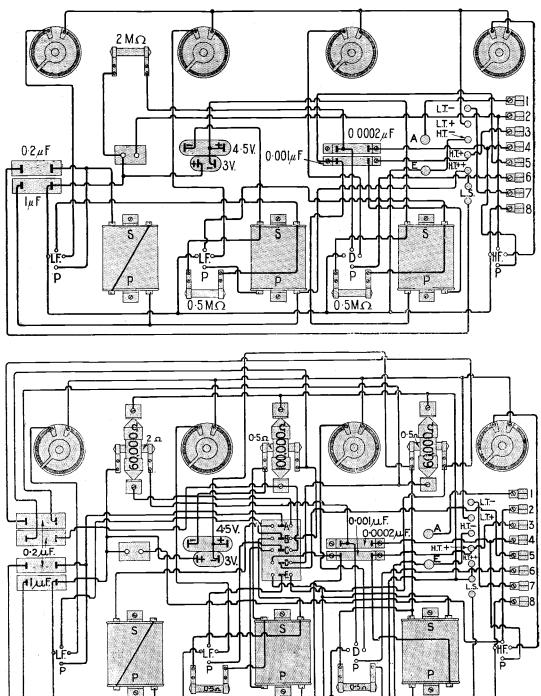
Two practical wiring diagrams. The resistance L.F. amplifying apparatus is omitted in the upper figure.
