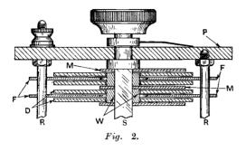
The spindle S, which is squared where it passes through the vanes, has fitted on to it the movable vanes, MM, spaced apart by the washers WW. Over these spacing washers are slipped the solid dielectric discs DD, which serve not only as dielectrics, but also to space apart the fixed (F) and movable (M) vanes so that they cannot touch each other.
