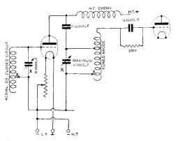
Fig. 2. An interesting H.F. amplifying arrangement. By reason of the small condenser in the plate lead it is possible to secure a higher potential across the anode coil than is normally possible. The H.F. feed choke must be well designed and of low self capacity to avoid excessive leakage.
