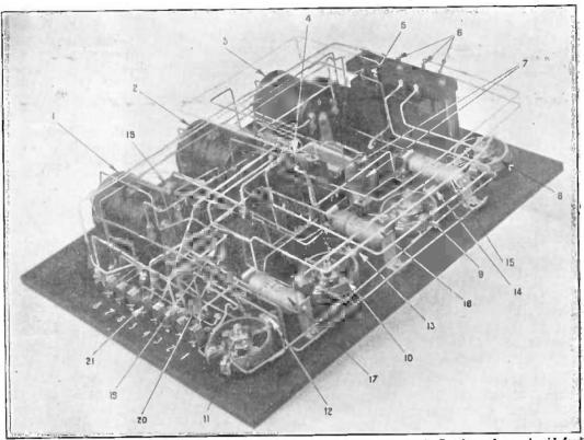
General view: 1, 2 and 3. Transformers. 4. Switch. 5. H.T. Condenser. 6. Loud speaker and grid feed condensers. 7. Grid cells. 8, 9, 10 and 11. Filament resistances. 12 and 13. Grid leaks of L.F. valves.
