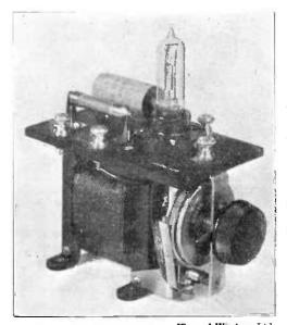
[General Wireless, Ltd. Fig. 2. One stage low frequency unit providing grid battery and resistance across transformer secondary to minimise distortion.
