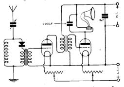
Fig. 1. "R.A.J." (Torquay). A crystal receiver with two note magnifiers.
