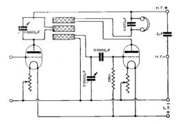
Fig. 1. "P.K.C." (Southport). A transformer coupled valve with reaction, using a three-coil holder.
