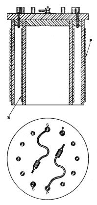
Fig. 26. A tapped transformer with the windings wound on tubes of different diameters.
