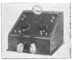
The constructor's two-valve receiver assembled. (Burndept
