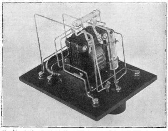
View of the underside. The method of wiring is clearly shown. The tinned ends of the high resistance (gridleak type) can be easily soldered to loops to avoid the fixing of brackets on to the panel, but care must be taken not to overheat the resistance.
