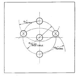
An enlarged drawing giving the exact setting out of the positions of the valve pins.
