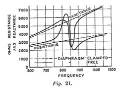
The ideal horn should therefore be made of a vibrationless material, and castings in iron have so far proved to give the best results. Anything of the nature of thin metal should be avoided, as invariably there is resonance frequency, often in the audible range.
