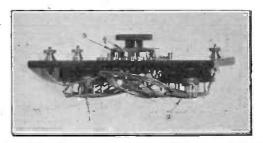
Fig. 13. A reactance unit consisting of two distinct coils, with one two-point switch for switching equal parts of each coil in circuit. (H. W. Sullivan, Ltd.)
