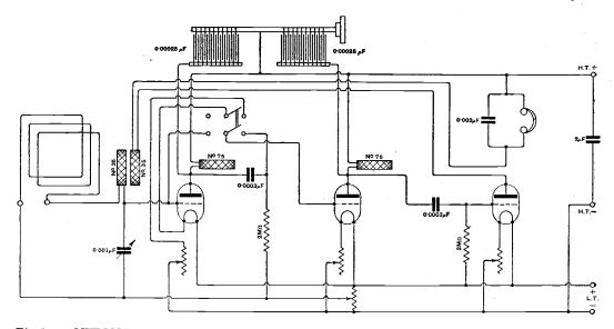
Fig. 1. "NITON" (Boscombe). Three-valve receiver (two H.F. and det.,) with switch to cut out one stage of H.F., and employing a coupled variable condenser for tuning the H.F. circuits.
