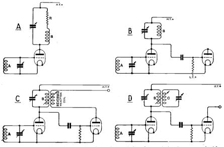
Fig. 2. Four methods for reducing the tendency of sharply tuned circuits connected with valves generating oscillations.
