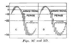
immediately it does so, the above process will go further. That is, after the circuit is again stable, the Armstrong oscillation will be slightly smaller, and the H.F. slightly greater, causing the second series to run slightly into the next cycle, as shown in Fig. 3D, and hence producing strong heterodyne.
