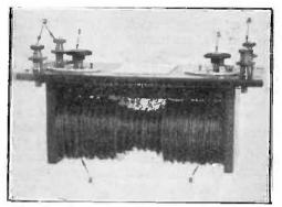
Fig. 9. A twner with multilayer coils. The coupling is fixed. (H. W. Sullivan, Ltd.)
