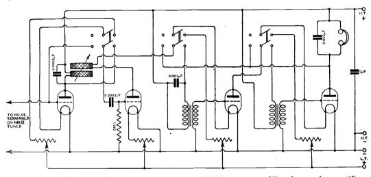
Fig. 2. "E.B." (Leeds). The first value operates as a high-frequency amplifier, the second as rectifier, and the last two as note magnifiers. The switches are connected so that the number of values in circuit may be easily varied.
