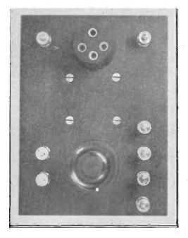
View of the top of the panel. The terminals can be identified by carefully enamelled lettering, or the panel can be put out for engraving before assembling.
