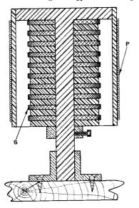
Fig. 27. A transformer with one winding in the form of a cylindrical coil, and the other consisting of a number of basket coils.
