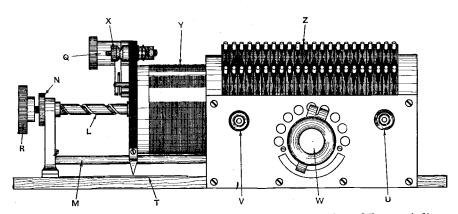
Fig. 8. Another type of long wavelength loose coupler with multilayer windings. The primary winding is Z, which is tapped by switch W, and connection is made with terminals V, U. The secondary winding is Y, which is tapped by switch Q; the connecting terminals are X. The secondary coil is moved by turning knob R and rod L. N is a lock nut, and slides along bars M. The pointer moves over the scale T.
