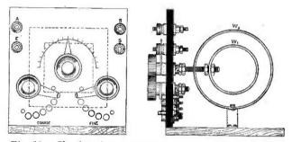
Fig. 11. Showing the construction of a tuner. The fixed coil  $W_2$  has two sets of tappings for rough and fine tuning respectively. The rotor  $W_1$  is connected in the secondary circuit.
