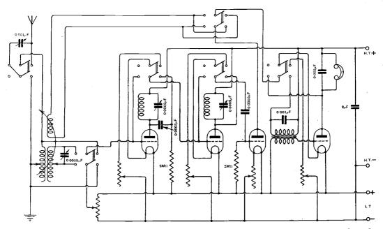
Fig. 1. "H.M." (Manchester). A four-value receiver (two H.F., det., one L.F.,) using tuned anode, and with switch for reversing reaction.
