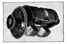
The Duanode variable condenser by the Fallon Condenser Co.
