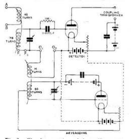
Fig. 2. Circuit connections of the oscillator and detector units.
