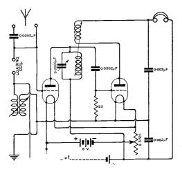
Fig. 3. Circuit diagram of the set.
