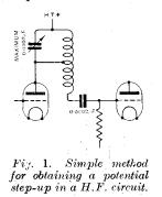
When making use of the tuned anode arrangement a much higher degree of amplification can be obtained if an additional inductance is connected in the lead to the grid condenser, and is coupled to the tuned anode coil. In the case of a single layer anode coil it is only necessary to wind on between 50 and 100 per cent. more turns, or when using duolateral coils of the plug-in type, to mount an additional coil near the tuned anode inductance (Fig. I).
