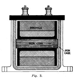
is to fit the open cored transformer into an iron box so that the magnetic circuit is closed through the case, as indicated in Fig. 3, which is a section through a transformer of this type.<sup>†</sup> The transformer winding is held in position in the box by a filling of wax compound.
