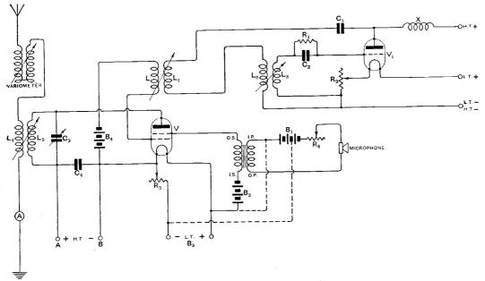
Fig. 5. Circuit of the complete transmitter.
