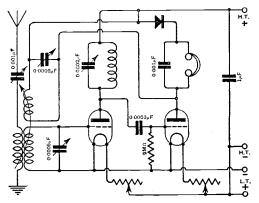
Fig. 2. "A.T." (Co. Cork). A receiver with two stages of H.F., tuned anode coupling, and crystal rectifier.
