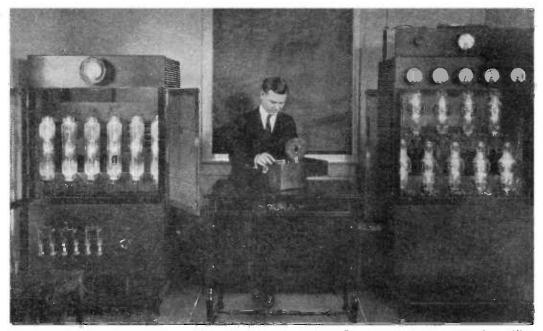
A corner of the transmitting room of station WJZ. The power panel, is shown at the left. The six rectifier values supply the 2,200 volts of direct current for the modulator and oscillator values of the transmitter panel to the right. Five 250-watt modulator, and 4 oscillator values of same rating are used in the transmitting circuit. The operator is shown checking the wavelength, which is 360 metres.
