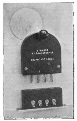
Fig. 24. A plug-in transformer with mounting. The inductance of the coils, and therefore their natural frequency, is varied by changing the position of the metal plate. (The Sterling Telephone Co.
