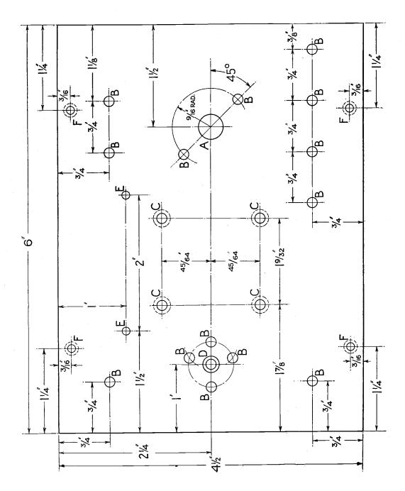
The location of the holes on the ebonite panels, and for the purpose it will be sufficiently accurate if the centres are pricked through on the panel. Size of holes: A, 3/8 in., B, 5/32 in., C, 5/32 in. and countersunk on top side. D, 5/32 and countersunk on underside; E,  $\frac{1}{8}$  in. blind holes 3/16 in. deep; F,  $\frac{1}{8}$  in. and countersunk on the top side for No. 4 wood screws.
