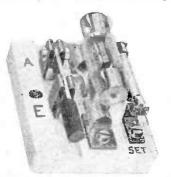
Aerial protection device of Messre. Siemens.
