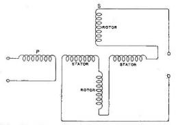
Fig. 29. Connections of another sort of variotransformer.
