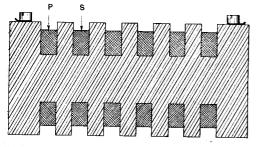
Fig. 25. A common form of long range high-frequency transformer.
