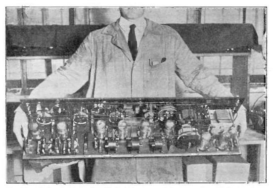
The photograph shows the interior of a well-built eight-valve super-heterodyne receiver. The first valve is the detector, the next the oscillator, then follow three H.F. stages, detector, and two note magnifiers.
