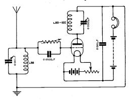
be made for critically adjusting it. Using this arrangement 35 miles north of London, it is possible to receive all the British broadcasting stations with good strength, far better, in fact, than can be hoped for with the single reacting valve arrangement.
