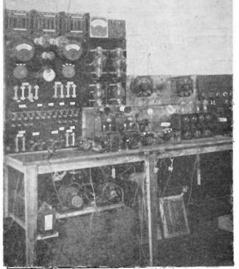
The experimental transmitting startsm (2 DY) of Mr. F. H. Haynes at Regent Square, Londom, W.C.1. The two small generator: supply A.C. at 700 cycles for stepping up to H.T., and also for the filament heating or the recilipring, oscillating and modulating values.
