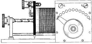
Fig. 7. An excellent short wavelength loose coupler.
