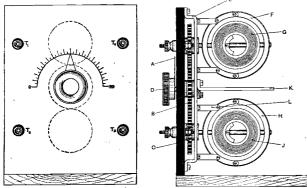
Fig. 19. Two variometers, operated through gearing by a single knob.
