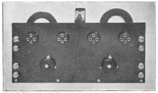
Fig. 3. The H.F. amplifier panel. The terminals are for input from the coupling unit, output to telephones, and H.T. and L.T. batteries. The inductances are arranged so that they present a minimum of coupling to each other.
