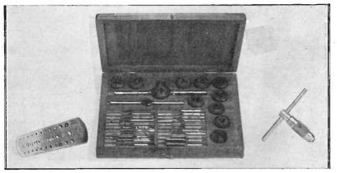
Fig. 2. BA. Tapping gauge, set of BA. stocks and dies, and tee tap-holder.
