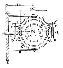
Fig. 4. End view of tuning and reaction coils.
