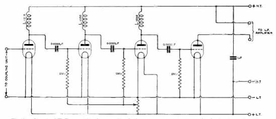
Fig. 2. Circuit of H.F. amplifier for use after the frequency change is effected by the detector and oscillator.
