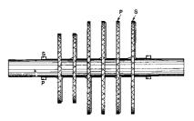
Fig. 22. When a number of basket coils are employed in a transformer, they should be spaced to reduce self-capacity.
