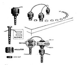
Plug connectors by Messrs. Autoveyors, Ltd.
