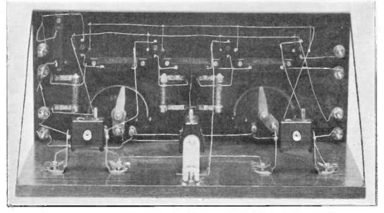
Fig. 1. Four value long wave amplifier with three high frequency circuits and detector.
