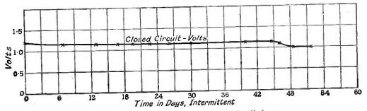
Fig. 1. Curve showing average voltage during discharge.
