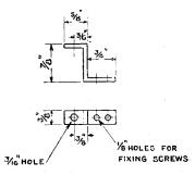
Fig. 5. Bracket for tuning coil.
