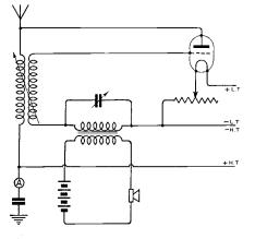
Fig. 1. A grid control valve transmitter.
