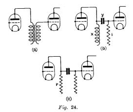
a low impedance condenser "y," which permits the grid to remain at an approximately zero potential. The leak "l" is inserted merely to maintain the grid mean potential constant, and in most cases is unnecessary, as sufficient leak is present in the valve and its connections.
