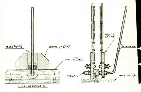
Scale drawing of simple yet effective coil holder.
