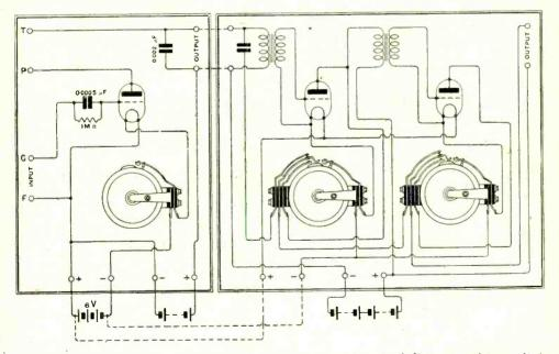
A particularly convenient arrangement for cutting in and out cf circuit low frequency amplifiers is the provision of spring contacts operated by a projection on the revolving resistance winding. With the rotary arm type of filament resistance it is not difficult to attach contacts to the panel which engage on the arm when the resistance knob is in the "off" position.
