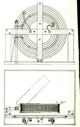
Fig. 4. Suitable for a larger power transmitter as described. The helix consists of 10 turns spaced  $\frac{1}{2}$  apart, outside diameter about 9". Connection for aerial and anode tap is made with clips. The grid coupling coil is the small cylindrical coil, 5" in diameter wound with 20 to 30 turns of No. 22 D.C.C. suitably mounted.
