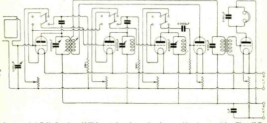
I ig. 1. "A.A.B." (London, N.W.8). A five-value receiver for use with a frame aerial. Three H.F., detector, and one L.F. values are employed, with switches for varying the number of values in circuit.
