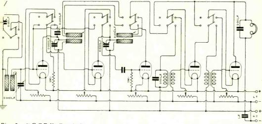
Fig. 5. "G.C.B." (London). Receiver with two H.F., rectifier and two note magnifiers, switches being connected to each valve. The reaction coil may be coupled with either the first or second anode circuits.
