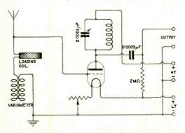
Fig. 2. "D.G." (London, W.1). Here we give a diagram indicating how a H.F. amplifying valve may be added to a receiver.
