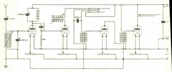
Fig. 3. "YANK" (Doncaster). Receiver with H.F., rectifier and optional note magnifiers (1-V-2). The telephones are connected to a plug. The purpose of the variometer in the anode circuit of the rectifier is to provide reaction effects.
