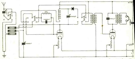
Fig. 6, "J.E." (Arbroath). Experimental receiver employing two values and a crystal rectifier. Switches are provided so that value or crystal rectification may be used. When the latter method is employed, both values may operate as low frequency amplifiers.
