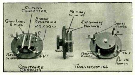
Constructional details of the plug-in units for intervalve coupling in the high frequency circuits.
