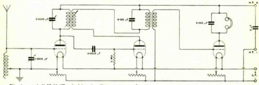
Fig. 1. "A.C.H." (Tonbridge.) Three valve receiver with one H.F., detector, and one L.F. valves. Tuned anode H.F. coupling is employed, with reaction to the anode coil.
