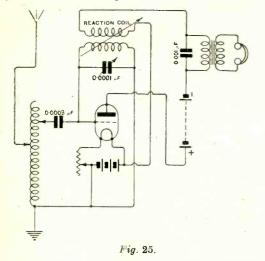
which can be tuned with the o-ooor microfarad condenser, and on the accuracy with which this circuit is tuned will depend the success of the experiment. The connections from the valve to the grid circuit coil and reaction coil should be kept as short as possible and well away from the other parts of the apparatus, especially the tuner.
