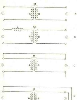
Fig. 107. To obtain the mutual inductance, measure the inductance with the coils in series as at (C), and then with the connections as at D. If the inductances are  $L_1$  and  $L_2$ ,  $M = \frac{L_1 - L_2}{4}$ .
