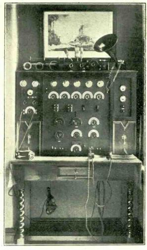
vernier condensers. At the bottom of the panel are potentiometer, reaction condenser and switch for providing reaction either on the aerial or the H.T. transformer. The programmes from all the British Broadcasting Co.'s stations can be heard at will. Paris and the Hague are received regularly.
