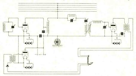
Fig. 3. Connections of transmitting and receiving equipment installed on the train.
