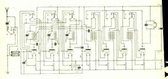
Fig. 2. " S.B." (Norway). Diagram of receiver with three stages of H.F., rectifier, and three note magnifiers.
