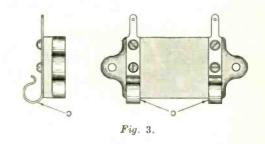
inside the moulded case under appropriate compression by means of a metal clamp, it is possible to ensure a greater constancy of capacity value than is otherwise possible.
