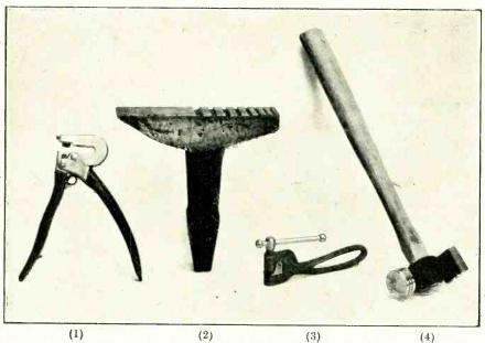
Fig. 2. Tools used in sheet metal working. (1) Punch. (2) Bick iron. (3) Screw punch. (4) Square-faced hammer.
