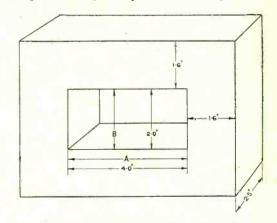
Fig. 91. Dimensions of the core which is built up of 10 to 14 mil. laminations of transformer steel.
