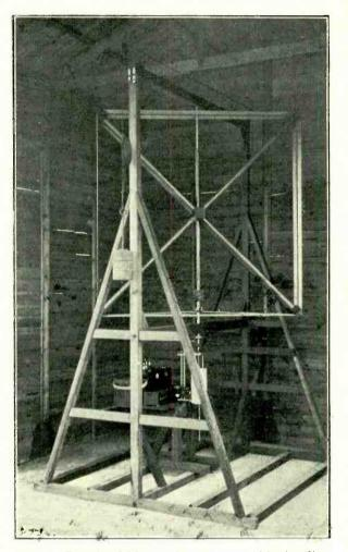
Fig. 5. Directional frame and apparatus used in recording atmospherics.
