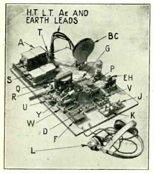
Fig. 8. Complete dual and crystal receiver.
