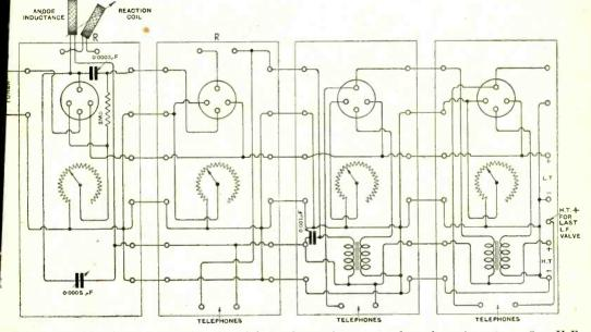
Fig. 5. "G.C." (Burton-on-Trent). A four-value receiver arranged on the unit system. One H.F., detector and two L.F. values are used. The tuned anode method of H.F. coupling is employed.
