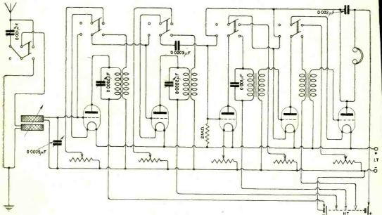
Fig. 2 " E.C.G." (Luton). Receiver with 2-v-2. detector, and two L.F. valves. A series-parallel switch is required for the aerial condenser, and switches for controlling the number of valves in use.
