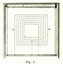
The complete roller can be turned into different directions in order to utilise the directive action of the frame aerial.
