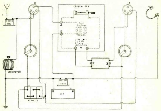
The principle of the circuit employed can be followed from this diagram. The aerial tuning induct i the crystal receiver is used as the tuned anode coil. If it is not desired to go to the trouble of incorporating the components into a complete instrument they may be set out as shown and secured to a base board.
