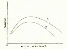
Fig. 111. The secondary current varies with the mutal inductance in the manner shown. There is one best value of coupling which gives the maximum secondary current. If the secondary resistance is increased, the relationship between secondary current and the coupling is as shown by curve B. secondary current as shown by curve B. the voltage applied to the primary is E, t primary and secondary resistances  $R_1$  and  $R_2$ .
