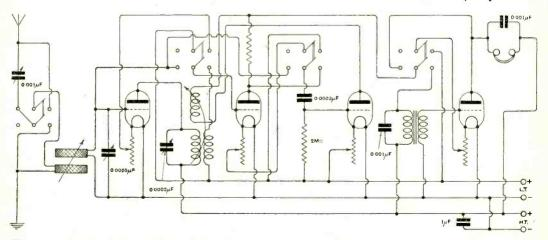
Fig. 4. "E.A.A." (West Ham). Diagram of a four-valve receiver employing two H.F., detector and one L.F. valves. The reaction coil is coupled to the H.F. transformer, and switches are provided for cutting out any valve except the detector.
