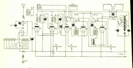
Diagram of the connections showing the arrangement of the switches.
