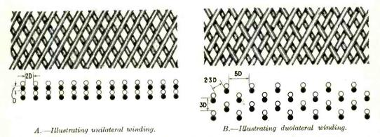
Fig. 1. Diagrams illustrating the difference between duolateral and unilaterial windings.
