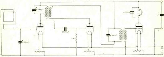
Fig. 2. "A.G.B." (Camberley) Receiver with H.F., rectifier and note magnifier (1-V-1), connected to a frame aerial.
