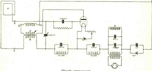
Circuit arrangement. A. Frame aeriai 3' 6" sq. 9 turns No. 20 C.C., <sup>3</sup>/<sup>"</sup> apart. B. For broadcast reception may be an Igranic coil No. 75. C. Reaction coil for broadcast reception may be Igranic, No. 100.
