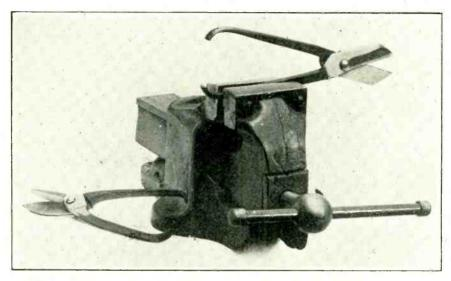
Fig. 1. Tinman's snips mounted in the vice for accurately cutting sheet metal.
