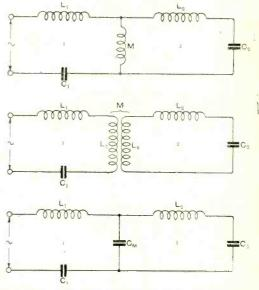
Fig. 106. The upper diagram (A) shows direct coupling; the centre diagram (B) shows magnetic coupling; and the lower diagram (C) capacitive coupling.
