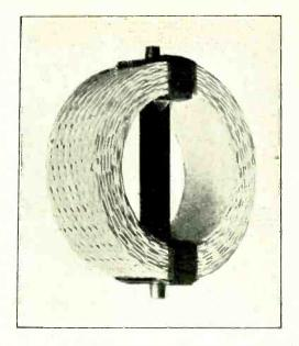
Fig. 6. A coil with the special gimbal method of mounting.
