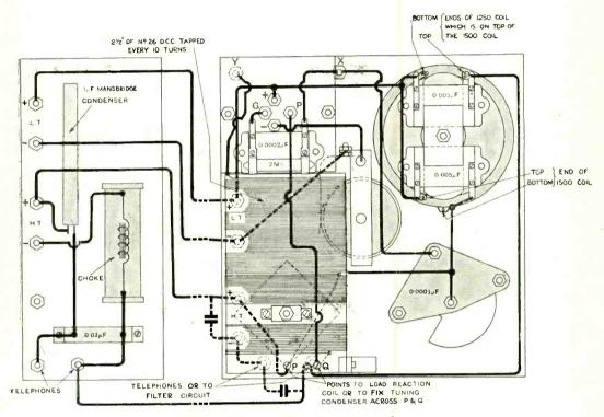
Wiring diagram of filter and tuner panels.
