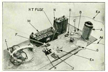
Fig. 1. The layout of the components of a dual amplification receiver with crystal detector. Wired up as shown, it is possible to demonstrate the action of the circuit, after which it is quite simple to design a boxed-up outfit if desired, to suit the requirements of the reader.
