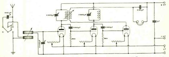
Fig. 1. "RL.S." (Geneva). A three-valve receiver is shown, employing two H.F. amplifying valves and detector. Tuned anode H.F. coupling is used, with reaction to the anode coil of the first valve.
