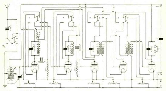
Fig. 4. "C.V." (Devon). Diagram of a receiver with two stages of tuned anode H.F. amplification, rectifier and two note magnifiers (2-V-2). The reaction coil is coupled with the first anode coil.
