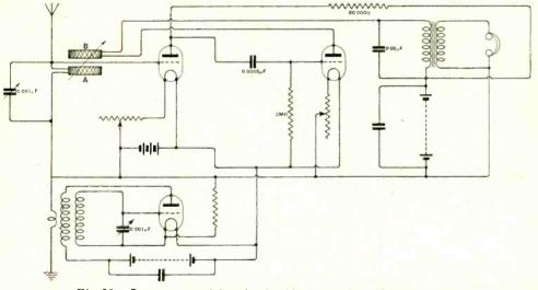
Fig. 26. Long-wave receiving circuit with separate heterodyne wavemeter.
