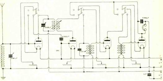
Fig. 1. "C.H.S." (Derby). Diagram of 4-value receiver with one H.F., tuned anode coupled, rectifier and two note magnifiers (1-V-2). Switches are provided so that any value except the rectifier may be cut out of circuit.
