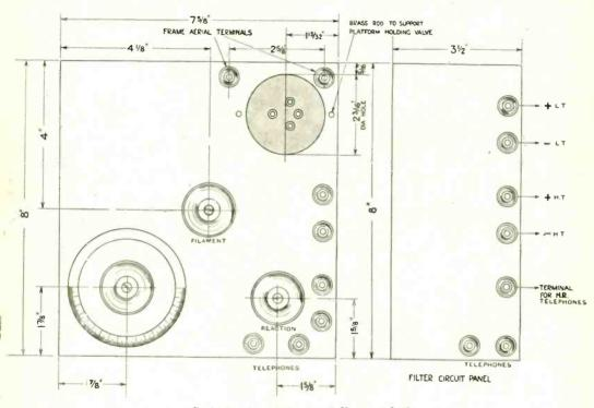
Scale drawing of tuner and filter punels.
