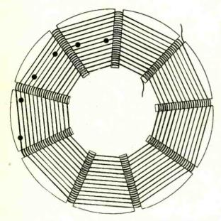
Fig. 3. Basket coil with taps. No. 18 D.C.C. wire wound upon ebonite or other insulating material. Sometimes a wooden former with wooden pegs is used. Suitable for small power transmitters.
