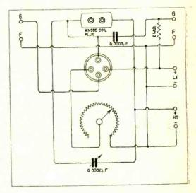
Fig. 1. " J.G.D." (Lewisham). Tuner and single valve H.F. panel.
