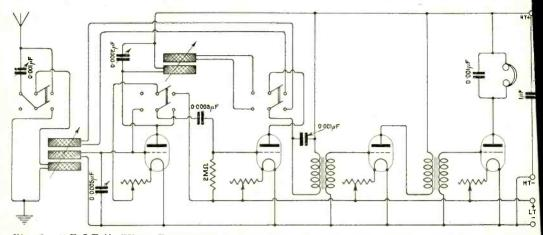
Fig. 3. "F.J.F." (West Bromwich). Connections of a four-value receiver employing one H.F., detector and two L.F. values. Switches are provided for disconnecting the H.F. value, and for employing reaction on either the closed circuit or anode coils.
