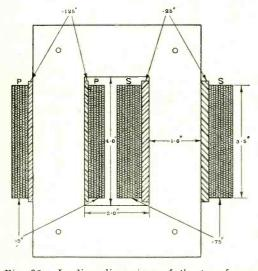
Fig. 92. Leading dimensions of the transformer. The primary winding has 275 turns of No. 17 D.C.C., and a sheet of paper is placed between each layer. The secondary winding has 2,500 turns of No. 27 D.C.C., with each layer separated with a sheet of thin paper or oiled silk. The coils should be tapped with empire cloth.
