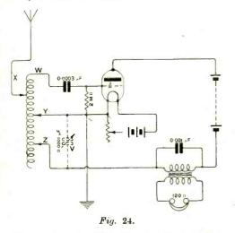
The valve in Experiment 12 has been employed for the purpose of amplifying high frequency oscillations, these amplified oscillations occurring in the plate circuit. The energy of the amplified oscillations
