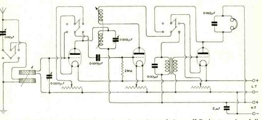
Fig. 3. "E.J." (Brondesbury N.W.6.). A three-valve receiver employing one H.F., detector, and one L.F. valves. The H.F. and L.F. valves may be switched out of circuit by means of double pole change-over switches.
