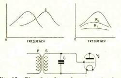
Fig. 97. The effect of transformer capacity is to give it a resonant frequency which may be shown by plotting frequency and amplitude of signal. The curve is moved to the left from say position 2 to position 1 by adding a capacity C across the windings. The effect of adding a resistance across the windings is shown. A high resistance produces a reduction in amplitude and a broader peak as at  $R_2$ . A lower resistance produces a flatter curve altogether, represented by  $R_1$ .
