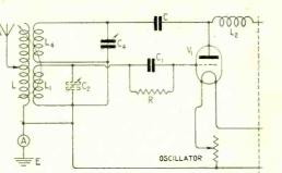
Fig. 2. Coupled or Meissner circuit. Values as in Fig. 1, also  $L_4 = 25$  to 30 turns of No. 22 D.C.C. on former 5" diameter,  $C_4 = variable$  condenser 0.0002  $\mu F$ .
