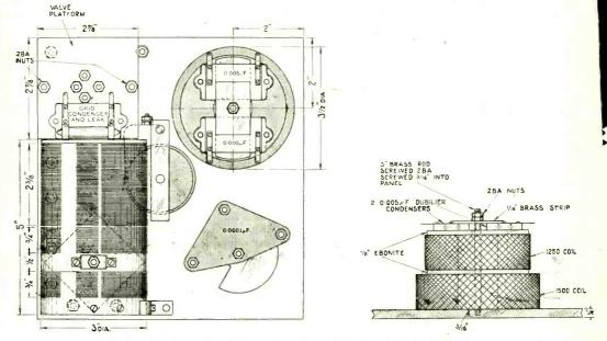
Underside of panel and the method of mounting the oscillator inductances.
