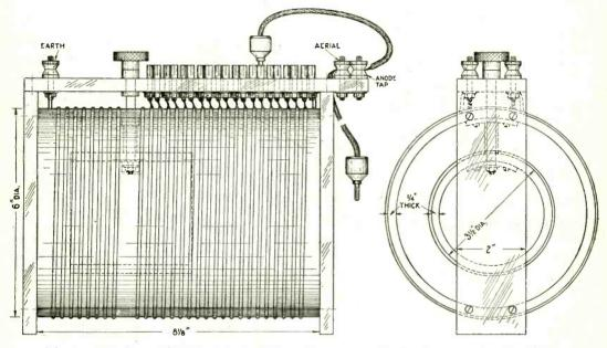
Fig. 5. Here the aerial coil is wound with bare No. 14 wire with the turns spaced. Tappings are taken to sockets, and connections for the aerial and anode tap are made with plugs. The grid coil rotates inside the large coil. The dimensions are given.
