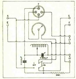
Fig. 2. "J.G.D." (Lewisham). A H.F. amplifying unit is shown, with switch for cutting out the valve when desired.
