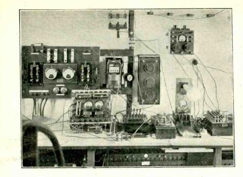
Fig. 13. Apparatus for examination of wave form of atmospherics.
