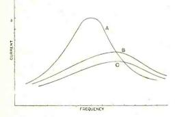
Fig. 109. Curve A represents the resonance curve for circuit (1) above. When circuit (2) is coupled, the resonance curve is as shown by curve B. If the resistance of circuit (2) is increased, or if the coupling is increased, the curve will be as represented by C.
