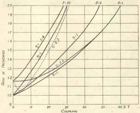
FIG. 9.-FREQUENCY RATIO AND COUPLING.
