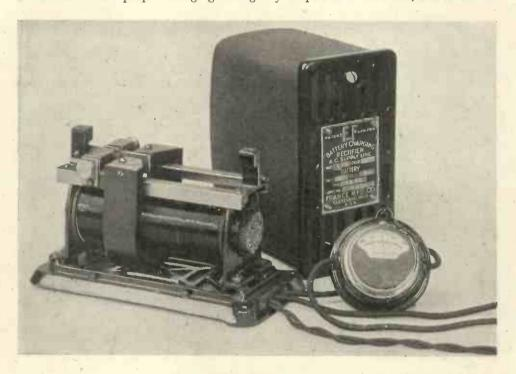
current is rectified by means of the vibrating tongue, which, actuated by magnets in circuit with the alternating supply, automatically connects the line first to one pair of contacts, then the other in exact synchronism with the supply current. The device has thus no rotary parts, and being simple of construction, can be marketed at low cost.
