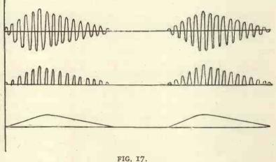
process. Fig. 17 illustrates this, and, like Fig. 16, also shows theoretically the rectified oscillations and the effect of the low frequency pulses on the telephone diaphragm.
