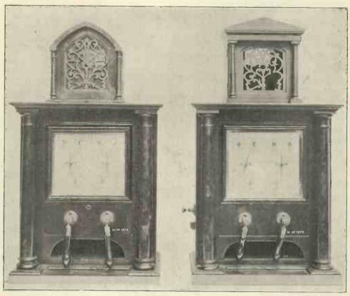
MESSRS. COOKE AND WHEATSTONE'S DOUBLE-NEEDLE TELEGRAPH INSTRUMENTS, A.D. 1837.
