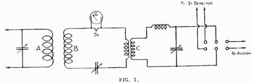
adjustments. The following method, while not giving the greatest sensibility, seems to give the most easily reproducible readings. The antenna and closed circuit are first tuned for best signal at very losse coupling adjusting the bridging condenser, grid condenser and reinforcing coupling, if one is used. Then the main coupling is gradually closed to the best point, and the secondary returned slightly for the note desired, leaving the antenna unchanged.\*
