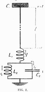
by considering the whole arrangement (antenna and flywheel coupling) as a pair of coupled quasistationary circuits, that is of circuits whose dimensions are small in comparison with the natural wavelengths of the system. With this assumption the system can be treated as two coupled circuits in each of which the capacity, as well as the inductance, are wholly separated.
