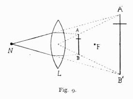
from a study of Fig. 9. Let L represent a double convex lens, with an object, AB, placed between it and the point F, which is the principal focus of the lens. The rays from the object, AB, are refracted on passing through the lens, and again refracted on leaving the lens, so that an image of the object is formed at the eye, N. As it is impossible for the eye to follow the bent rays from the object, a virtual image
