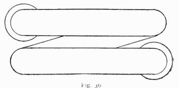
form of a spiral. The whole is then covered with braid. Hence all the conductors lie on the surface of a **tube** of **large** diameter, and the current distribution is more uniform than if they were made into a solid cable.
