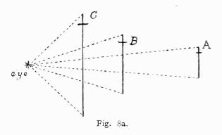
to the eye than the angle presented by the object when moved to B, and the image therefore appears smaller. When the object is moved to either B or C, it is viewed under a much greater angle, causing the image to appear much larger. If we take a watch or other small circular object and place it at A, which we will suppose is
