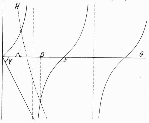
that lies between the two branches of the curve  $y = \tan \theta$ , and the nearer the hyperbola passes through the point  $\theta = \frac{n}{2}$  on the axis of  $\theta$ . The conditions, therefore, that two natural wave-lengths of the antenna with flywheel coupling are near together are:  $\sqrt{\frac{LC}{LC}}$  near to  $\frac{n}{LC}$
