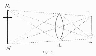
In this, LL, Fig. 8, whose local length suits the length of the box, the image produced will be brighter and more distinct than that formed by the aperture, H, since the rays which proceed from any point of the object will be brought by the lens to a focus on the glass screen, forming a bright, distinct image of the point from which they come. The image
