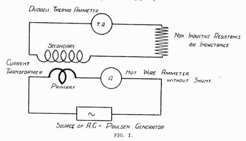
ARRANGEMENT OF APPARATUS FOR DETERMINING THE ERROR IN THE TRANSFORMATION RATIO OF A CURRENT TRANSFORMER DUE TO RESISTANCE OR INDUCTANCE IN THE SECONDARY CIRCUIT.
