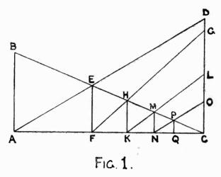
Further, in dealing with three or more quantities, Mr. Lowey's method may be considerably simplified by setting them all off, after the first, along the same line, *CD*, as shown in Fig. 1, which applies to five quantities. The construction is as follows:—
