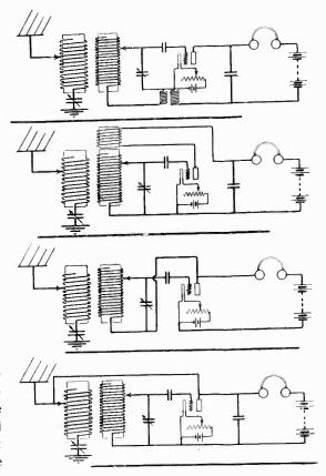
instead of to the filament as in the usual circuits. In the fourth diagram the aerial is joined to the plate. It is said that some operators have difficulties in making the valve oscillate with the current, but when the knack is discovered it is easy enough. The author states that with any of these circuits signals from Europe can be heard as far west as St. Louis under favourable conditions with comparatively small aerials.
