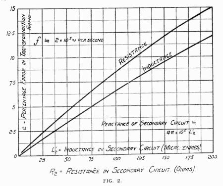
CURVES SHOWING THE RELATION BETWEEN THE PERCENTAGE ERROR IN THE TRANSFORMATION RATIO AND (I) THE RESISTANCE IN THE SECONDARY CIRCUIT, (2) THE INDUCTANCE IN THE SECONDARY CIRCUIT, AT A GIVEN FREQUENCY.
