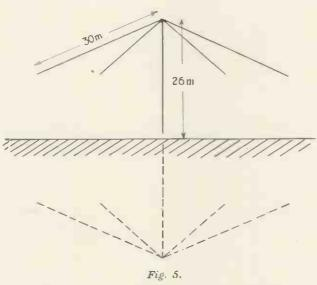
the six ribs would be  $6 \times 1.55 = 9.3$ , since m would then be 52/30. Since the average potential of the actual vertical wire due to the six ribs is 13.5, that of the other half of the 52 metres, remote from the ribs, must be  $2 \times 9.3 - 13.5 = 5.1$ . Hence this
