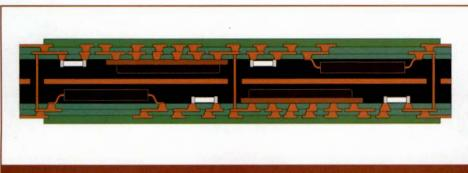
**Figure 2**: The Occam Process uses unthinned, packaged chips, and a variety of core and build-up materials. Both methods can bury active and passive components. Each chip shown here is several times thicker than the chip shown in Figure 1
