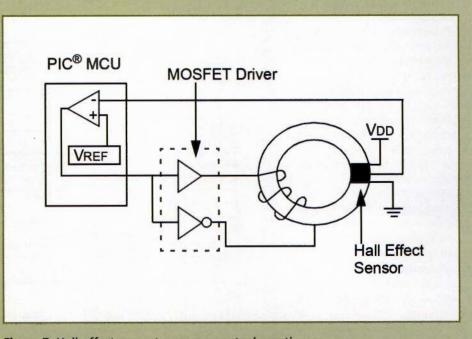
Figure 7: Hall-effect current measurement schematic
