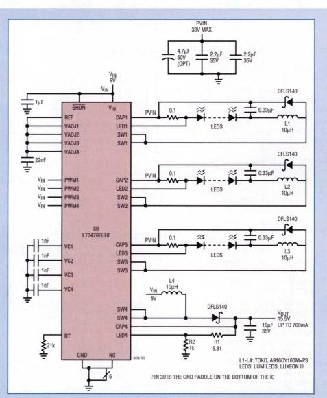
**Figure 9:** Here is a simple way to save BOM cost and reduce solution size in an LCD. A single-quad LED driver IC provides power for the LED backlight and the LCD bias of an LCD projector. Three of the channels drive R, G and B LED strings, while the fourth provides a voltage source in boost mode
