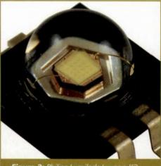
Figure 2: Philips Lumileds Luxeon K2 with TFFC
