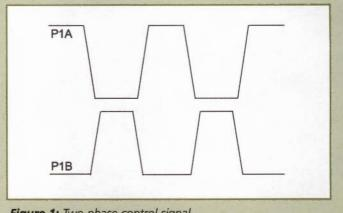
Figure 1: Two-phase control signal
