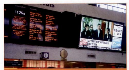
This picture, taken at Euston station, shows that a well-designed LED video wall can overcome the problem of reflections off the front surface. Sadly, the lower cost LED displays mounted adjacent to the video wall are mounted inside protective boxes and, again, ambient light reflecting off the surface of these displays reduces the legibility of the text
