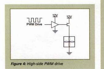
For 3-wire fans, the tachometer output will not be accurate if PWM is used. The sensor providing the tachometer output on 3-wire fans is powered from the same supply as the fan coils, thus using a PWM to control fan speed will render the fan's tachometer inaccurate.
