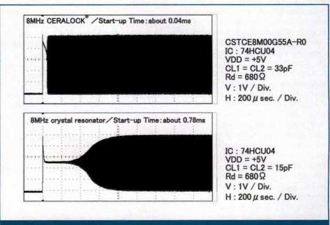
Figure 1: Comparison of start-up time characteristics
