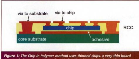
core, and electrolessly plates the chip bond pads at the wafer level
