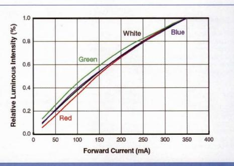
Figure 1: Relative luminous intensity vs forward current
