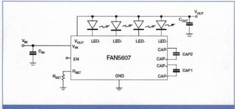
Figure 5: The FAN5607 uses two capacitors and has three modes, 1X, 1.5X and 2X
