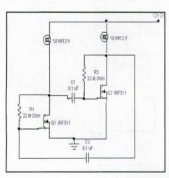
The given circuit (left) is for an 'Incandescent Lamp Flasher' using two IRF511 MOSFETs which are configured as a simple astable multivibrator to alternately switch the two lamps on and off.
