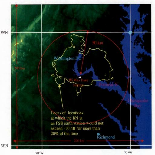
A grid of points was set up at 2.5km intervals over an area of 200 x 200km with the WiMAX base station at the centre. The value of path loss was computed between the base station and each point. The resulting locus is shown in this graph. For fixed satellite service earth stations sited outside the contour the long-term protection criterion would be met, but it would not be met for earth stations inside the contour
