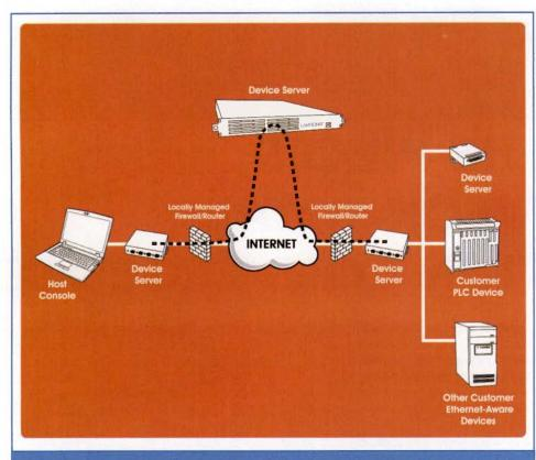
Figure 2: Users must be able to easily establish two-way communication that works without weakening the firewalls
